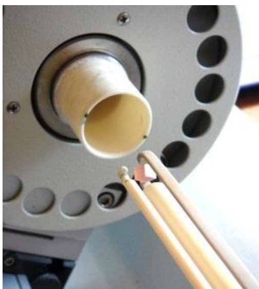
Figure 5.1. High-temperature Resonant Ultrasound Spectroscopy system at the University of Cambridge [2].
