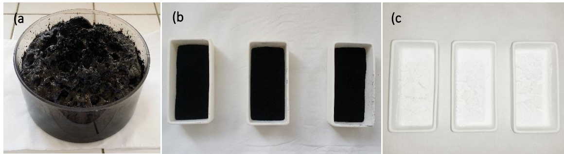
Figure 2.4. (a) Black porous sponge-puffy stuff; (b) Black milled precursor; (c) Whitish powder after calcination.
