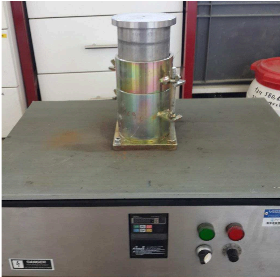
Figure A5-4: the test mold on the vibration table
