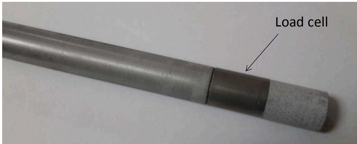
Figure 2-3 : Detail of the rough instrumented model pile (pile 1 diameter=18mm)
