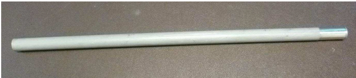
Figure 2-3 : Detail of the rough instrumented model pile (pile 1 diameter=18mm)
