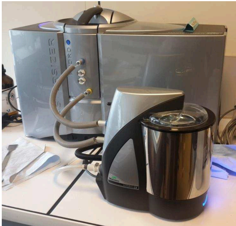
Figure A6-1: Size distribution by laser machine of IFSTTAR
