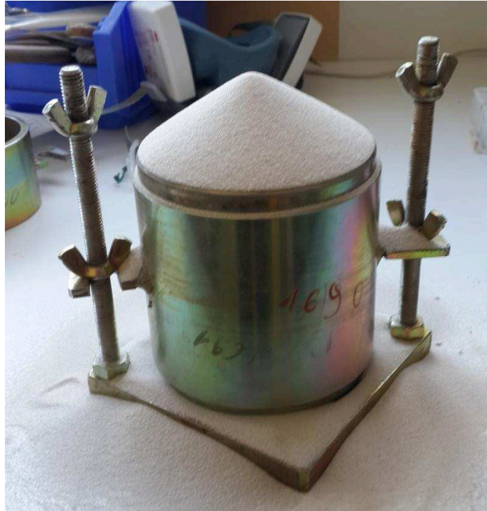
Figure A5-2: the test mold with the conical sand at the end of the filling step
