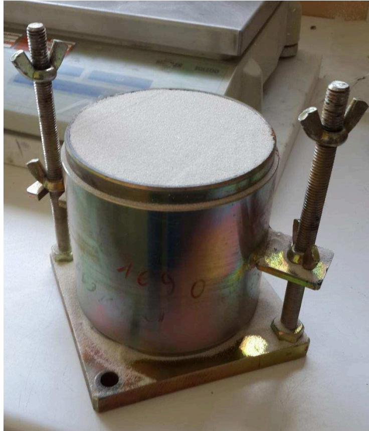
Figure A5-3: the test mold after shaving the extra sand
