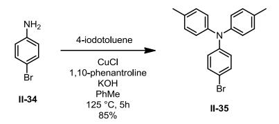
Figure 2.27 - Copper-catalyzed synthesis of functionalized triarylamine II-35.
