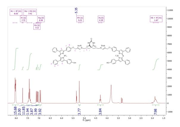
Figure 3.33 -  $^{1}$ H NMR of barbiturate-containing BF<sub>2</sub>-chelate azadipyrromethene thread III-52 (300 MHz in dichloromethane- $d_2 + 0.5\%$  of methanol- $d_4$ ).
