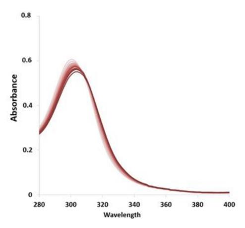
Figure 2.15 - Titration of II-28 in the presence of barbital II-4 monitored by electronic absorption spectroscopy in dichloromethane ([II-28] =  $25 \mu M$ ).
