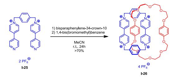
**Figure 1.18** -  $\pi$ - $\pi$  Stacking-based synthesis of [2]catenane **I-26**.
