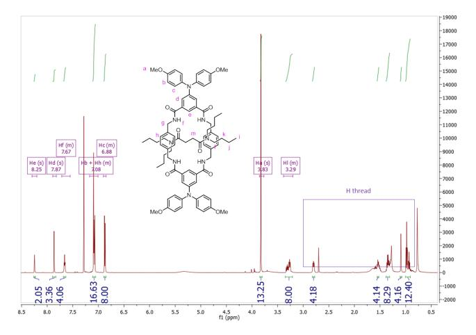
Figure 4.15 - <sup>1</sup>H-NMR of triarylamine-containing clipped [2]rotaxane IV-22 (600 MHz in CDCl<sub>3</sub>).
