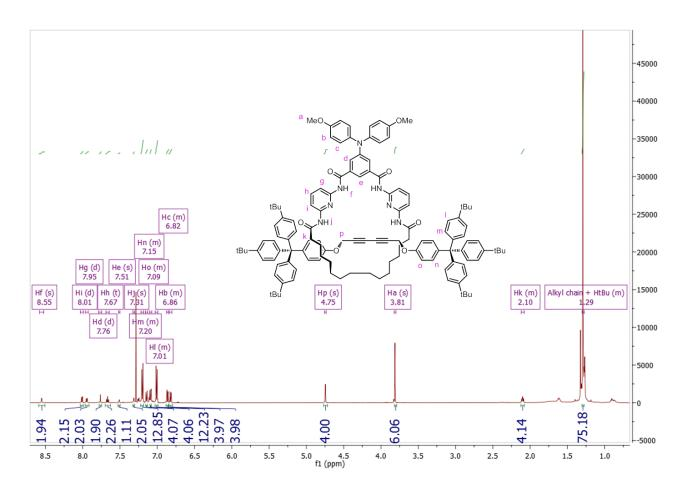
Figure 4.10 - <sup>1</sup>H-NMR of triarylamine-containing Glaser [2]rotaxane IV-21 (600 MHz in CDCl<sub>3</sub>).
