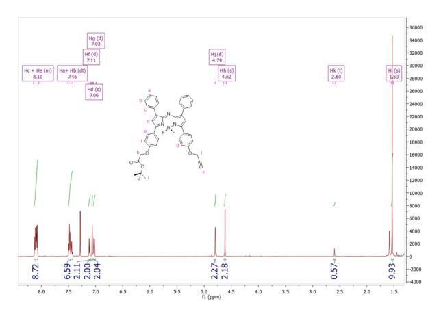
**Figure 3.16** - <sup>1</sup>H NMR of *tert*-butyl-carboxypropargyloxy BF<sub>2</sub> - azadipyrromethene **III-30** (600 MHz in CDCl<sub>3</sub>).
