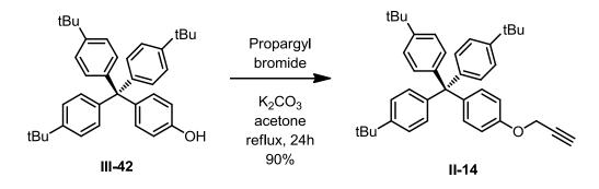
Figure 3.25 - Synthetic scheme of alkyne trityl stopper II-14.
