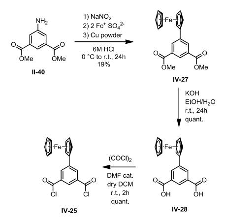
Figure 4.13 - Synthetic scheme of 5-ferrocenylisophthaloyl chloride IV-25.
