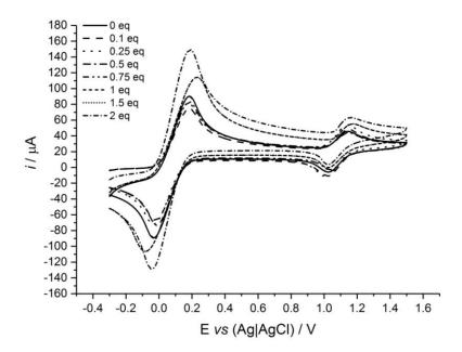
**Figure 2.18** - CVs recorded of DCMF and macrocycle **II-29** on addition of 0.1-2 molar equivalents of barbital **II-4**. Scan rate =  $500 \text{ mV s}^{-1}$ , in  $10^{-1} \text{ M TBAPF}_6$  in in dry degassed dichloromethane.
