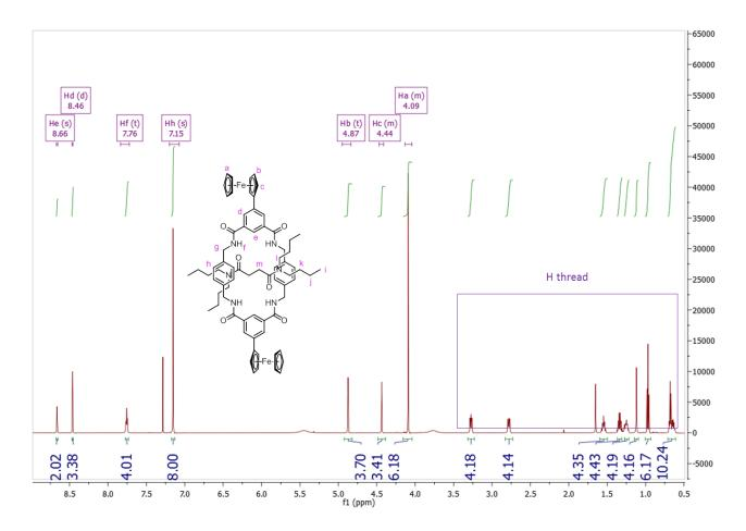
Figure 4.16 - <sup>1</sup>H-NMR of ferrocene-containing clipped [2]rotaxane IV-23 (600 MHz in CDCl<sub>3</sub>).
