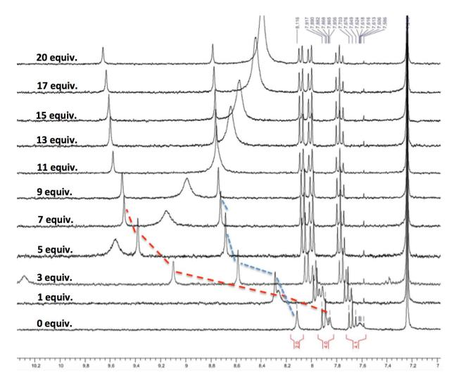
**Figure 2.16** - Titration of ferrocene-containing macrocycle **II-28** in the presence of barbital **II-4** monitored by <sup>1</sup>H NMR using the chemical shifts of the host amide protons (1 mM in *d*-chloroform).
