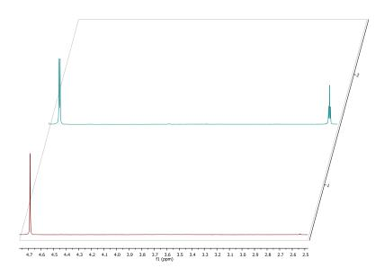
**Figure 3.27** - <sup>1</sup>H NMR of alkyne stopper **II-14** (top) compared to deuterated alkyne stopper **III-51** (bottom) (300 MHz in CDCl<sub>3</sub>).
