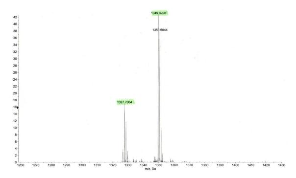
Figure 7.16 - Mass spectrum (ESI) of triarylamine-containing clipped [2]rotaxane IV-22.
