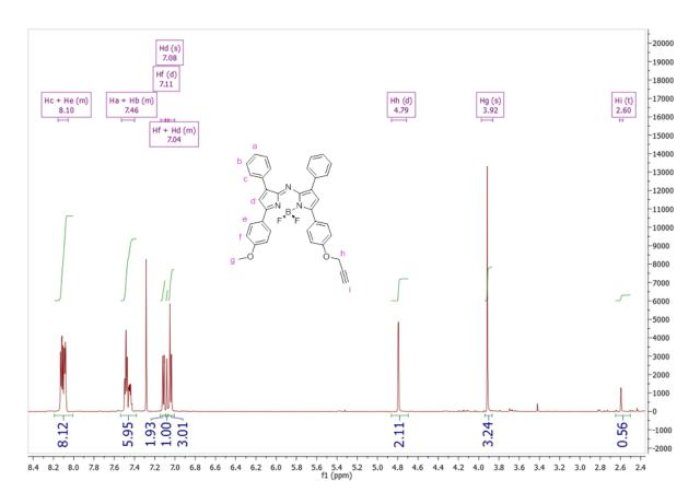
**Figure 3.14** - <sup>1</sup>H NMR of methoxypropargyloxy BF<sub>2</sub> - azadipyrromethene **III-29** (600 MHz in CDCl<sub>3</sub>).
