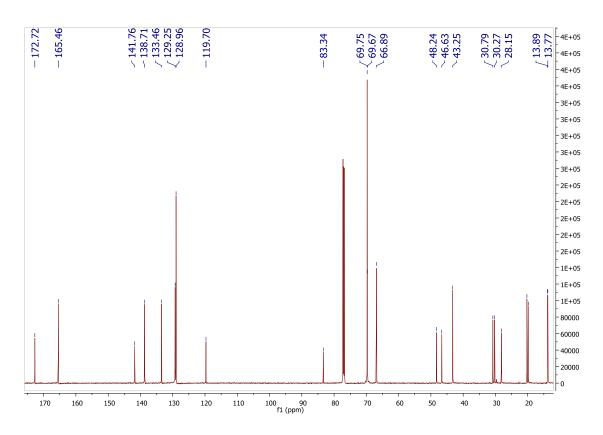
Figure 7.17 - <sup>13</sup>C-NMR of ferrocene-containing clipped [2]rotaxane IV-23 (600 MHz in CDCl<sub>3</sub>).
