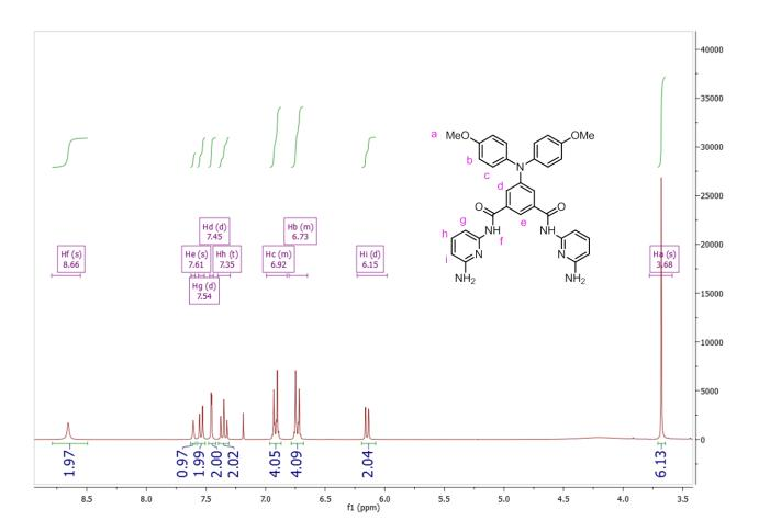
Figure 2.34 - <sup>1</sup>H-NMR of acyclic triarylamine Hamilton-type receptor II-49 (600 MHz in CDCl<sub>3</sub>).
