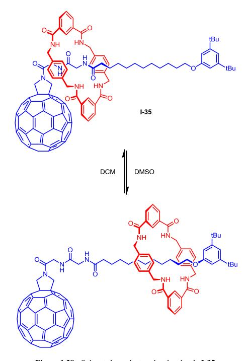
Figure 1.28 - Solvent-dependent molecular shuttle I-35.
