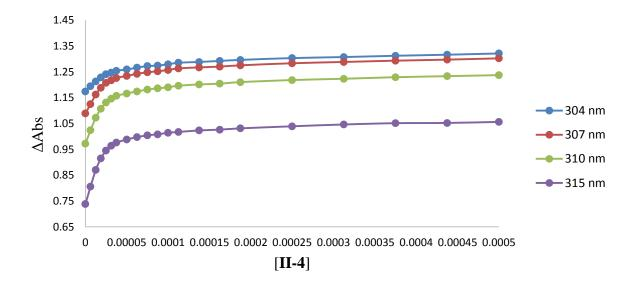
Figure 2.37 - Titration of II-50 in the presence of barbital II-4 monitored by electronic absorption spectroscopy in dichloromethane ([II-50] =  $25~\mu M$ ).
