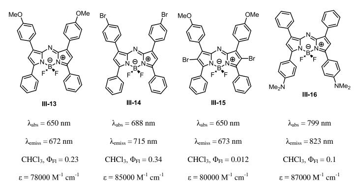
**Figure 3.6** - Molecular structures and optical properties of differently substituted BF<sub>2</sub>-chelates of tetraaryl-8-aza-dipyrromethenes.
