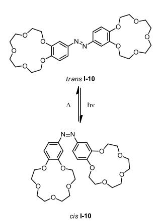
Figure 1.5 - Photoisomerization of crown ether-based molecular tweezer I-10.
