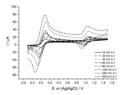
**Figure 2.17** - Cyclic voltammogram of 1:1 DCMF and macrocycle **II-29**, in a solution of 10<sup>-1</sup> M TBAPF<sub>6</sub> in dry degassed dichloromethane at different scan rates.
