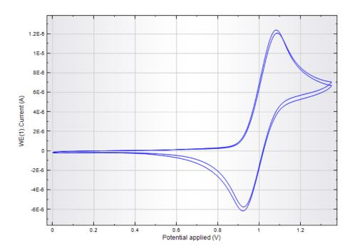
**Figure 2.39** - Cyclic voltammogram of **II-50**, in a solution of  $10^{-2}$  M TBAPF<sub>6</sub> in dry degassed tetrahydrofuran at scan rate =  $100 \text{ mVs}^{-1}$ .
