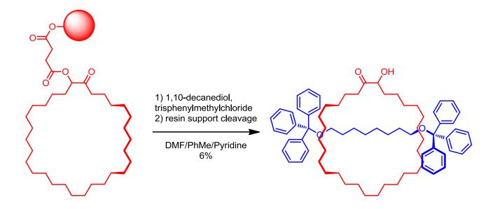
Figure 1.20 - Synthetic scheme of first [2]rotaxane I-28.
