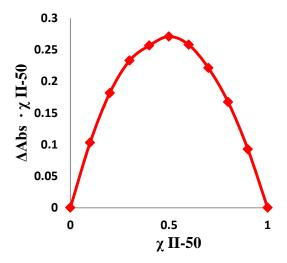
**Figure 2.38** - Job plot for the change of absorption of macrocycle **II-50** at 304 nm in dichloromethane in presence of barbital **II-4** ([**II-50**] =  $25 \mu M$ ).
