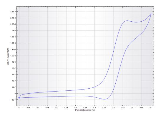
**Figure 4.17** - Cyclic voltammogram of **IV-23**, in a solution of  $10^{-2}$  M TBAPF<sub>6</sub> in dry degassed acetonitrile at scan rate =  $200 \text{ mVs}^{-1}$ .
