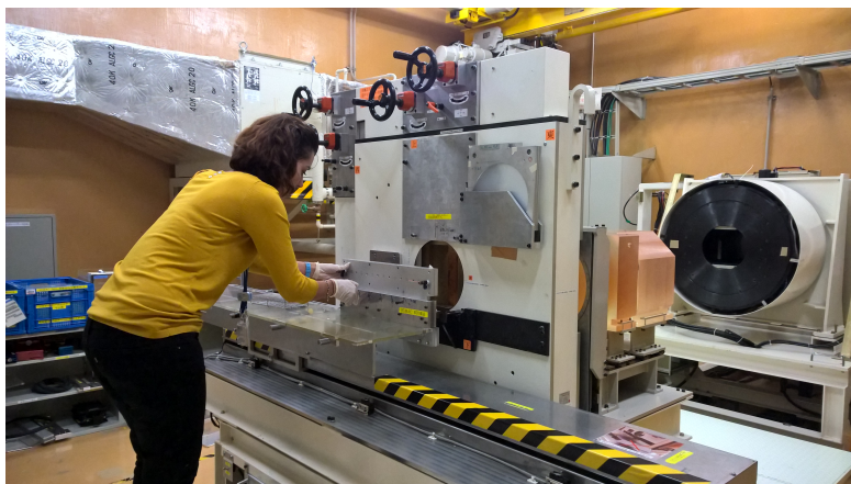
Figure III.5: The gas chamber is placed in front of the beam exit at the irradiation room of HIMAC.
