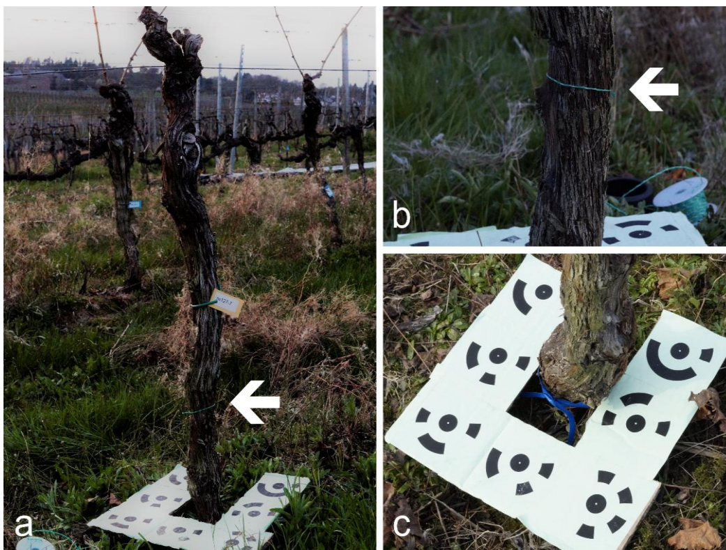
Figure 5.1. Example of the experimental setup for taking the pictures (a) with a general view of grapevine with the georeference grid and the point of measurement (white arrow); (b) focus on the point of measurement of trunk circumference and cross-sectional area 10 cm above the grafting point highlighted in the field using a plastic cord; (c) focus on the georeference grid around the base of the trunk.
