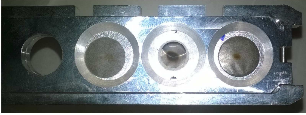
Figure 3.3: Target support and targets (photograph taken after the experiment), from left to right: hole, carbon backing, plutonium target and lead target. The Pu target was slightly detached from the support. Note the marks left by the beam on the targets.
