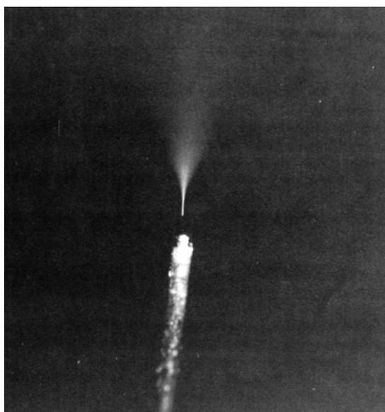
**Figure 16** - Photograph of a stable cloud, also known as Taylor cone, created by electrospray ionisation. From (Smith et al., 1988).
