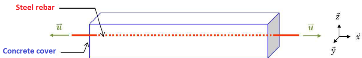
Figure 1.1 Principles of the tie-beam test (Torre-Casanova 2013).
