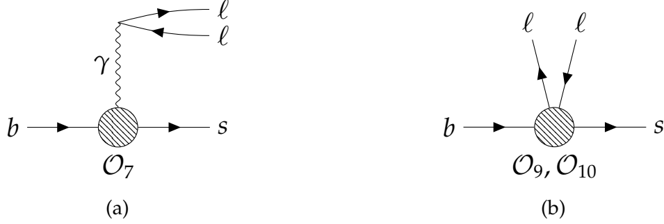
Figure 1.5: Diagrams for the radiative b \rightarrow s\gamma and semileptonic b \rightarrow s\ell^+\ell^- operators. Short-distance contributions are hidden in the vertex.
