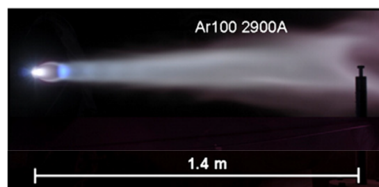
Figure 39: Photograph of PS-PVD plasma jets emitted from 03CP plasma torch. Chamber pressure and net power input were kept constant at 200 Pa and 60 kW [58]
