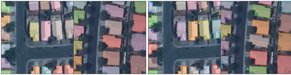
Figure 2.1: Vectorization vs. direct extraction of polygons. Left: a pixel-wise segmentation of aerial images, predicted by a neural network [LQQ + 18]. Vectorizing the contours of each building instance will result in numerous approximations. Right: polygons are directly extracted using an adapted architecture [LWL18]. Image taken from [LWL18].
