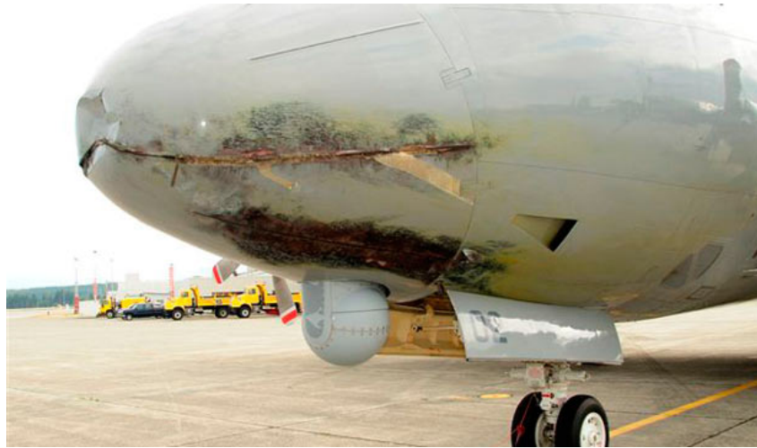
Figure 1.9: Effect of the swept stroke displacement of a lightning arc attachment on the radom of an RNZAF Orion. Taken from [27].
