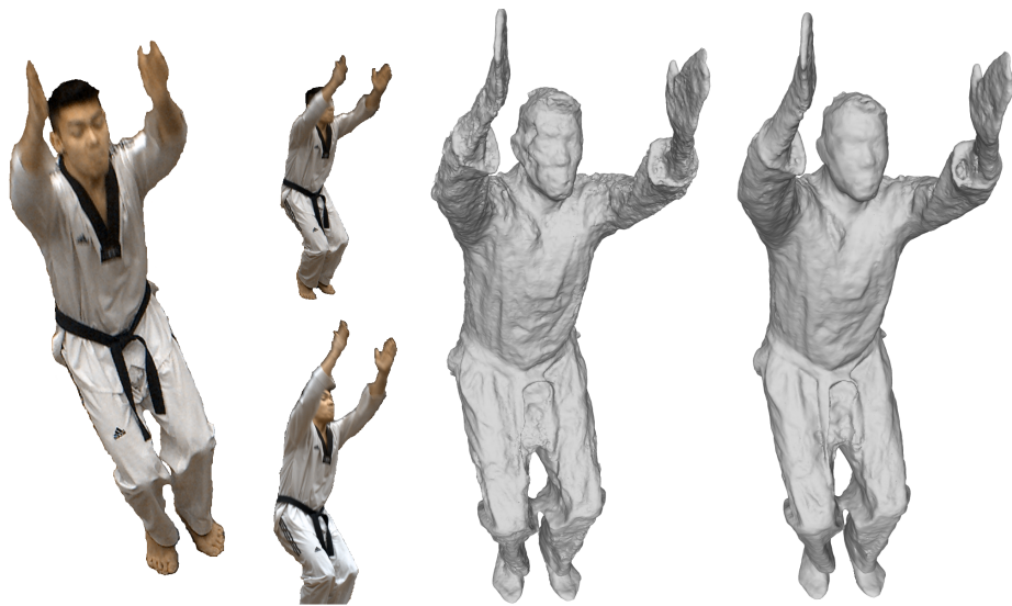
Figure 3.10: ( Left ) 3 input images, ( middle ) plane based classifier, ( right ) volumetric classifier. The face is highly occluded ( left ) yielding noisier and less accurate reconstructions when using a planar receptive field, whereas the volume counterpart yields smoother and more accurate details.
