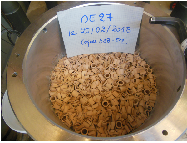
Figure 6.5 : The oedometer test finished at \sigma_a = 0.42 MPa ( Figure 6.4 ): a – A view of the top surface after the test (in contact with the loading plate), and b – The fragments divided into the sieve sizes ( Figure 6.6 ).
