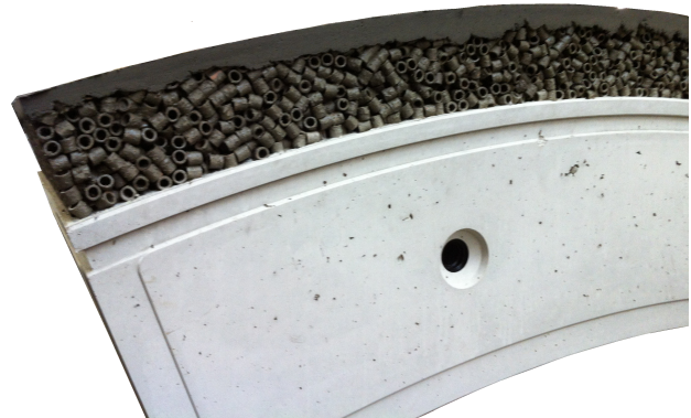
Figure 1.2 : Compressible arch-segment (VMC) is an element of tunnel lining constructed as an union of classic concrete segment and coated granular layer – according to joined US Patent (pending) of Andra and CMC.
