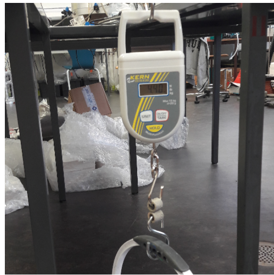
Figure 4.4 : Experimental determination of tensile strength of mortar joints. a – Scheme of loading conditions, and b – the experimental setup testing shaft-shaft contacts ( Figures 4.3a ).
