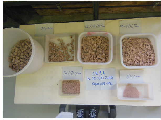
Figure 6.5 : The oedometer test finished at \sigma_a = 0.42 MPa ( Figure 6.4 ): a – A view of the top surface after the test (in contact with the loading plate), and b – The fragments divided into the sieve sizes ( Figure 6.6 ).
