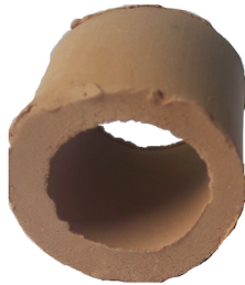
Figure 1.3 : A shell is a tube-shaped particles with large internal void manufactured from COx clay-stone by means of the mechanical and thermic treatments.
