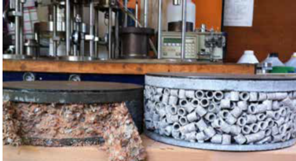
Figure 1.5 : Photo of sample before (right) and after (left) uniaxial compression. Test performed by Euro-Géomat-Consulting EGC (Orléans) on sample with diameter of 30 cm and height of 13.5 cm (Ly, 2018).
