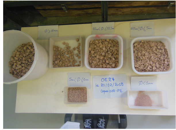
Figure 6.5 : The oedometer test finished at \sigma_n = 0.42 MPa ( Figure 6.4 ): a – A view of the top surface after the test (in contact with the loading plate), and b – The fragments divided into the sieve sizes ( Figure 6.6 ).
