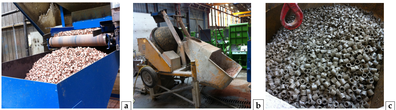
Figure 4.2 : a and b – Photos showing the coating process done at Stradal plant. c – Material used in density measurements – shell in the size d18 with the coating of cement mortar (see Table 4.3 ).
