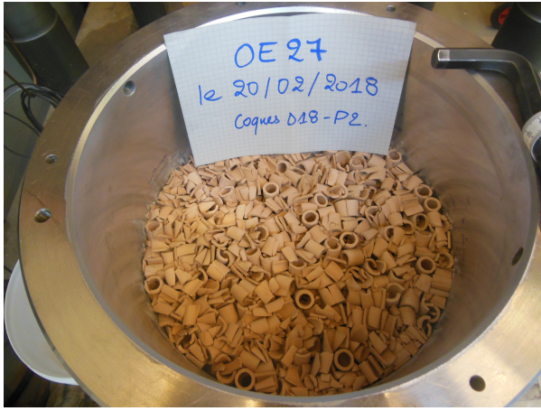
Figure 6.5 : The oedometer test finished at \sigma_n = 0.42 MPa ( Figure 6.4 ): a – A view of the top surface after the test (in contact with the loading plate), and b – The fragments divided into the sieve sizes ( Figure 6.6 ).
