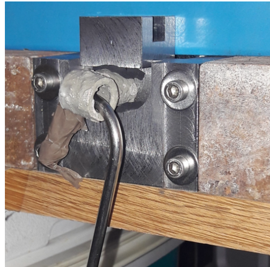
Figure 4.5 : An experimental attempt to extract the shear strength of mortar joints. a – Scheme of loading conditions, and b – the experimental setup presented in the case of base-shaft joint (Figures 4.3c).
