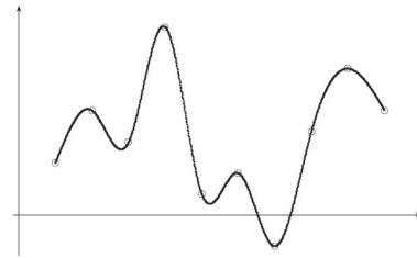
Figure 3.4: Constructed \mathcal{C}^2 using natural cubic spline interpolation
