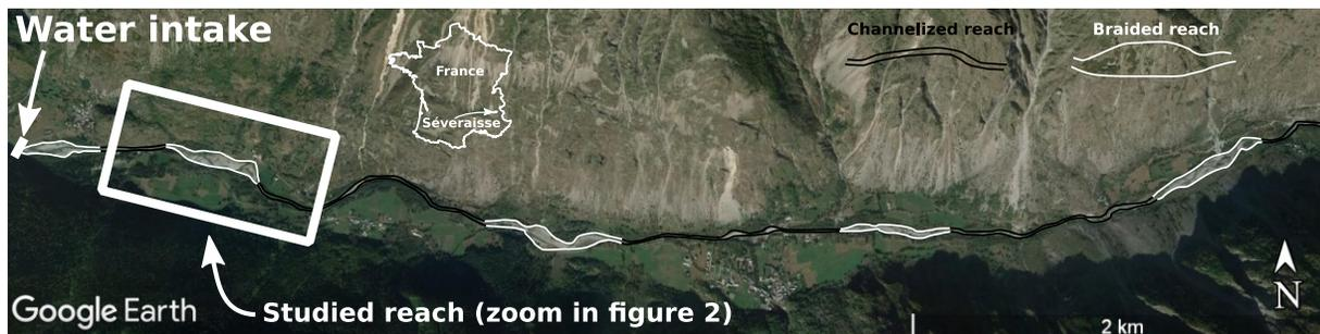
**Figure 4.1:** Braided reaches (white lines) alternating with narrow constrained reaches (black lines) in the Séveraise river (Google earth 2016). A water intake is located downstream the study area.
