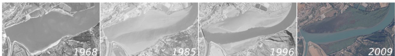
Figure 0.3: Example of siltation on the Escale Dam on the Durance river in the south of France ( 44^{\circ} 05' 08'' \text{ N} , 6^{\circ} 00' 42'' \text{ E} ) built between 1959 and 1963. Aerial photograph were obtained from the IGN website ( http://remonterletemps.ign.fr/ ).
