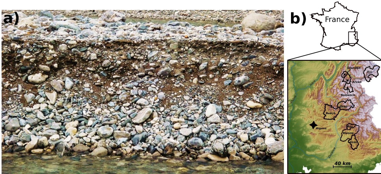
Figure 3.1: a) Picture of a typical gravel bar in a braided reach of the Aigues rivers. A coarse armor layer in surface and large stocks of fine sediments in the subsurface can clearly be distinguished. The picture location is indicated on the right panel by a black star. b) Locations of the alpine catchments used for this study. Note: The Bouinenc, Brusquet, Duyes, Galabre, laval and Moulin catchments are small tributaries of the Bléone rivers.
