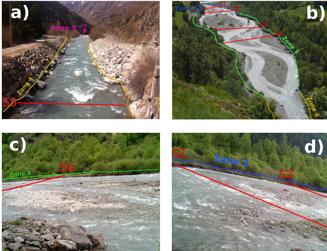
Figure 4.2 : Location of the instruments and measurements within the studied reach of the Séveraise. S1 to S5 correspond to cross-section surveys located from upstream to downstream; (a) is the narrow and paved downstream section where flow rate measurements and bedload sampling were performed, (b) is a view of the braided reach, (c) is a picture taken from a time-lapse camera in the middle of the braided reach and (d) is a picture taken from a time-lapse camera in the upstream part of the braided reach. The five zones used to analyze tracking pebble surveys are indicated with different colors. These zones have different morphologies: zone 1 and 4 are narrow and constrained, zone 2 is the entrance of the braided reach, and zone 3 is the downstream part of the braided reach. Zone 5 is located downstream the gauging station few meters upstream the water intake and is the most downstream prospected zone.
