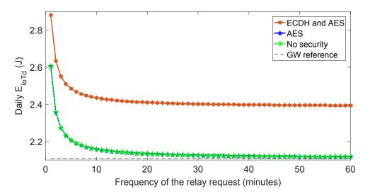
Figure 12: Energy consumption with and without relaying
