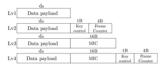
Figure 21: Security overhead for each security level
