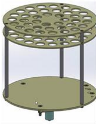
Figure 2. 3. Sample holder for irradiation of ampoules.
