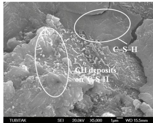
Figure 3. SEM images of the mortar specimens after 28 days of curing OPC [5]
