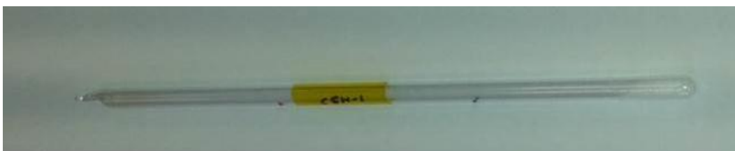
Figure 2. 7. The EPR tube for electron beam irradiation. The yellow part is kapton tape that protects the name. The external diameter of tube is 4 mm.
