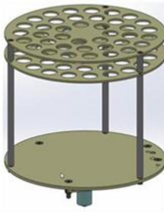
Figure 2. 3. Sample holder for irradiation of ampoules.
