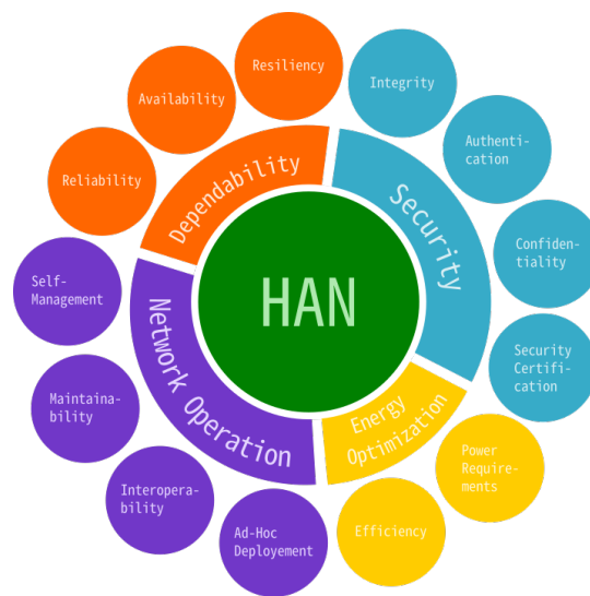
Figure 1.4 – The classification of the main characteristics and requirements for a Home Area Network
