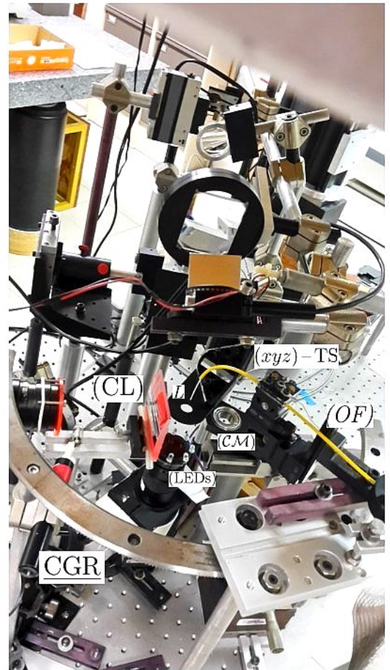
Figure 3.6: The core of the ‘hot bead setup’. ( Left figure ) Schematic of the central part of the device (not to scale). \{(OF) + (st)\} , optic fibre + sewing thread (adjustable tension); CGR circular guide rail; (xyz) -TS, xyz translation stage; \{(BC) + (MO)\}/(SC) bottom camera + microscope objective/side camera; (LEDs) ring encrusted with light-emitting diodes. ( Right figure ) Photograph under actual operating conditions. Same abbreviations plus (CM) cuvette mounting; L lid; (CL) correction lens.
