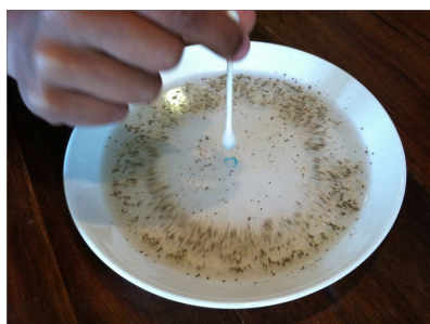
Figure 1.13: Pepper and soap experiment showing the solutal Marangoni effect. Surfactant molecules contained in the drop of washing–up liquid drive an outward solutocapillary flow repelling the pepper flakes towards the edges of the dish. Source: sciencearoundus1.blogspot.com .
