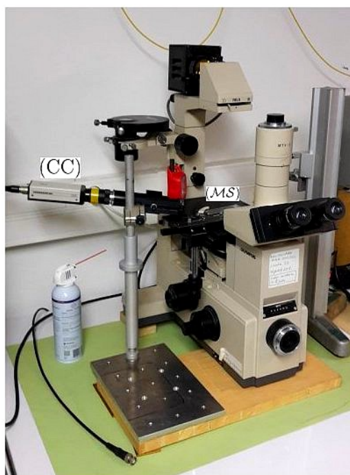
Figure H.1: The bead collage setup. (Top figure) Schematic of the device (not to scale). (MS) microscope slide; (OF) optic fibre; (xyz)-TS, xyz translation stage; (MO) microscope objective; {(CC) + (ET) + (L)}, control camera + extension tube + lens. Step (1): soak the tip of the optic fibre in the glue droplet gd . Step (2): find an isolated sphere in the carbon bead powder cbp and stick it onto the fibre. Pay attention to the bead alignment with the fibre axis. Step (3): cure the adhesive with the 'UV pistol' (image taken from Thorlabs official website). (Bottom figure) Photograph of the setup under actual operating conditions. Same abbreviations.
