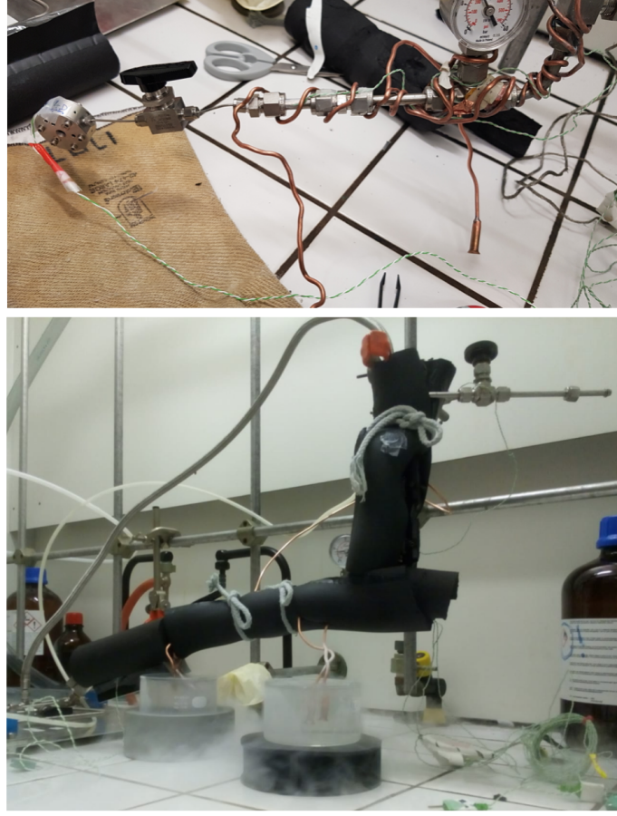
Figure 5.7 – Cooling system of the last part of the filling circuit used in experiment B. Top. Two copper capillaries are coiled around the final portion of the system. The white-green wires are the thermocouples permitting the measurement of the temperature in different portions of the system during the filling procedure. Bottom. The final portion of the system is thermally isolated by a sleeve wrapped around it and secured. The free ends of the two copper capillaries are immersed in a beaker filled with liquid nitrogen.
