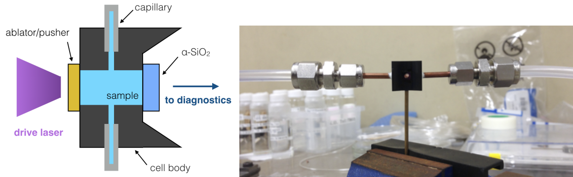
Figure 4.3 – Left. Scheme of the target developed for the laser shock compression of liquid mixtures. Right. Photo of a target connected to plastic tubes to be filled with the liquid sample under study.
