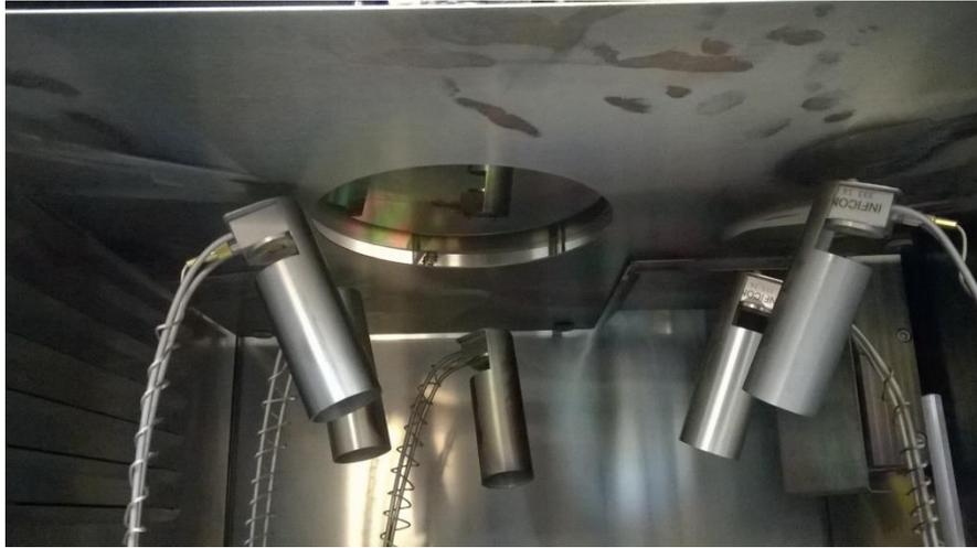
**Figure 53.** Picture of the inside of the reactor (lower part, below the screening shield) highlighting the presence of a white MAI veil covering all the surfaces.
