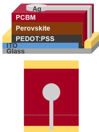
**Figure 94.** Ag top electrode deposition (side and top views of the sample stack).
