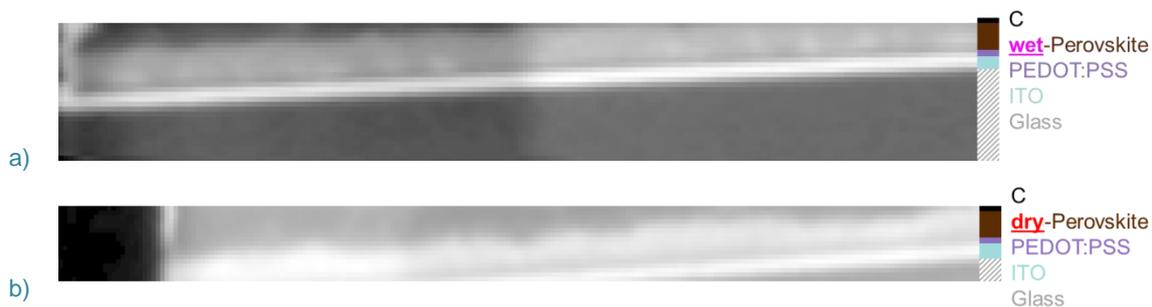
**Figure 80.** Examples of aligned, ODed and cropped STXM images at 490 eV for the a) wet- and b) dry-processed perovskite samples (reminder: what is shown here is just one out of the 116 images of each stack scan).
