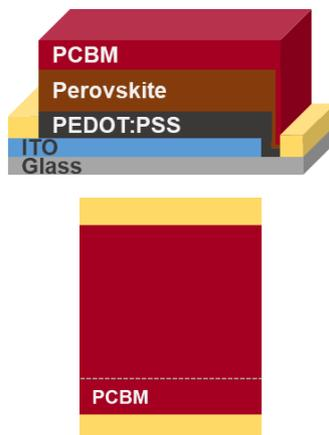
**Figure 93.** PCBM deposition (side and top views of the sample stack).
