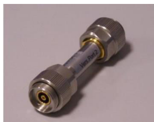
Figure II. 20. Cellule EpsiMu 7 mm ( L = 50 mm)
