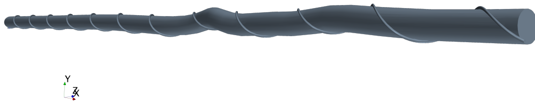
Figure 5.14.: CAD representation of a helically flexed fuel pin and its spacer wire. The lateral displacement of the pin computed by DOMAJEUR2 has been multiplied by 40 to obtain the CAD model presented in this figure.
