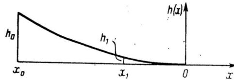
FIGURE 1.7 – Plate with a power-law tapered edge.  $x_1$  and  $h_1$  correspond to the coordinate of the ABH edge and its thickness in the practical case respectively.  $x_0$  is the coordinate of the ABH edge in the ideal case where the thickness is null in this case [127].
