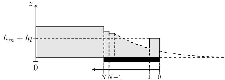
FIGURE 3.6 – Diagram of the spatial discretisation of the ABH with an added mass.
