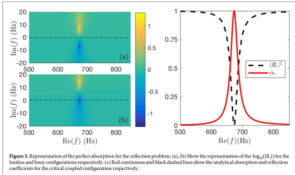
**Figure 3.** Representation of the perfect absorption for the reflection problem. (a), (b) Show the representation of the  $\log_{10}(|R_r|)$  for the lossless and lossy configurations respectively. (c) Red continuous and black dashed lines show the analytical absorption and reflection coefficients for the critical coupled configuration respectively.
