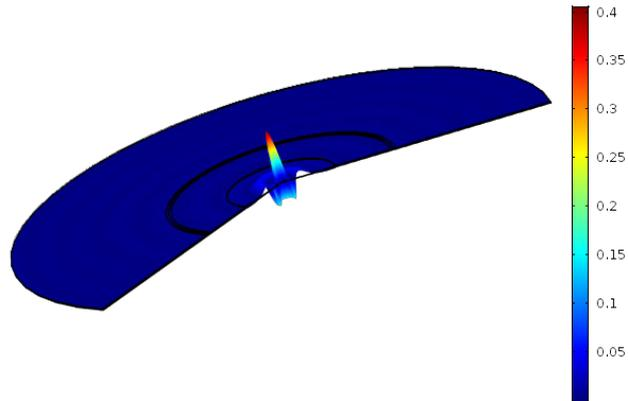
FIGURE 4.11 – Displacement response of the ABH (in m) embedded at the centre of a circular plate for the critically coupled configuration ( $\text{Re}(f) = 580$  Hz,  $\eta_l = 0.45$ ), using a 2D axisymmetric model of solid mechanics in COMSOL software. The concentric incident wave is simulated by imposing a load at the edge of the circular plate.
