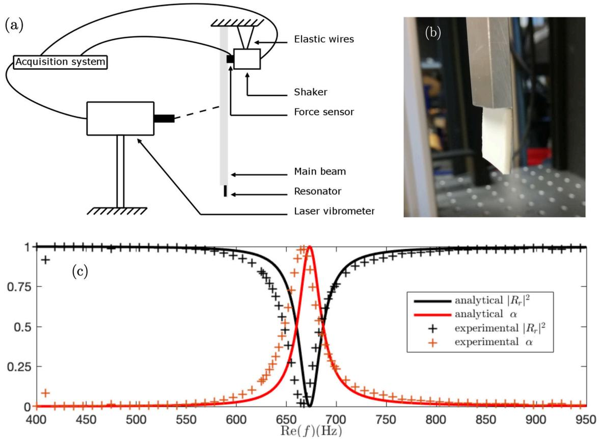
FIGURE 2.6 – (a) Diagram of the experimental set-up. (b) Photograph of the resonator. (c) Black crosses and red open circles show respectively  $|R_r|^2$  and  $\alpha_r$  for the critically coupled configuration measured with the experimental set-up. Black dashed and red continuous lines show  $|R_r|^2$  and  $\alpha_r$  calculated with the analytical model.
