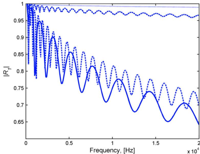
FIGURE 1.8 – Frequency dependence of the reflection coefficient  $|R_1|$  for a beam with an ABH termination covered by a  $700 \mu\text{m}$  absorbing film (solid curve) and  $10 \mu\text{m}$  absorbing film (dash-dotted curve); with an ABH without absorbing film (dashed curve); and for a uniform beam with  $700 \text{ mm}$  absorbing film (dotted curve). [79]
