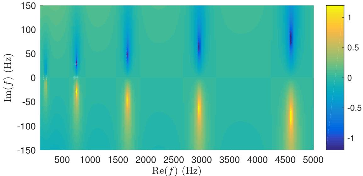
FIGURE 4.5 – Representation of  $\log_{10}(|\tau_0|)$  in the complex frequency plane for the lossless case. The real frequency of each pole corresponds only to the resonance frequency of the axisymmetric modes of the resonator since the incident wave imposes axisymmetric displacements at its edge.
