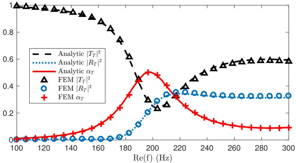
FIGURE 5.4 – Representation of  $|R_T|^2$ ,  $|T_T|^2$  and  $\alpha_T$  around the first eigenfrequency of the critically coupled resonators. Black dashed, blue dotted and red solid lines show the analytical transmission, reflection and absorption coefficients  $|R_T|^2$ ,  $|T_T|^2$  and  $\alpha_T$  respectively, whereas black triangle, blue circles and red crossed lines correspond to the transmission, reflection and absorption coefficients computed by means of a FEM model.
