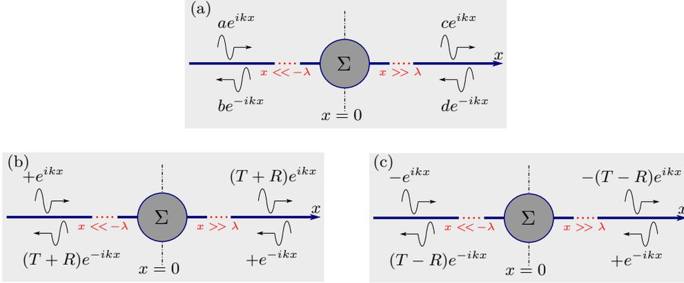
FIGURE 2.1 – (a) Diagram of the scattering process. (b) Symmetric and (c) antisymmetric uncoupled sub-problems for the case of a mirror-symmetric scatterer  $\Sigma$ . The time convention is  $e^{-i\omega t}$ . (adapted from [125])
