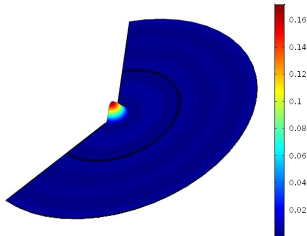
FIGURE 4.7 – Displacement response (in m) of the circular resonator embedded at the centre of a circular plate for the critically coupled configuration ( $\text{Re}(f) = 184.9$  Hz,  $\eta_l = 2$ ), using a 2D axisymmetric model of solid mechanics in COMSOL software. The concentric incident wave is simulated by imposing a load at the edge of the circular plate.
