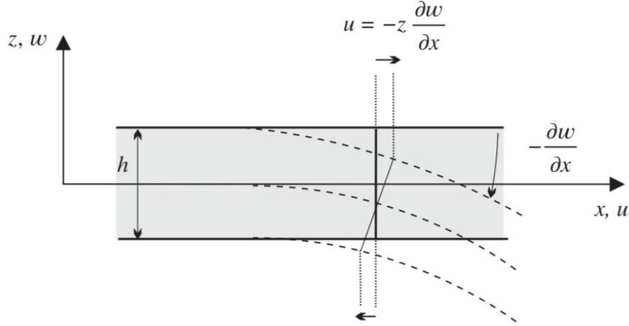
FIGURE 4.1 – Kinematic of the thin plate deformation (from [81]).
