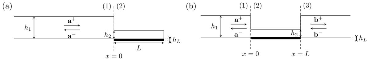
FIGURE 2.2 – Diagrams of the 1D configurations analysed for the reflection and transmission problems for flexural waves. (a) Configuration for the reflection problem. (b) Configuration for the transmission problem.
