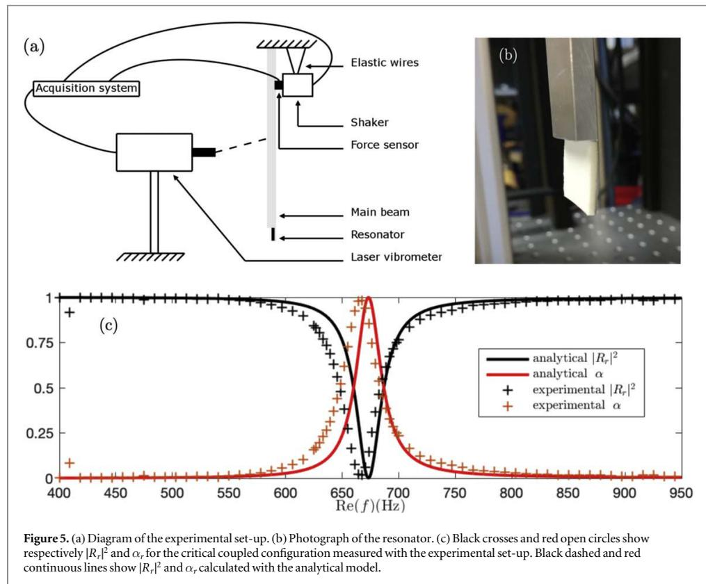
**Figure 5.** (a) Diagram of the experimental set-up. (b) Photograph of the resonator. (c) Black crosses and red open circles show respectively  $|R_r|^2$  and  $\alpha_r$  for the critical coupled configuration measured with the experimental set-up. Black dashed and red continuous lines show  $|R_r|^2$  and  $\alpha_r$  calculated with the analytical model.
