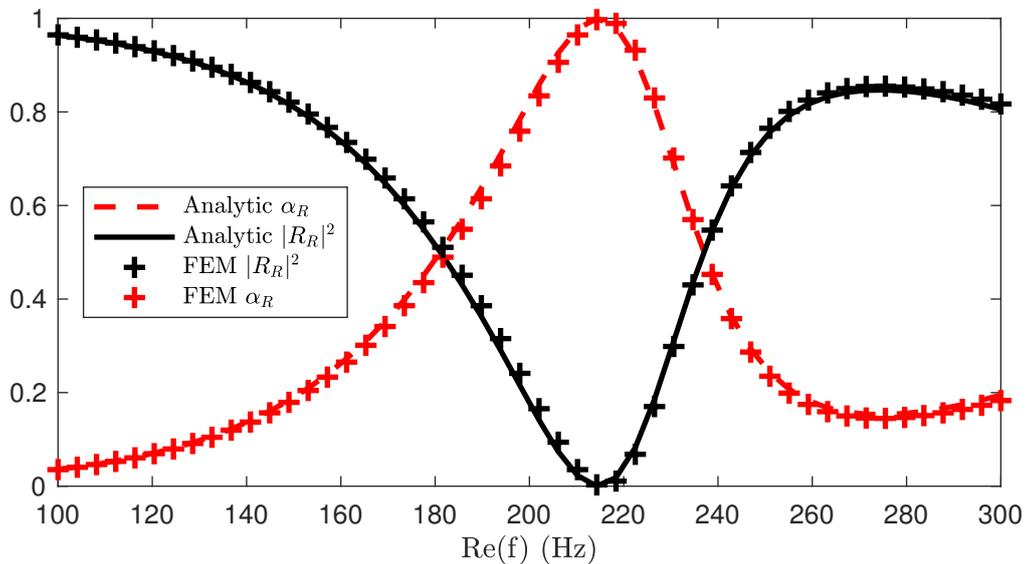
FIGURE 5.8 – Representation of  $|R_R|^2$  and  $\alpha_R$  around the first eigenfrequency of the critically coupled resonators centred in unit cells of width  $d_x = 24$  cm and  $y_0 = 16.3$  cm. Black and red solid lines show the analytical reflection and absorption coefficients  $|R_R|^2$  and  $\alpha_R$  respectively, whereas black and red crossed lines correspond to the reflection and absorption coefficients computed by means of a FEM model respectively.
