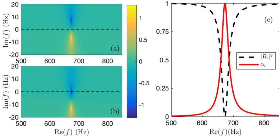
FIGURE 2.4 – Representation of the perfect absorption for the reflection problem. (a), (b) show the representation of the  $\log_{10}(|R_r|)$  for the lossless and lossy configurations respectively. (c) Red continuous and black dashed lines show the analytical absorption and reflection coefficients for the critical coupled configuration respectively.
