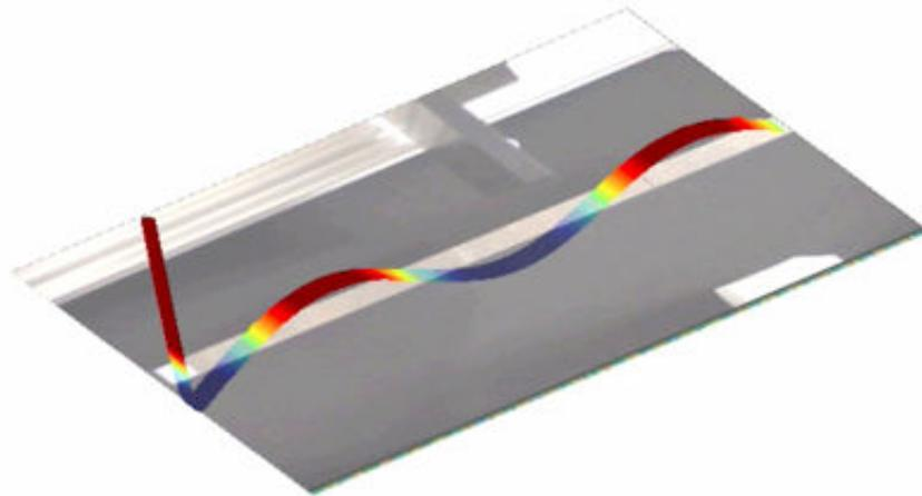
FIGURE 2.7 – Snapshot of the displacement response of the beam system measured with the experimental set-up at 800Hz. The critically coupled resonator is located on the left-hand of the beam system.
