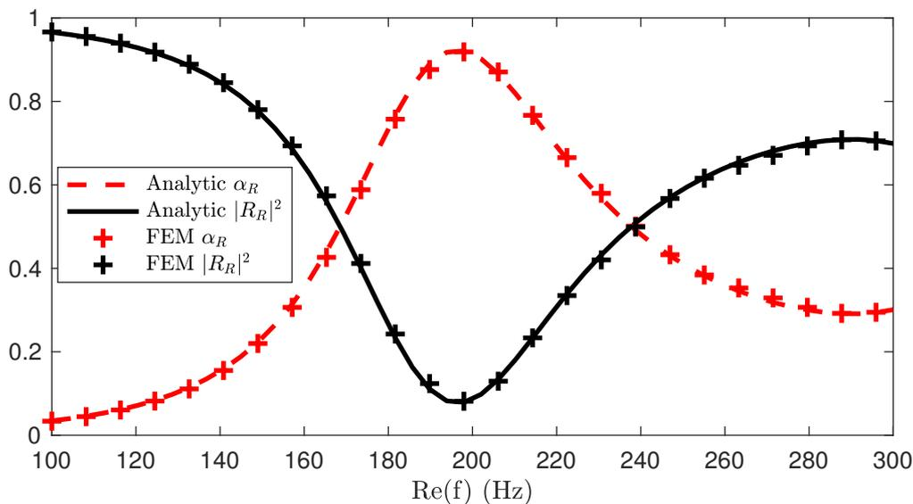
FIGURE 5.6 – Representation of  $|R_R|^2$  and  $\alpha_R$  around the first eigenfrequency of the critically coupled resonators placed in unit cells of width  $d_x = 24$  cm and  $y_0 = 12$  cm. Black and red solid lines show the analytical reflection and absorption coefficients  $|R_R|^2$  and  $\alpha_R$  respectively, whereas black and red crossed lines correspond to the reflection and absorption coefficients computed by means of a FEM model respectively.
