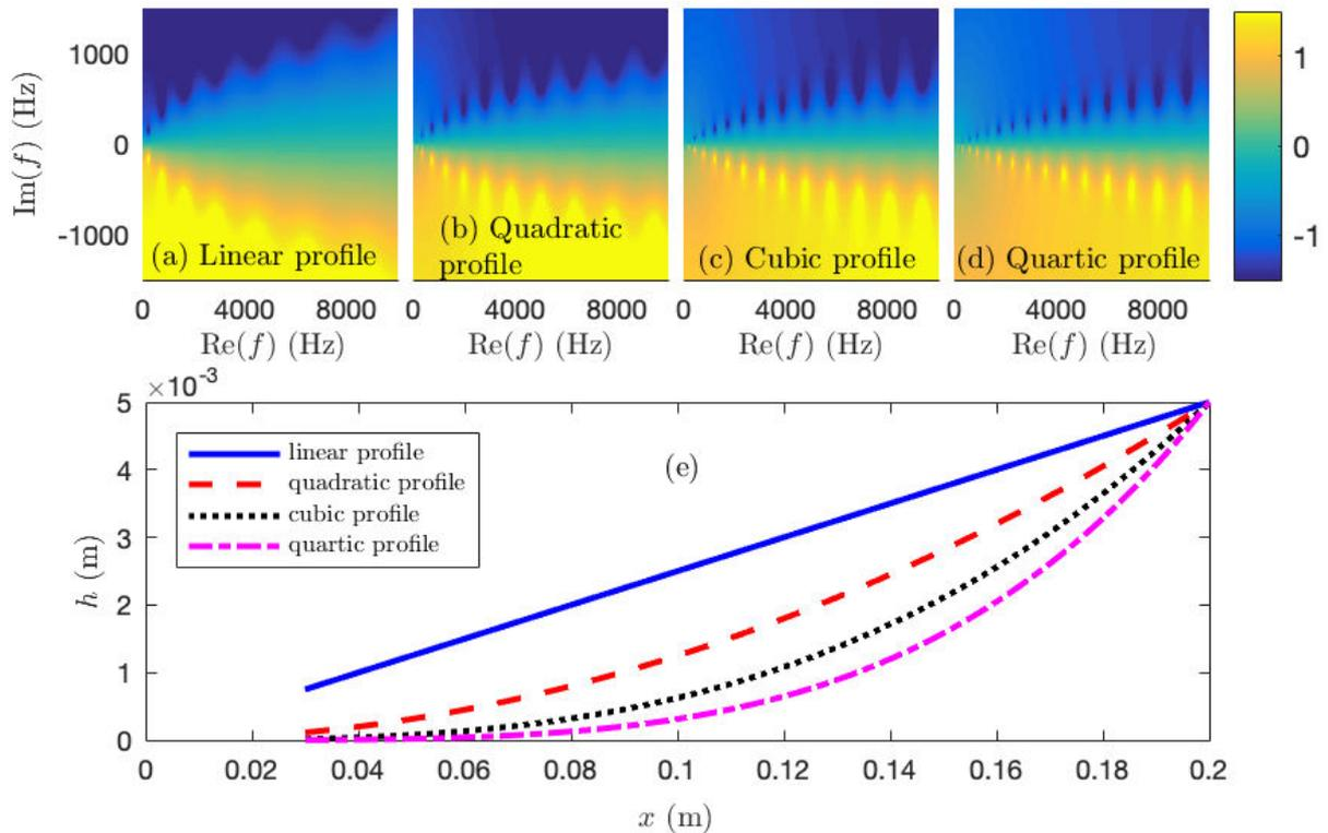
FIGURE 3.2 – (a)-(d) Representation of  $\log_{10}(|R_N|)$  in the complex frequency plane for different thickness profiles of ABH in the lossless case (linear, quadratic, cubic and quartic thickness profiles, respectively). (e) Thickness profiles of the ABH studied in (a)-(d).
