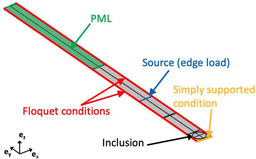
FIGURE 5.7 – 3D FEM model of the unit cell of the infinite array of inclusions used in COMSOL software to numerically compute  $|R_R|^2$  and  $\alpha_R$ . The periodicity along  $\mathbf{e}_x$  is simulated using Floquet conditions and the semi-infinite length along  $\mathbf{e}_y$  with Perfectly Matched Layers (PML). The simply supported condition is simulated by imposing a displacement equal to 0 along  $\mathbf{e}_z$  at the corresponding face.
