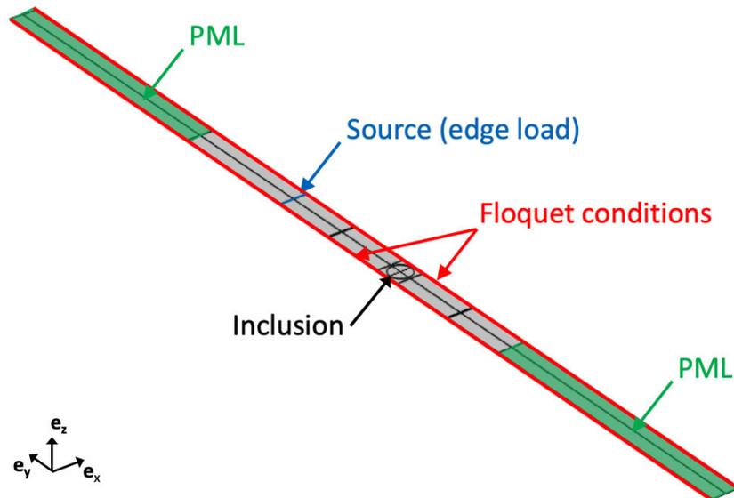
FIGURE 5.5 – 3D FEM model of the unit cell of the infinite array of inclusions used in COMSOL software to numerically compute  $|R_T|^2$ ,  $|T_T|^2$  and  $\alpha_T$ . The periodicity along  $\mathbf{e}_x$  is simulated using Floquet conditions and the infinite length along  $\mathbf{e}_y$  with Perfectly Matched Layers (PML).
