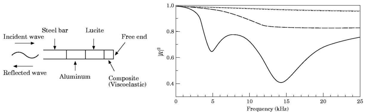
FIGURE 1.5 – Diagram of a graded impedance interface at the edge of a steel bar [181] (left). Reflected energy by four configurations of graded edges of a steel bar: ( $\cdot \cdot \cdot$ ) steel bar; ( $- - -$ ) steel bar, Al; ( $- \cdot - \cdot -$ ) steel bar, Al, Lucite; ( $- - -$ ) steel bar, Al, Lucite, Composite. (right)
