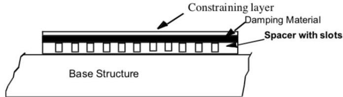
FIGURE 1.3 – Diagram of a stand-off layer damping system. [151]
