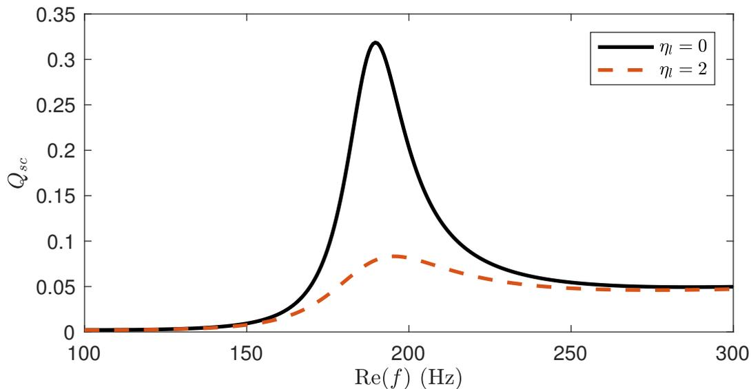
FIGURE 4.8 – Representation of  $Q_{sc}$  in the lossless (continuous black line) and lossy (red dashed line,  $\eta_l = 2$ ) cases for an incident wave defined by a Bessel function of the first kind at the order  $n = 0$ . The parameters of the inclusion are given in Tab. 4.1. The lossy case corresponds to the critically coupled configuration of the inclusion when the incident wave is described by a Hankel function of the second kind  $H_n^{(2)}(x)$ .
