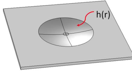
FIGURE 1.9 – Diagram of a typical 2D circular ABH with a radially dependent thickness profile  $h(r)$  and a central plateau. (adapted from [41])
