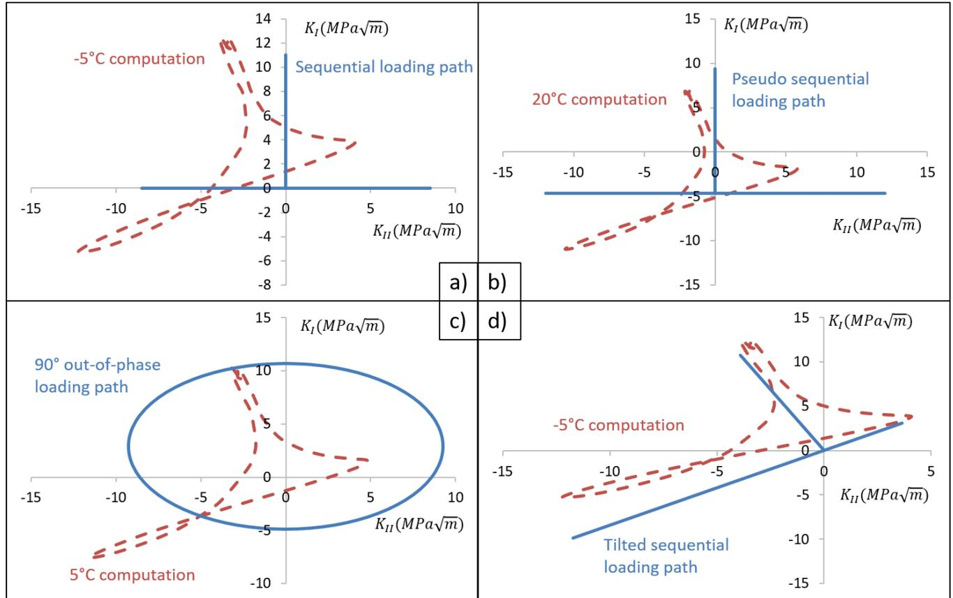
Figure 6.8: Examples of computed and tested loading paths. Computations at the deepest point of a  $10\text{ mm}$  deep squat crack, loaded with a TGV train in a straight line, at various operating temperatures. a) sequential path applied to exp. 19. b) pseudo sequential path applied to exp. 6. c)  $90^\circ$  out-of-phase path applied to exp. 13. d) tilted sequential path applied to exp. 16. Negative values of  $K_I$  are plotted to account for compression.
