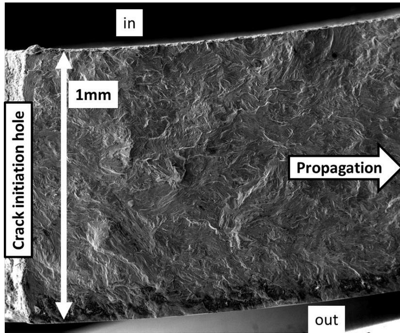
Figure 6.42: Fracture surface of sequential experiment  $N^{\circ}9$  ( $F = +13/0 \text{ kN}$ ,  $C = \pm 90 \text{ Nm}$ ) near the crack initiation hole. The scale is given by the  $1 \text{ mm}$  thickness of the samples.
