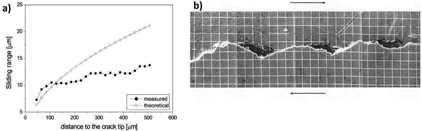
Figure 2.27: (a) comparison of measured in-plane sliding displacement jumps with LEFM predictions, from [Bertolino and Doquet, 2009], (b) *in situ* SEM (Scanning Electron Microscope) image of a crack under mode II loading from [Pinna and Doquet, 1999], 5  $\mu\text{m}$  grid pitch..
