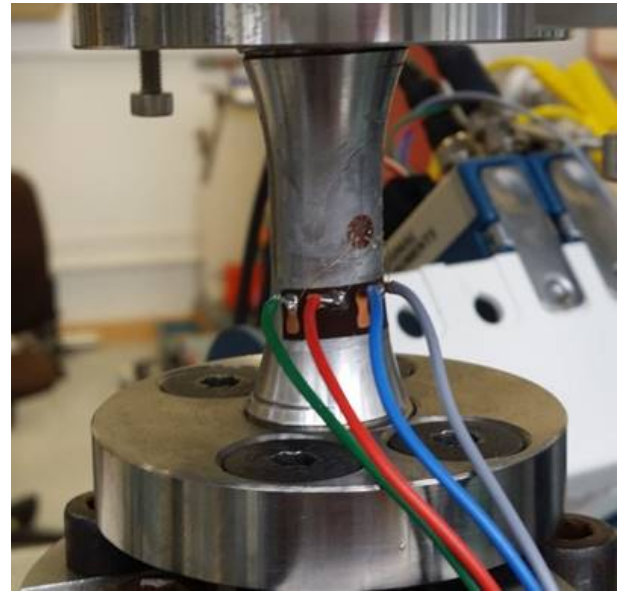
Figure 3.10: Cyclic shear test specimens: drawing and experimental setup.
