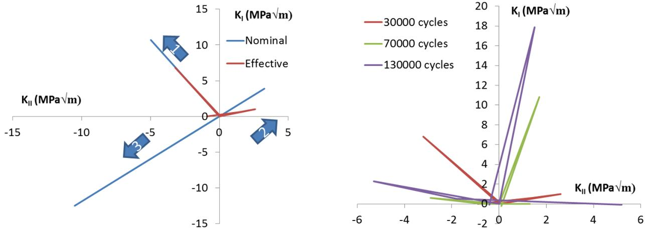
Figure 6.33: Loading paths for sequential experiment  $N^\circ 16$  on a tilted precrack ( $F = +10/0 \text{ kN}$ ,  $C = +45/-145 \text{ Nm}$ ) before bifurcation, at cycle 30000 (left), and effective loading paths for various cycles (bifurcation occurred shortly after cycle 30000) (right).
