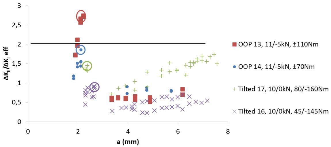
Figure 6.41: Evolution of  $\Delta K_{II}^{effective}/\Delta K_I^{effective}$  as a function of the crack length for 90 ° out-of-phase (OOP) and sequential experiments on tilted precracks. Bifurcations are marked by circles.
