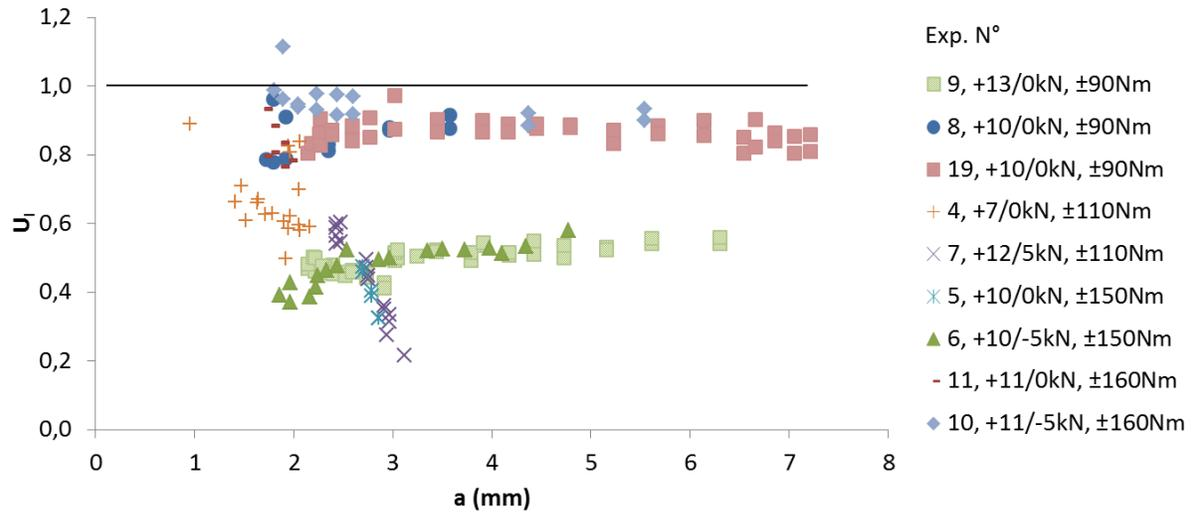
Figure 6.35:  $U_I$  as a function of the crack length for sequential experiments without bending correction. Experiments leading to long coplanar growth are in full symbols, and the other in line-made symbols.
