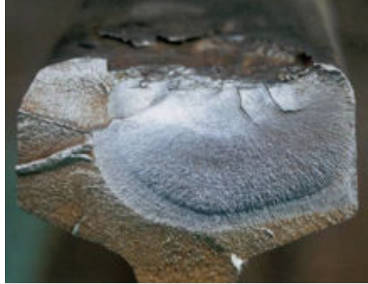
FIGURE 1 – Fissure de type Squat.
