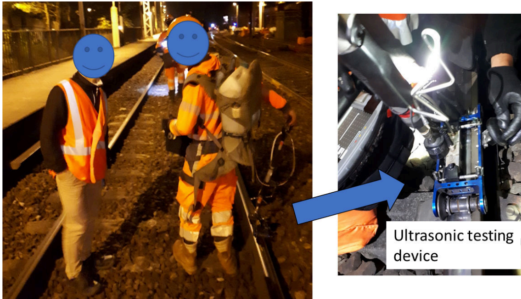
Figure 1.8: Ultrasonic testing of a rail: a cart containing the transmitter and receptor is pushed manually over the track.
