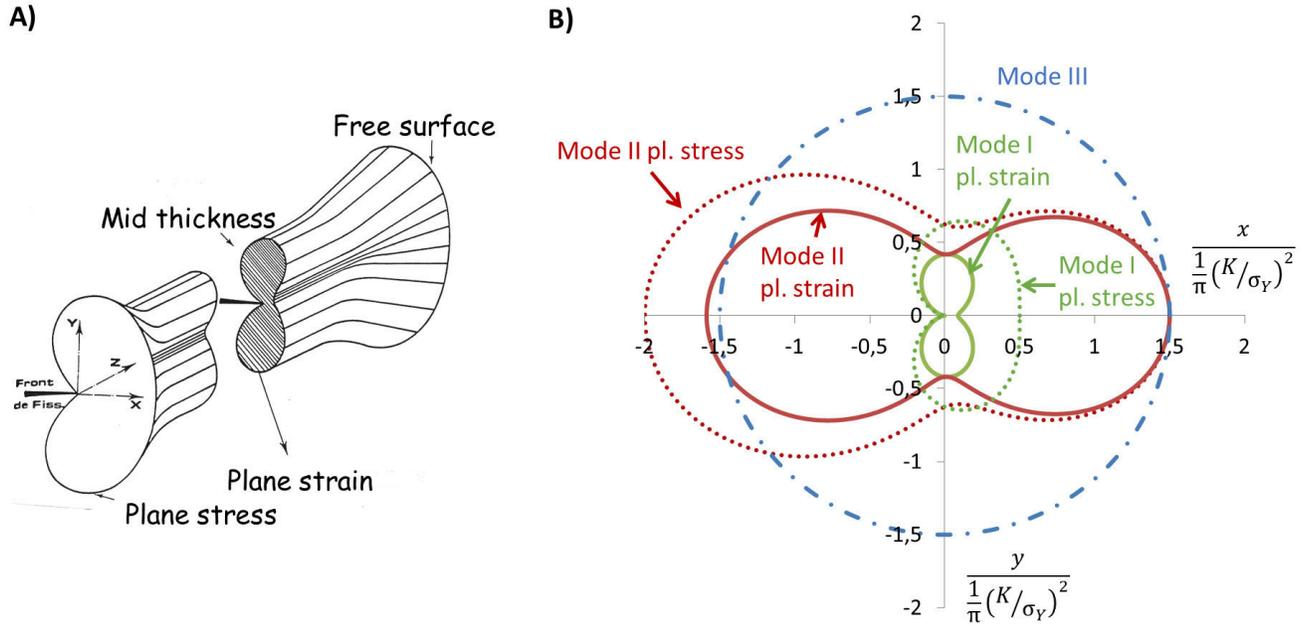
Figure 2.9: Shape of the monotonic plastic zone, under plane stress (in the bulk) or plane strain (on the surface) in mode I (A&B), mode II (B) and mode III (B).  $\nu = 0.29$
