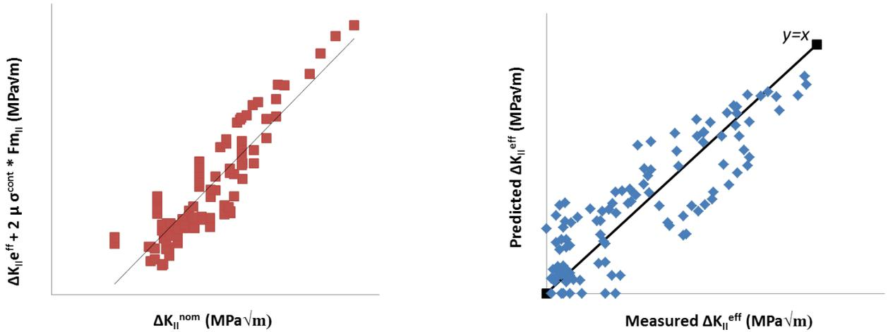
Figure 6.68: Influence of  $\Delta K_{II}^{nom}$  on  $\Delta K_{II}^{eff}$  when removing the effect of the contact stress (a) . Predicted (eq. 6.30) versus measured  $\Delta K_{II}^{eff}$  (b). *No data for confidentiality reasons.*
