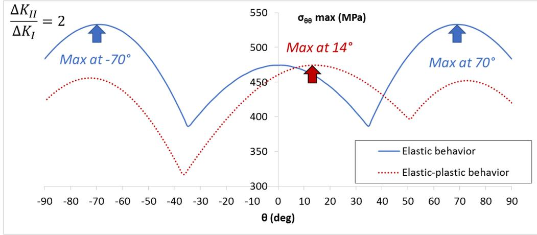
Figure 6.5: Evolution  $\sigma_{\theta\theta}(t)$  extracted at an angle  $\theta$  ahead of the crack tip, for  $\Delta K_{II}/\Delta K_I = 2$ , with an elastic or elastic-plastic behavior.
