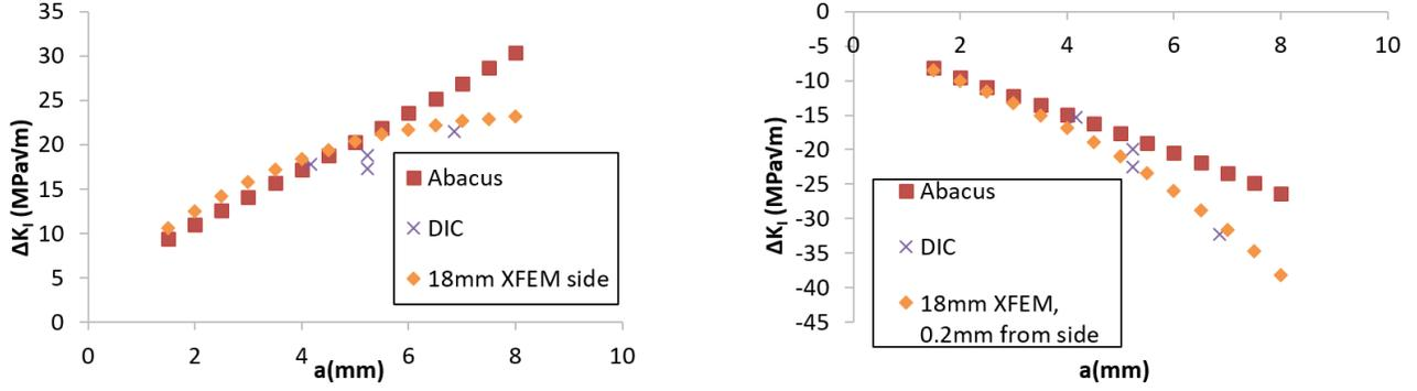
Figure 6.10: Left:  $K_I^{nom}$  estimated using DIC, Erdogan's abacus, and XFEM computations (uniform displacement of a 18 mm half height tube) for a tensile load, as a function of the crack length. Right:  $K_{II}^{nom}$  estimated using DIC, Erdogan's abacus, and XFEM computations for a shear load, as a function of the crack length.
