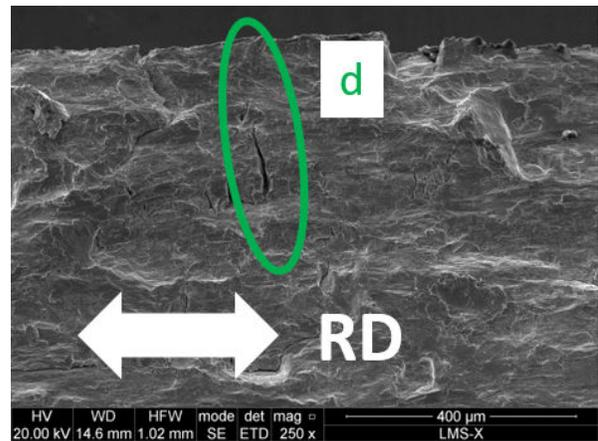
Figure 3.14: Left: broken inclusion in sample  $N^{\circ}3$ ,  $\Delta\tau = 580MPa$  and  $\sigma_n = 0$ . Right: transversal crack in sample  $N^{\circ}7$ ,  $\Delta\tau = 628Pa$  and  $\sigma_n = 90MPa$ .
