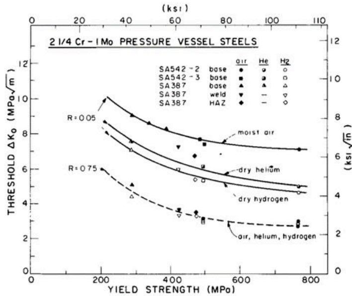
Fig. 6—Variation of threshold  $\Delta K_0$  values for as-received 2 1/4 Cr-1 Mo pressure vessel steels with yield strength. Data for  $R = 0.05$  and  $0.75$  in moist air, dry hydrogen and dry helium environments.
