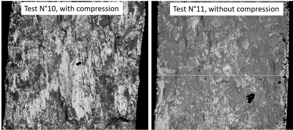
Figure 6.55: Oxidized areas on the fracture surface of test  $N^{\circ}10$  ( $F = +11/-5 \text{ kN}$ ,  $C = \pm 160 \text{ Nm}$ ) (left) and  $N^{\circ}11$  ( $\pm 160 \text{ Nm}$ ,  $11/0 \text{ kN}$ ) (right) with BSE.
