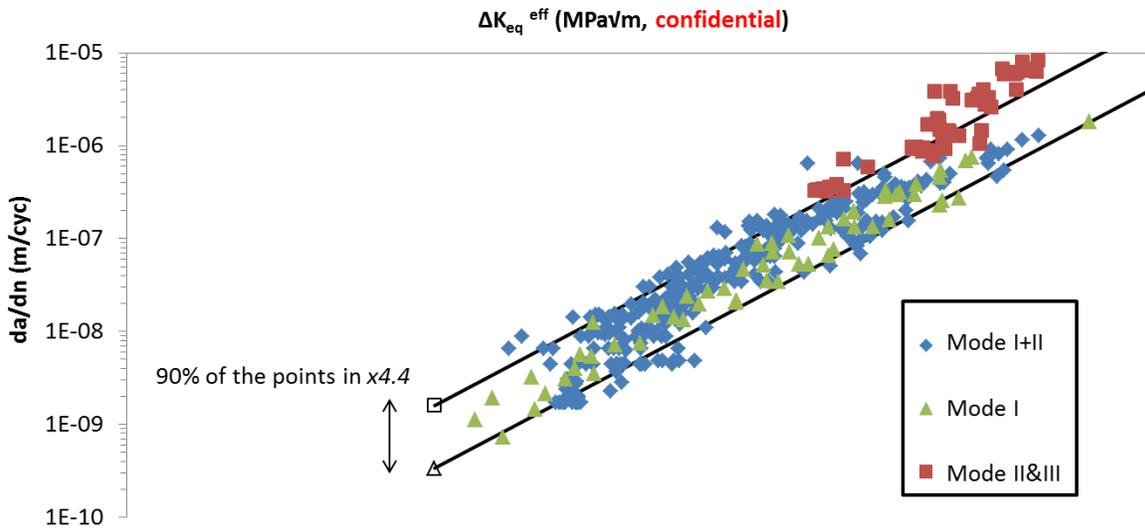
Figure 6.60: Crack growth rates for all the non-proportional mixed-mode I + II experiments as a function of  $\Delta K_{eq}^{eff}$ , and corresponding 90% upper and lower envelopes. The pure mode I and non-proportional mixed-mode I + II data are superimposed.
