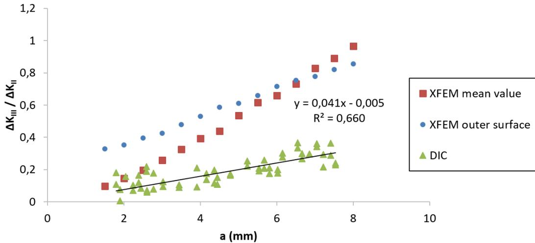
Figure 6.40: Evolution of  $\Delta K_{III} / \Delta K_{II}$  as a function of the crack length, mean value along the front computed by XFEM, value on the outer surface computed by XFEM and value measure on the outer surface by DIC during experiments 10 and 19.
