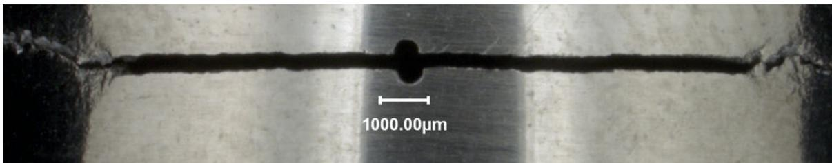
Figure 6.20: Crack path for pseudo sequential experiment  $N^{\circ}9$ .  $F = +13/0 \text{ kN}$ ,  $C = \pm 90 \text{ Nm}$ .
