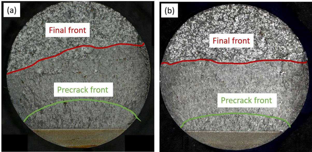
Figure 7.7: Precrack and final crack front of sequential mixed-mode I + II & III test  $N^{\circ}1$  ( $F = 17/ - 7 \text{ kN}$ ,  $C = 33/ - 31 \text{ Nm}$ ) (a) and test  $N^{\circ}2$  ( $F = 17/0 \text{ kN}$ ,  $C = 33/ - 31 \text{ Nm}$ ) (b).
