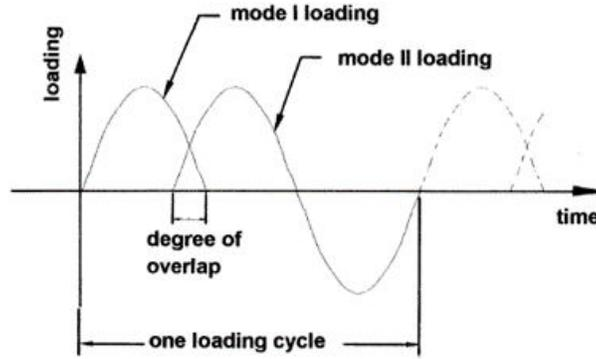
Figure 6.1: Sequential I + II loading with an overlap.
