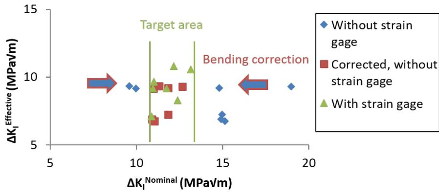
Figure 6.14:  $\Delta K_I^{nominal} - \Delta K_I^{effective}$  curve during precracking.
