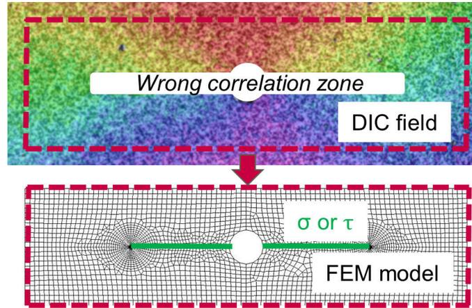
Figure 3.23: Principle of the DIC-FEM coupling.
