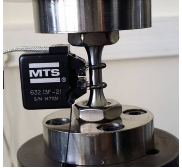
Figure 3.6: Cyclic tensile test specimens: drawing and experimental setup.
