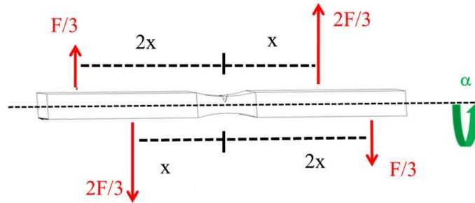
Figure 5.1: Asymmetric four point bending device.
