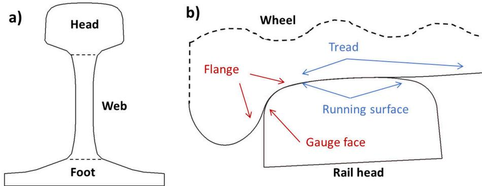
Figure 1.1: Rail nomenclature (a). Rail-wheel contact areas (b).
