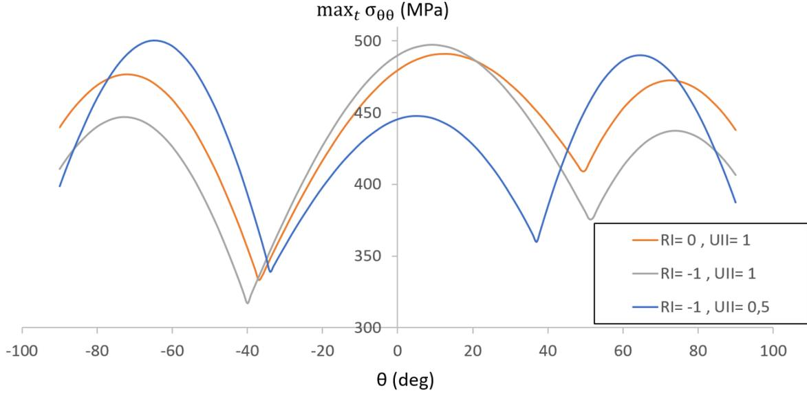
Figure 6.63: Evolution of the maximum of the tangential stress  $\sigma_{\theta\theta}$  a function of the direction, at  $40 \mu m$  from the crack tip for an **elastic plastic** behavior and pseudo sequential mode I + II loadings at  $\Delta K_I^{eff} = 8.1 MPa\sqrt{m}$  &  $\Delta K_{II}^{eff} = 16.1 MPa\sqrt{m}$ .
