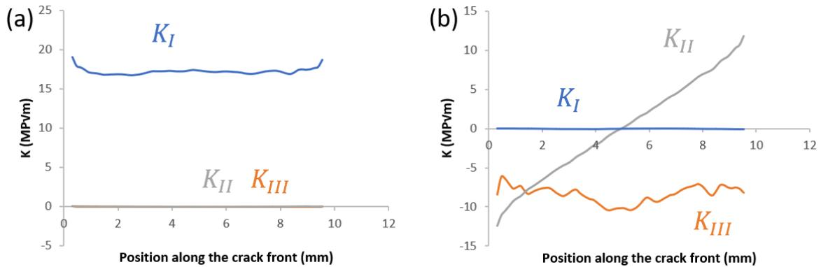
Figure 7.11: Evolution of the SIFs along the precrack front a) at peak tensile load and b) at maximum torque for the sequential mixed-mode I + II & III test  $N^{\circ}1$ , for a 17 kN tensile load, and a 35 Nm torque.
