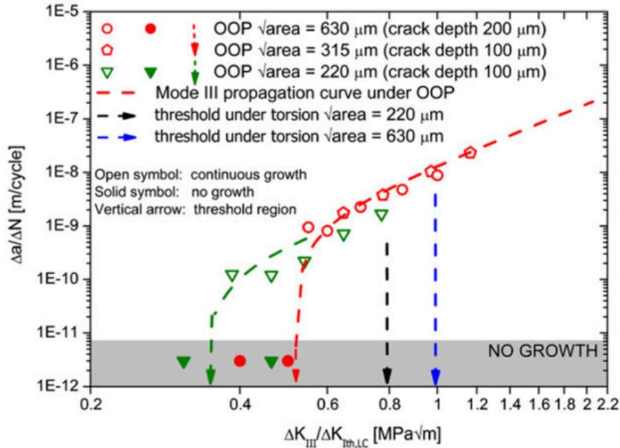
Figure 2.40: Crack growth rate as a function of  $\Delta K_{III}^{nom}$  for pure mode III and  $90^\circ$  out-of-phase mode III + compression (noted "OOP"), with various notch sizes. "Continuous growth" means stable coplanar growth.
