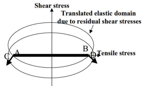
Figure 3.22: Coupling between shear and tensile plastic flows at the crack tip during a sequential experiment. Image from [Doquet and Pommier, 2004].
