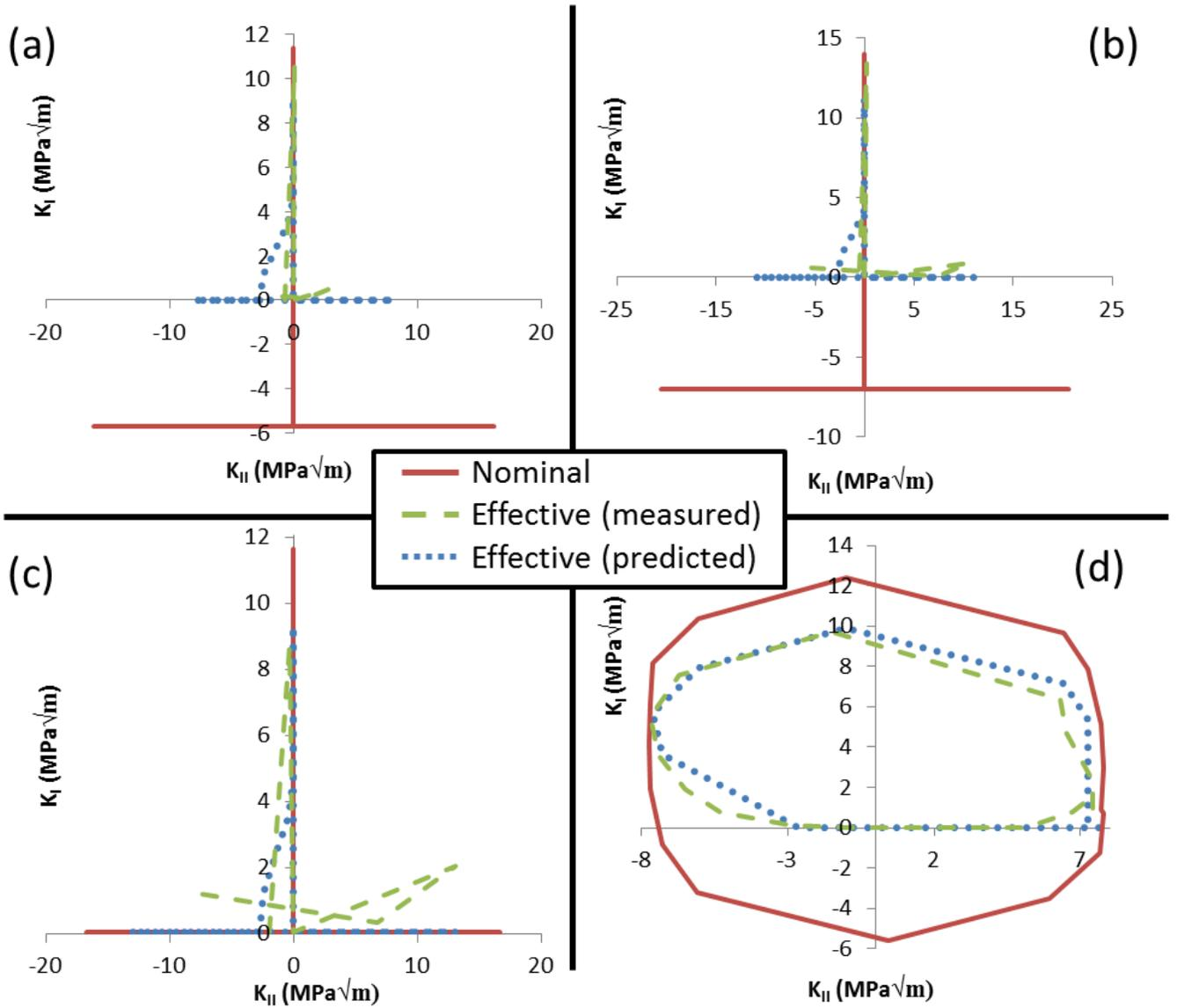
Figure 7.4: Evolution of  $K^{nom}$ ,  $K^{eff}$  measured by DIC, and  $K^{eff}$  predicted using the proposed approach in the  $K_I - K_{II}$  space, for various experiments: experiment  $N^{\circ}10$  ( $F = +11/-5$ ,  $C = \pm 160 Nm$ ) at cycle 2000 (a) & 11 000 (b), experiment  $N^{\circ}11$  ( $F = +11/0 kN$ ,  $C = \pm 160 Nm$ ) at cycle 2000 (c) and  $90^{\circ}$  out-of-phase experiment  $N^{\circ}14$  ( $F = +11/-5 kN$ ,  $C = \pm 70 Nm$ ) at cycle 5000 (d).
