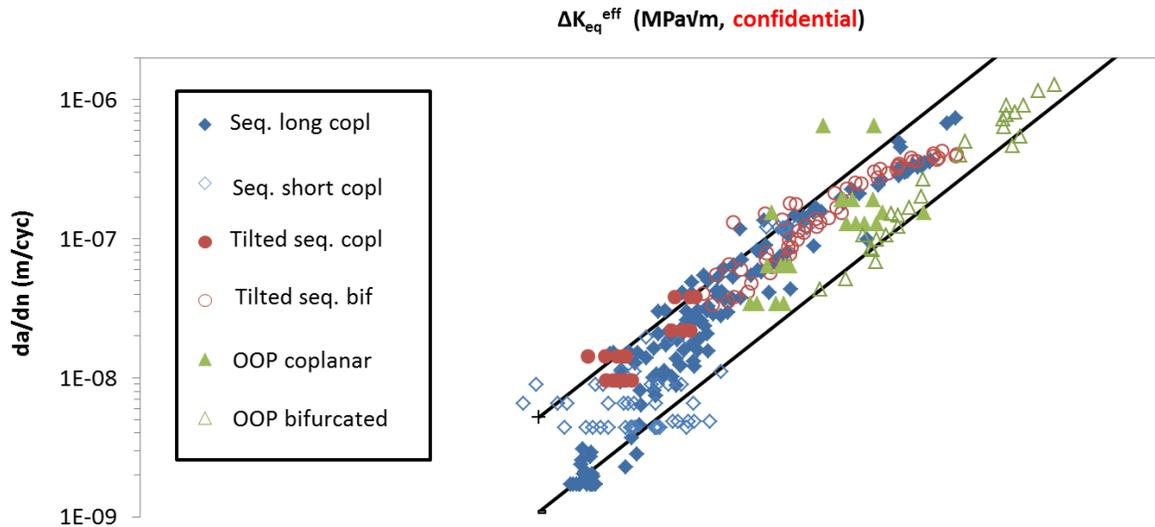
Figure 6.61: Crack growth rates for all the non-proportional mixed-mode I + II experiments as a function of  $\Delta K_{eq}^{eff}$ , depending on the testing conditions and crack path. Seq. long/short copl: sequential experiments giving rise to a long/short coplanar growth. Tilted seq. copl/bif: tilted sequential experiments, before/after bifurcation. OOP coplanar/bifurcated: 90 ° out-of-phase experiments before/after bifurcation.
