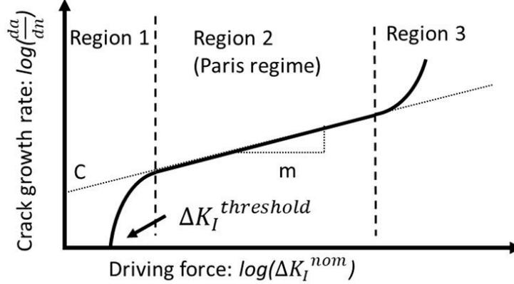
Figure 2.17: Typical mode I crack growth kinetics.
