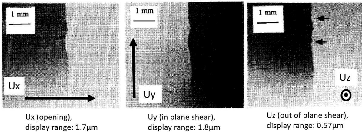
Figure 2.28: Displacements maps along the three directions, obtained by electro-optic holographic interferometry, for  $\Delta K_{II}^{nom} \approx 5.6 \text{ MPa}\sqrt{\text{m}}$ , from [Gross et al., 1995].
