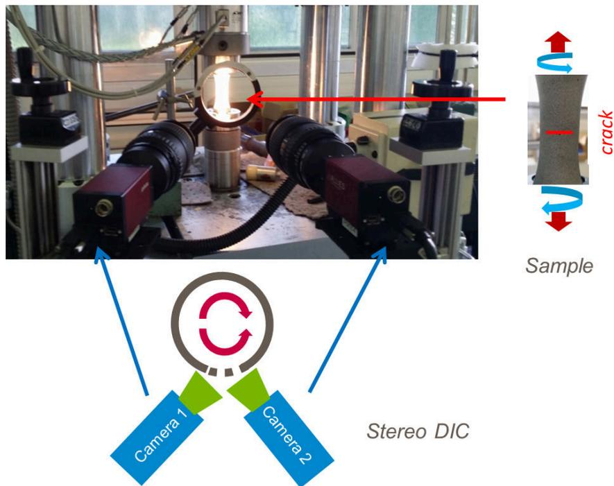
Figure 6.7: Experimental setup with the two cameras.
