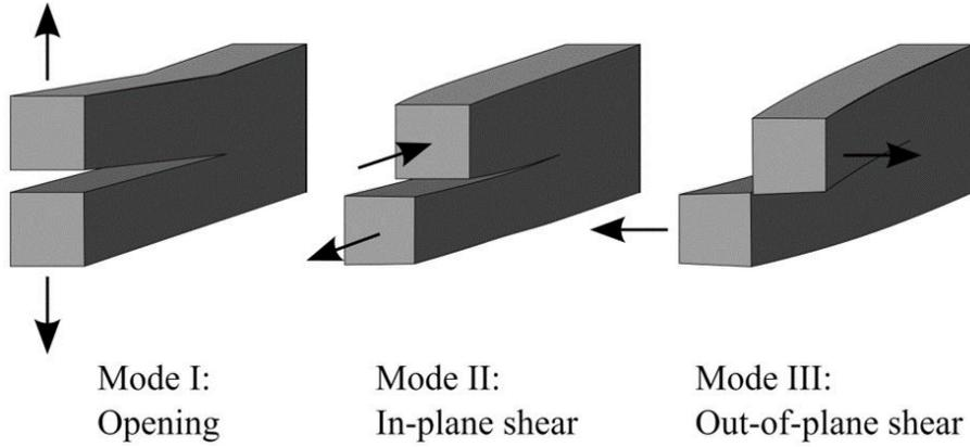
Figure 2.7: Displacements induced by the three modes.
