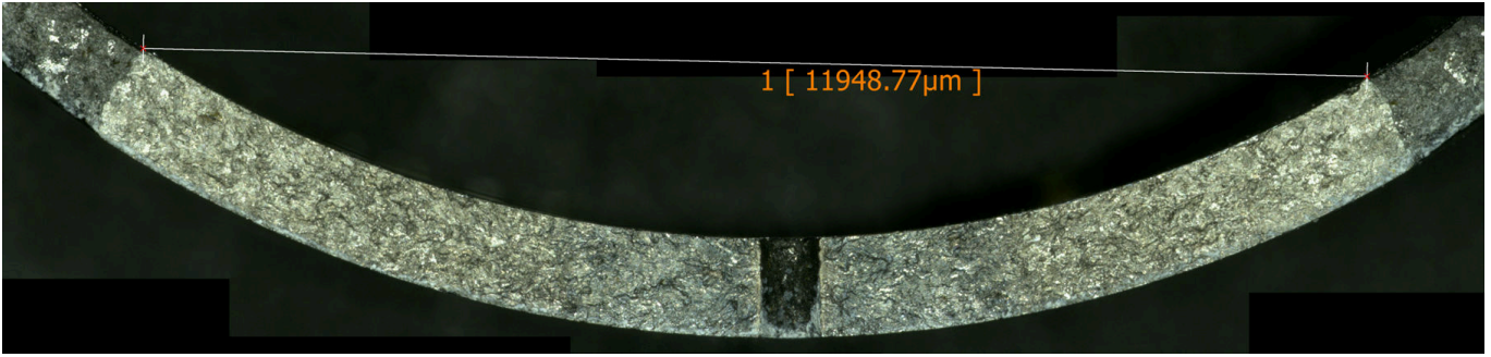
Figure 6.44: Fracture surface of sequential experiment N^{\circ}9 ( F = +13/0 kN, C = \pm 90 Nm) obtained with an optical microscope.
