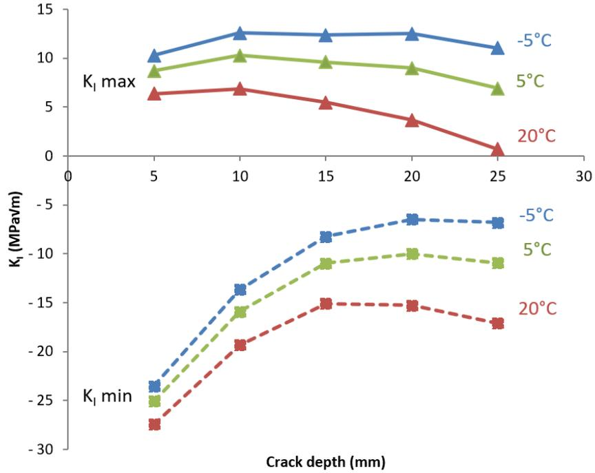
Figure 4.4: Evolution of  $K_I^{max}$  and  $K_I^{min}$  at the deepest point of a Squat-type crack, as a function of the crack depth, with residual stresses and for various operating temperature (20 °C corresponding to the reference state)
