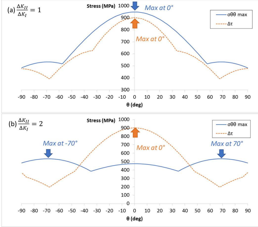
Figure 6.4: Evolution  $\sigma_{\theta\theta}(t)$  and  $\Delta\tau$  extracted at an angle  $\theta$  ahead of the crack tip, for  $\Delta K_{II}/\Delta K_I = 1$  (a) and  $\Delta K_{II}/\Delta K_I = 2$  (b).
