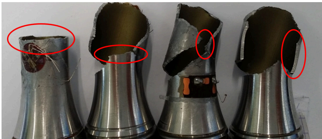
Figure 3.11: Various crack paths, from left to right: long transversal growth, short transversal growth, short longitudinal growth and long longitudinal growth.
