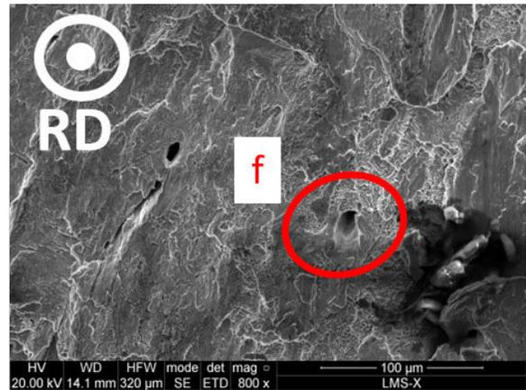
Figure 3.15: Left: longitudinal crack in sample  $N^{\circ}8$ ,  $\Delta\tau = 628Pa$  and  $\sigma_n = 150MPa$ . Right: detached inclusion in sample  $N^{\circ}8$ ,  $\Delta\tau = 628Pa$  and  $\sigma_n = 150MPa$ .
