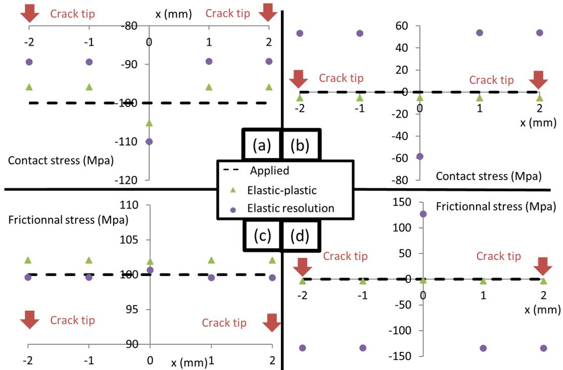
Figure 3.25: Estimated profile of the contact/friction stresses along the crack faces, for the hole-free model shown on figure 3.20. (a): Mode I  $\Delta K_I^{FEM} = 10 MPa\sqrt{m}$ , 100  $MPa$  compression. (b) Mode I,  $\Delta K_I^{FEM} = 30 MPa\sqrt{m}$ , no compression. (c): Mode II  $\Delta K_{II}^{FEM} = 1.9 MPa\sqrt{m}$ , 100  $MPa$  friction. (d): Mode II  $\Delta K_{II}^{FEM} = 20 MPa\sqrt{m}$ , no friction.
