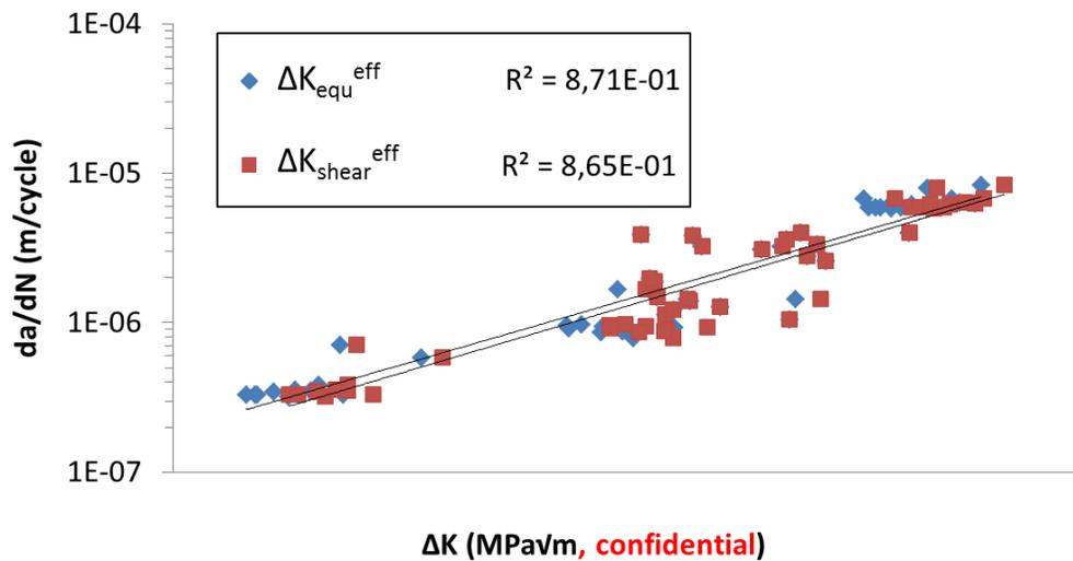
Figure 5.14: Experimental and predicted crack growth rate as a function of  $\Delta K_{shear}^{eff}$  and  $\Delta K_{equ}^{eff}$ , with  $\beta = 1.25$ .
