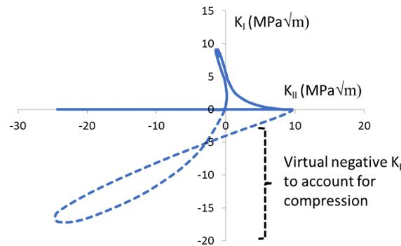
Figure 2.15: Loading path in  $K_I - K_{II}$  space at the deepest point of the crack front ( $90^\circ$ , see on fig. 2.13). TGV motor load ( $8.5 \text{ T}$ ).  $30 \text{ MPa}$  longitudinal thermal stresses, corresponding to a  $5^\circ$  temperature. No friction between the crack faces. Residual stresses taken into account.
