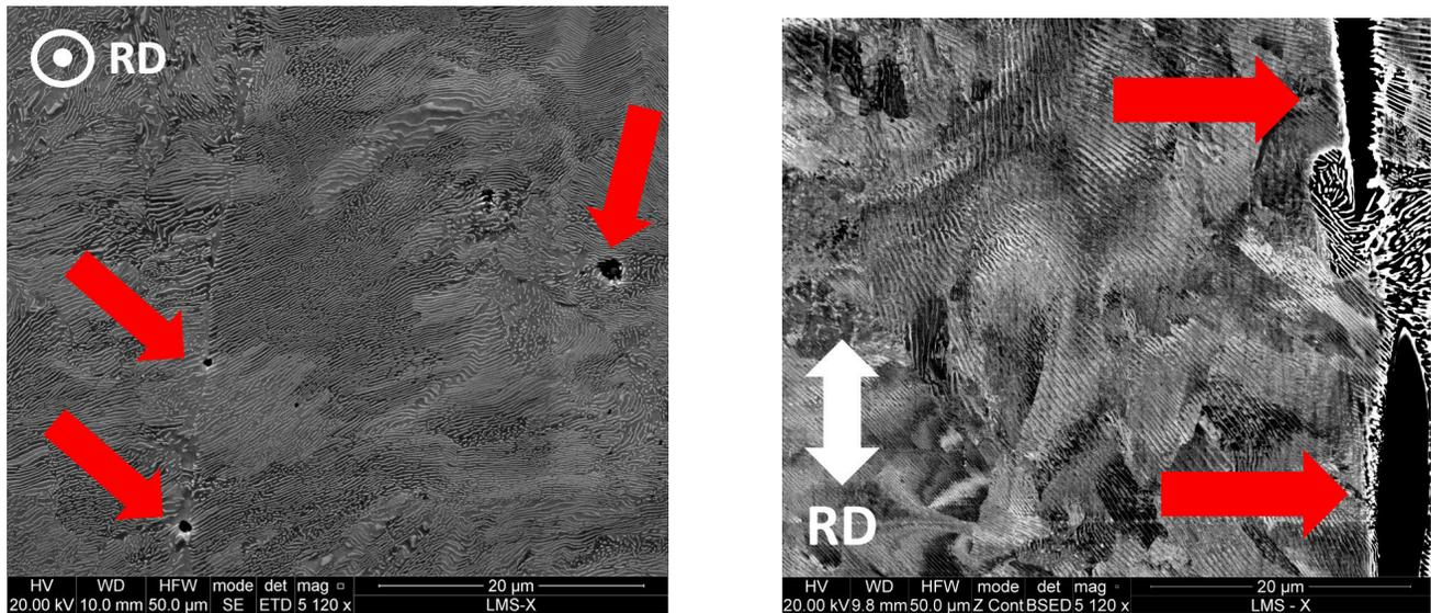
Figure 3.2: SEM observations of the lamellar structure in the plane orthogonal to the rolling direction *RD* (left), and in a plane containing the rolling direction (right). The red arrows point towards manganese sulfide inclusions.
