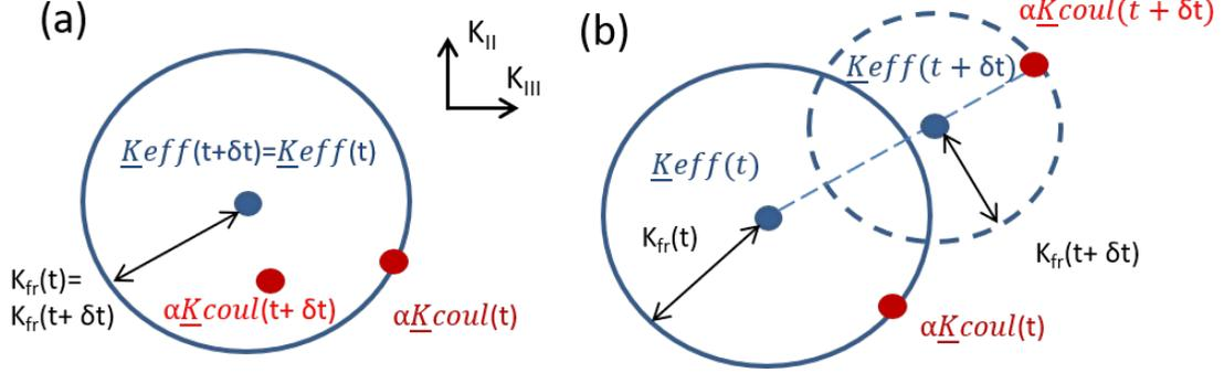
Figure 7.3: Illustration of the evolution of  $\underline{K}^{eff}(t)$  (SIFs in the  $K_{II} - K_{III}$  space) using eq. 7.8. (a):  $\|\alpha\underline{K}^{Coul}(t+1) - \underline{K}^{eff}(t)\| < K_{fr}(t+1)$ , and (b):  $\|\alpha\underline{K}^{Coul}(t+1) - \underline{K}^{eff}(t)\| > K_{fr}(t+1)$
