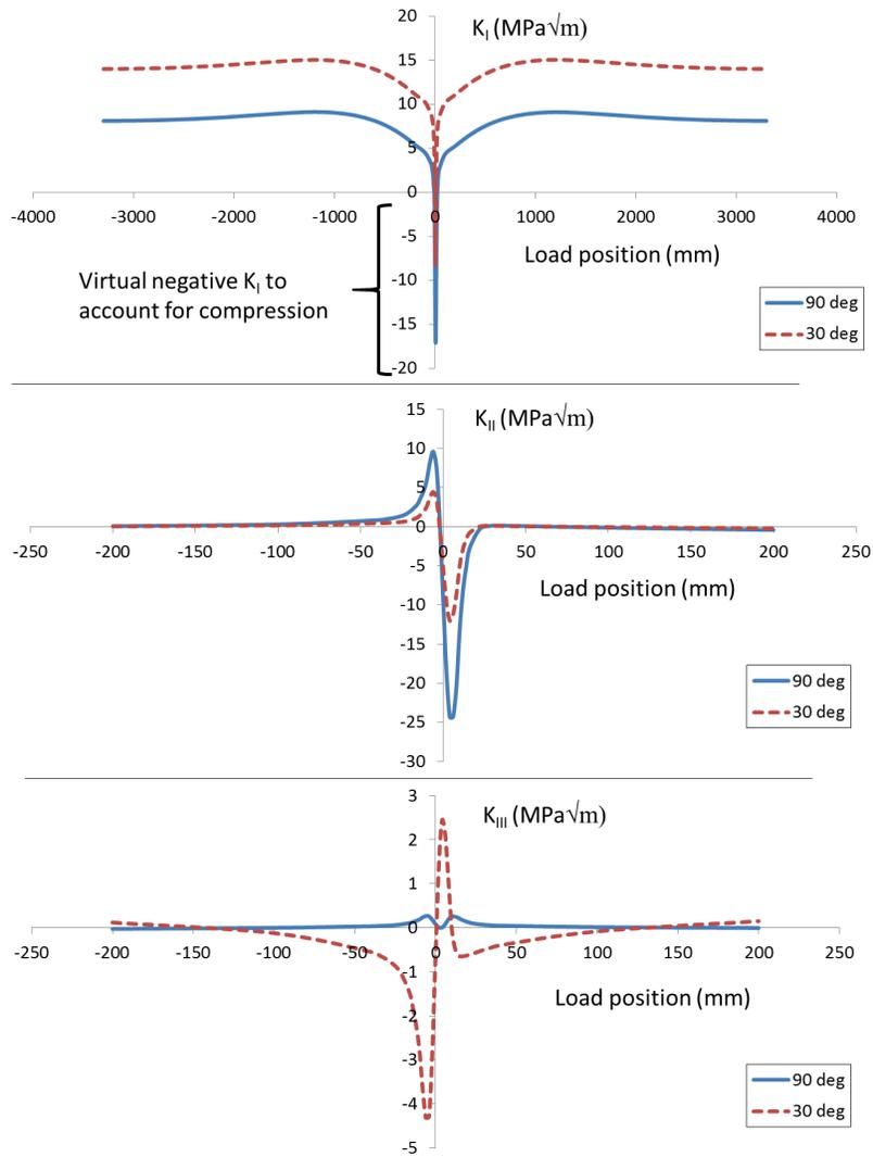
Figure 2.14: Evolution of the SIFs on two points at  $30^\circ$  and  $90^\circ$  on the crack front (see on fig. 2.13) versus the load position. TGV motor load ( $8.5 \text{ kN}$ ).  $30 \text{ MPa}$  longitudinal thermal stresses, corresponding to a  $5^\circ$  temperature. No friction between the crack faces. Residual stresses taken into account.
