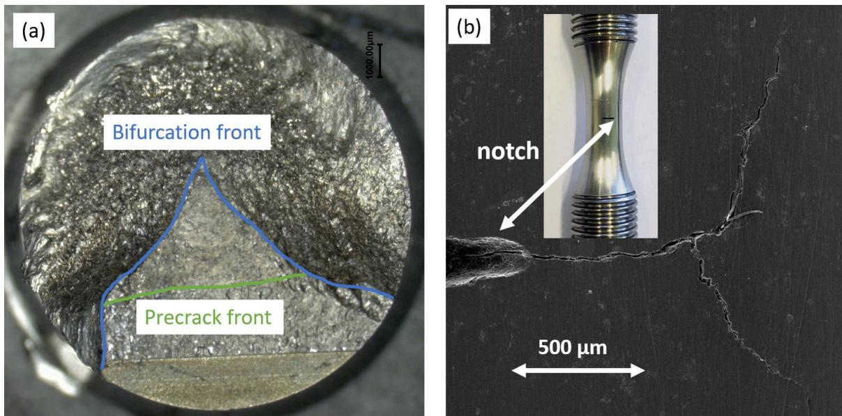
Figure 7.8: Precrack and final crack front of sequential mixed-mode I + II & III test  $N^{\circ}3$  ( $F = 17/0 \text{ kN}$ ,  $C = 66/-62 \text{ Nm}$ ) (a), along with a side surface view of the bifurcation (obtained by SEM observation of a casted replica) (b).
