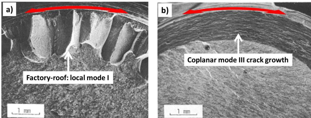
Figure 2.23: Factory roof type fracture surface (low  $\Delta K_{III}$ ) (a) and coplanar (high  $\Delta K_{III}$ ) (b) crack growth during a mode III experiment from [Tschegg, 1983b]. Loading direction indicated by the red arrow.
