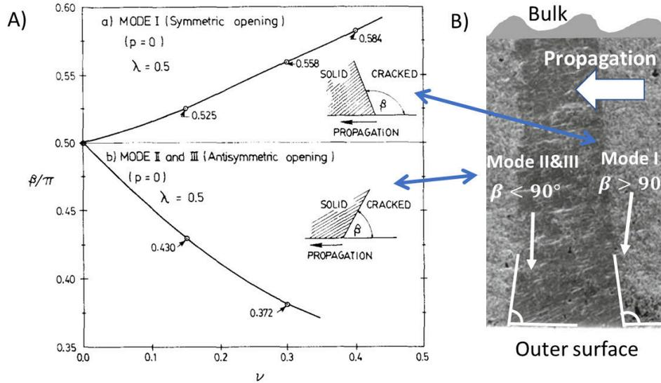
Figure 2.11: A) Evolution of the emergence angle leading to  $\lambda = 0.5$  in mode I and mode II & III with the Poisson's ratio from [Bazant and Estenssoro, 1979]. B) Fracture surface after mode I precracking followed by mode II & III experiment from [Doquet et al., 2010a].
