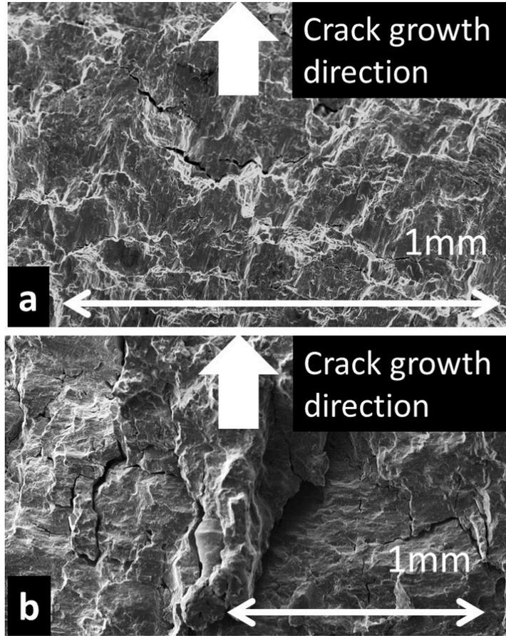
Figure 5.9: Secondary cracks on the fracture surfaces: a) nearly normal to the local crack growth direction where mode *II* dominates and b) nearly parallel to the local crack growth direction where mode *III* dominates.
