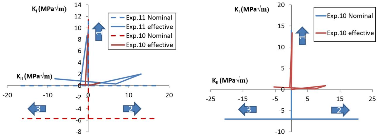
Figure 6.30: Nominal and effective loading paths for sequential experiment  $N^\circ 10$ &11 ( $F = +11/-5$  &  $+11/0$  kN,  $C = \pm 160$  Nm), a) at cycle 2000 for both experiments (similar crack lengths), and b) test  $N^\circ 10$  at cycle 11000.
