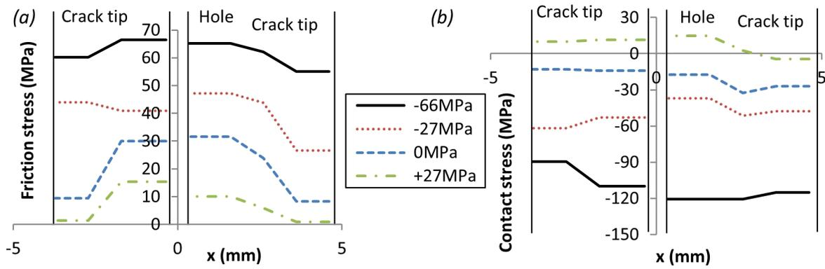
Figure 3.29: Estimated friction stress profile at fixed  $\Delta\tau = 115 \text{ MPa}$  with various static tensile or compressive loads (a). Estimated contact stress profile in mode I at fixed  $\sigma_{max} (133 \text{ MPa})$  for various  $\sigma_{min}$  (b)
