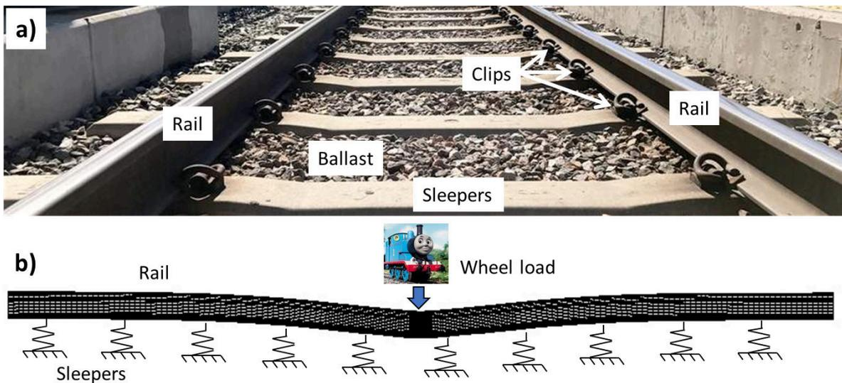
Figure 1.3: Track nomenclature (a). Equivalent Mechanical model (b).
