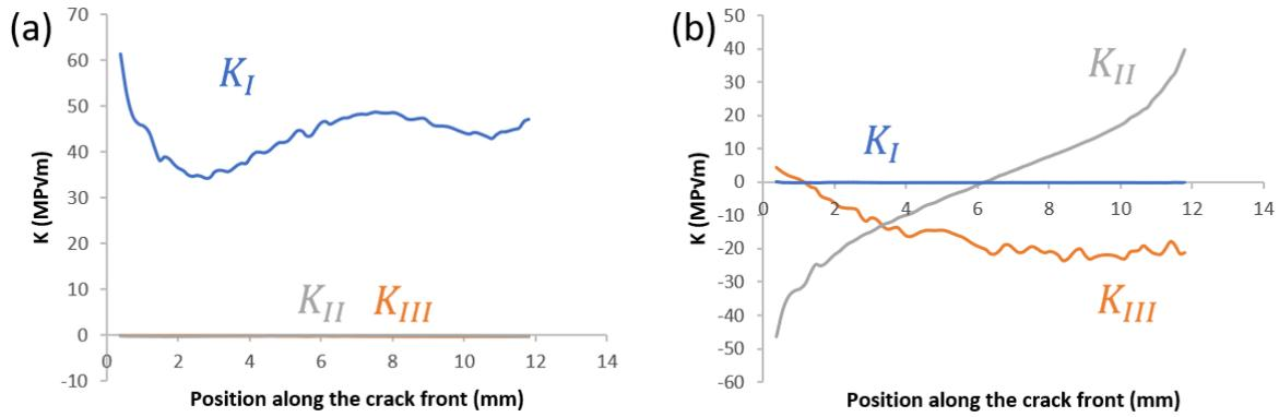
Figure 7.12: Evolution of the SIFs along the final crack front a) at peak tensile load and b) at maximum torque for the sequential mixed-mode I + II & III test  $N^\circ 1$ , for a 17  $kN$  tensile load, and a 35  $Nm$  torque.
