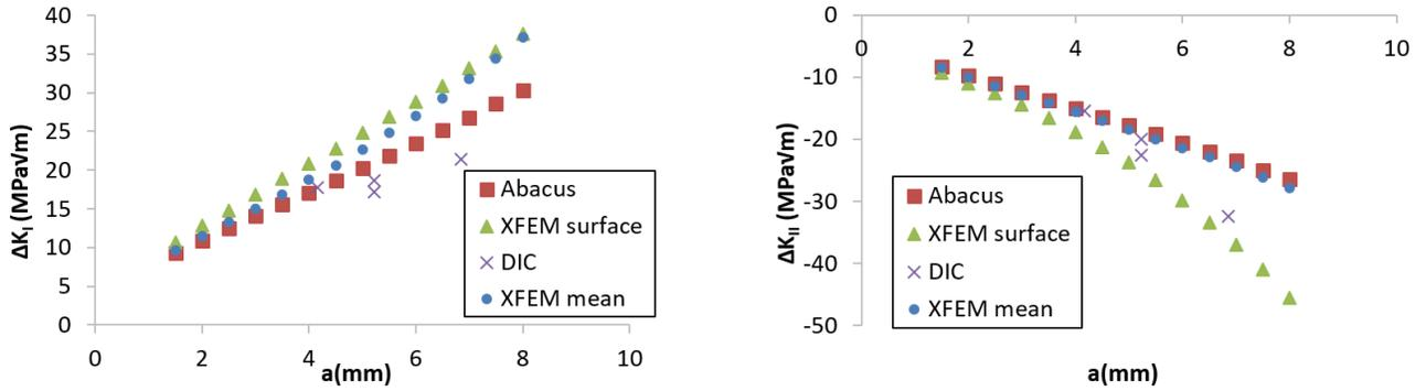
Figure 6.9: Left:  $K_I^{nom}$  estimated using DIC, Erdogan's abacus, and XFEM computations (mean and 50  $\mu\text{m}$  from the outer surface value on the crack front) for a tensile load, as a function of the crack length. Right:  $K_{II}^{nom}$  estimated using DIC, Erdogan's abacus, and XFEM computations for a shear load, as a function of the crack length.
