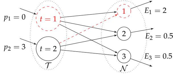
FIGURE 1.1: Example of a flow representation of the disaggregation problem ( $T = 2$  and  $N = 3$ ,  $\underline{x} = 0$ ,  $\bar{x} = 1$ ). Here, the aggregate constraints (1.6) are verified, but condition (1.7) written with  $\mathcal{A} = \{t_1, n_1\}$  (dashed nodes) does not hold.
