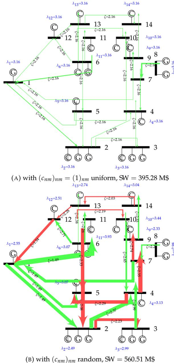
FIGURE 7.6: Trades [\$/MWh] at the VNE of the IEEE 14-bus network with homogeneous differentiation prices (left) and heterogeneous differentiation prices (right). With heterogeneous prices, the quantities traded are larger, and some links become congested. In the homogenous case, marginal trade prices  $(\zeta_{nm})_{n,m}$  are all equal. In the case of heterogeneous prices  $(c_{nm})_{nm}$ , marginal prices  $(\zeta_{nm})_{n,m}$  are also heterogeneous.
