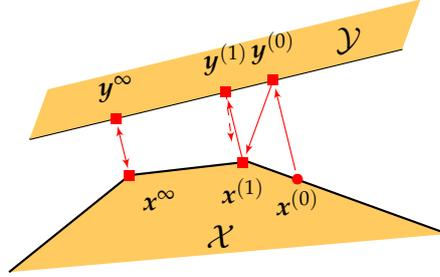
FIGURE 1.2: Alternate projections method (APM) on two sets  $\mathcal{X}$  and  $\mathcal{Y}$ . When  $\mathcal{X} \cap \mathcal{Y} = \emptyset$ , APM cycles over two points  $\mathbf{x}^\infty$  and  $\mathbf{y}^\infty$ .
