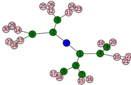
FIGURE 7.1: Example of a radial network. The root node at the interface of the distribution and transmission networks, can trade energy with any other node in the distribution network. In the distribution network, prosumer nodes organize in local energy communities, trading energy with neighbors inside their local community.
