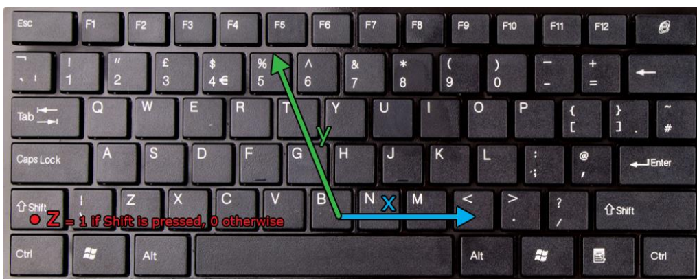
Figure 3.2: Keyboard coordinate system, starting at the bottom left. The string "Arc" has coordinates ((1, 1, 1), (4, 2, 0), (3, 0, 0)) .
