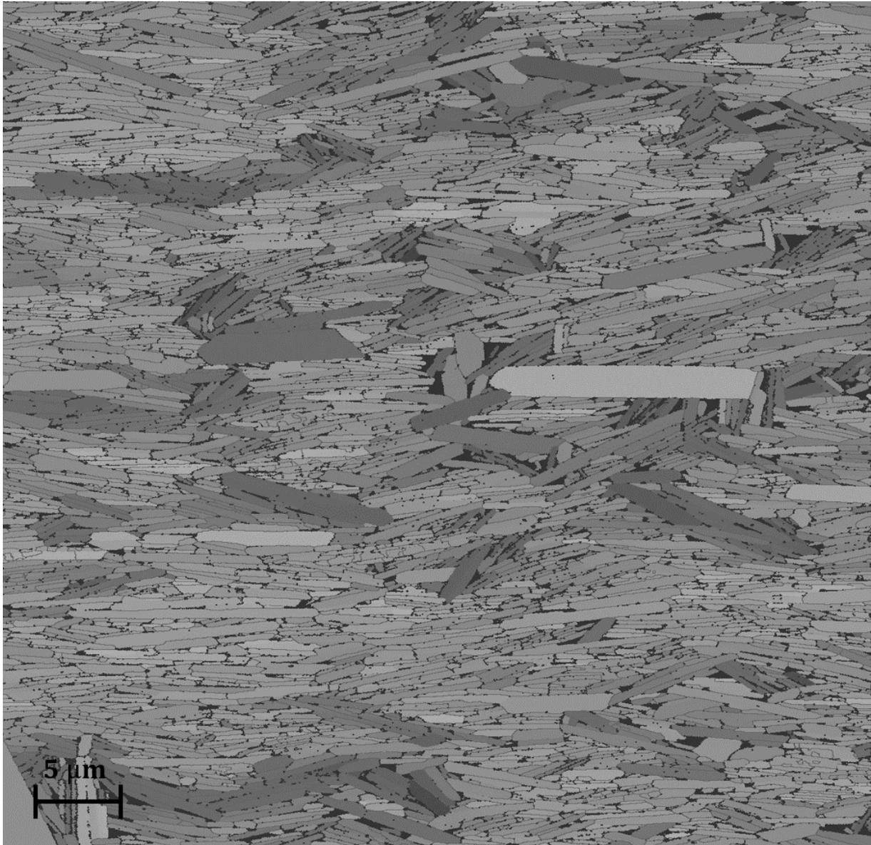
Figure 5.13: EBSD analysis of the sample (Index quality map). The image here is rotated compared to the previous figure.
