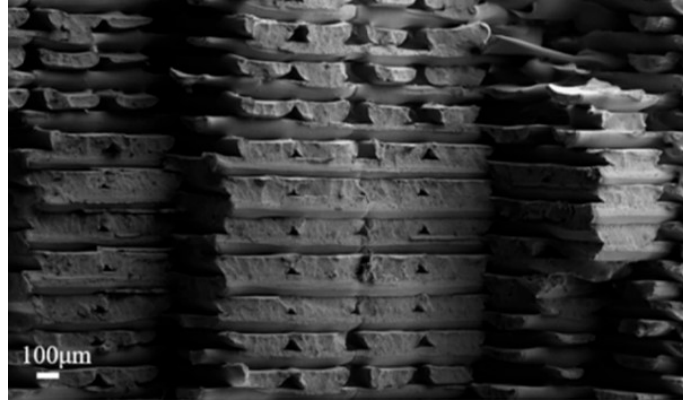
Figure 2.8: A SEM micrograph of a printed nacre produced by Yadav et al. using 3D printing method [Yadav et al., 2018].
