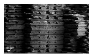
Figure 2.8: A SEM micrograph of a printed nacre produced by Yadav et al. using 3D printing method [Yadav et al., 2018].
