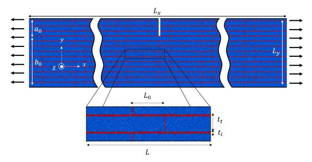
Figure 4.1: Overview of a notched microstructure with staggered tablets (in blue) showing geometry, dimensions ( $L_x = 57 \,\mu\text{m}$ ,  $L_y = 9 \,\mu\text{m}$ ), and loading. Similar unnnotched samples are used for strength determination. Only half of the volume used in our simulations is represented here. A close-up view shows a representative volume element together with characteristic structural parameters.
