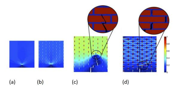
Figure 2.20: : Longitudinal strain fields of the brick and mortar system, (a) bulk material, (b) with a stiffness ratio  $E_i/E_t = 0.64$ , (c)  $E_i/E_t = 0.44$ , (d)  $E_i/E_t = 0.02$ . The interface absorbs the increasing portion of strain as the stiffness ratio decreases which occurs along with a delocalization of stress and strain from the crack tip. c) Shows a clear transition in the fracture mode (from interface to tablet). Figures are reproduced from [Dimas & Buehler, 2013].
