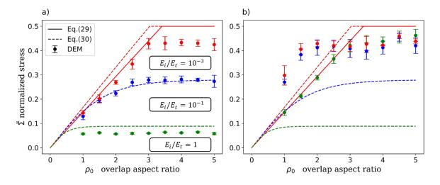
Figure 3.11: Normalized macroscopic stress  $\tilde{\Sigma} = \frac{\Sigma}{\Sigma_t}$  of the RVE as a function of  $\rho_0$  for three different stiffness ratios  $\frac{E_i}{E_t}$  compared to analytical models [Ni et al., 2015; Barthelat, 2014]. (a) Fracture initiation stress  $\Sigma_{init}$  and (b) Maximum stress  $\Sigma_{max}$  after crack propagation. Eq. (3.29) is only valid for small elastic modulus ratios for which it is very similar to Eq. (3.30).
