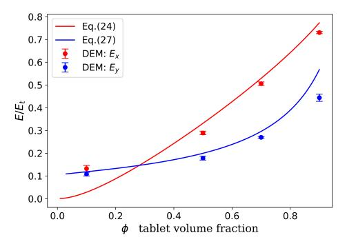
Figure 3.9: Normalized analytical Young's modulus  $\tilde{E}_x$  and  $\tilde{E}_y$  (Eqs. (3.26) and (3.27) against the tablet volume fraction  $\phi$  with an aspect ratio  $\rho = 20$  compared to the DEM results (bullet symbols). The error bars are computed based on five simulations.
