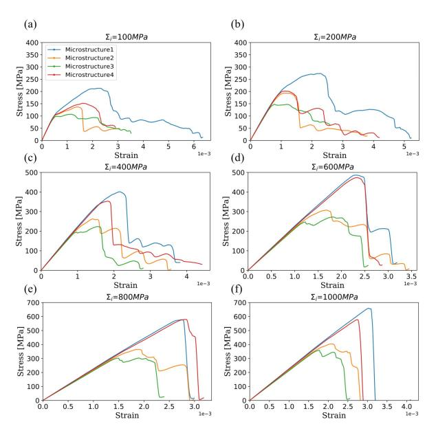
Figure 5.20: Stress-strain plots of single edge notched samples for different interface strength values. a)  $\Sigma_i = \frac{1}{40} \Sigma_t$ , b)  $\Sigma_i = \frac{1}{20} \Sigma_t$ , c)  $\Sigma_i = \frac{1}{10} \Sigma_t$ , d)  $\Sigma_i = \frac{1}{7} \Sigma_t$ , e)  $\Sigma_i = \frac{1}{5} \Sigma_t$ , f)  $\Sigma_i = \frac{1}{5} \Sigma_t$ .
