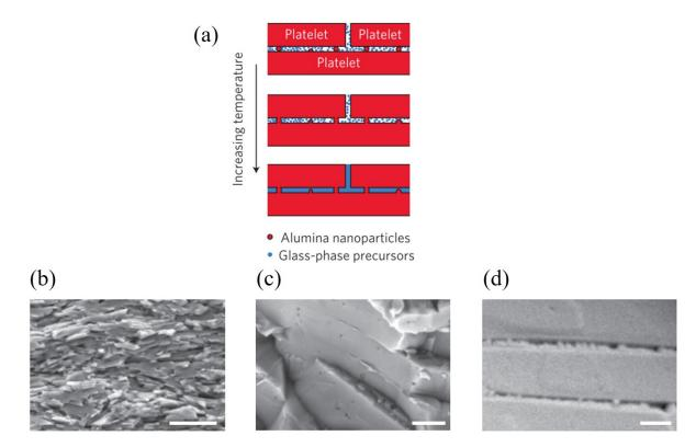
Figure 1.1: Nacre-like alumina. a) A simple scheme with the components of the material. b,c, d) SEM images showing the brick and mortar structure on different scales (scale bars 10 10 µm (b), 500 nm (c) and 250 nm (d) [Bouville et al., 2014b].
