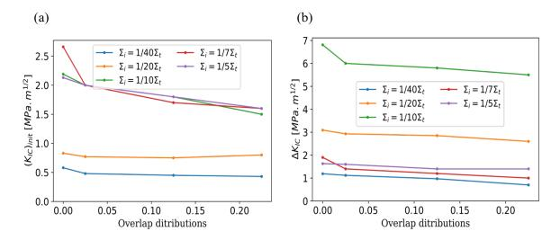
Figure 5.10: Toughness of samples versus overlap aspect ratio distributions for different interface strength values. a) Initiation toughness  $(K_{Ic})_{init}$  and b) crack growth toughness  $\Delta K_{Ic}$  as a function of the interface strength.
