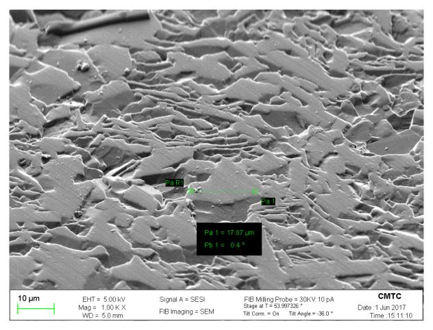
Figure C.2: FIB-SEM milling in the coated region.
