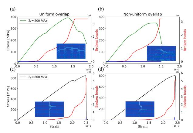
Figure 5.8: Comparison of the samples' final shape after failure for uniform and non-uniform distributions. Both cases of failure are captured here, a,b) stable crack propagation or non-catastrophic failure (green curves), and c,d) catastrophic failure (black curves). Stress-strain curves are plotted along the number of broken bonds in the interface (red curves) and the tablets (blue curves).
