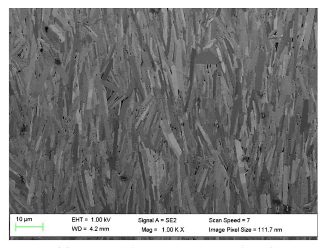
Figure 5.12: A SEM micrograph of the obtained microstructure after the final polishing and before EBSD analysis.
