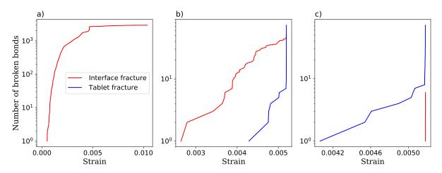
Figure 3.13: Number of broken bonds versus strain for both interface and tablet, where red and blue curves represent the interface and the tablet bonds, respectively. (a) Interface fracture initiation and propagation (b) Interface fracture initiation and tablet fracture propagation (c) Tablet fracture initiation and propagation.
