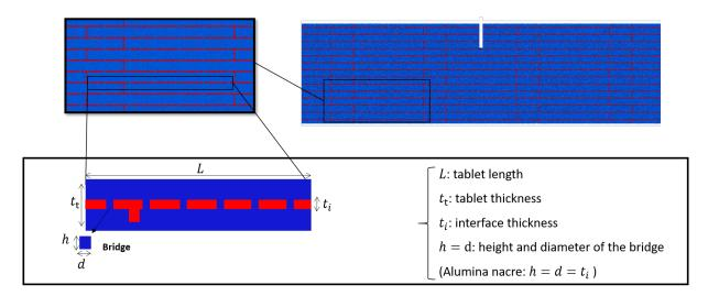
Figure A.4: A notched sample with nano-bridges (in blue) connecting two tablets through the interface. A zoom-in shows the distribution and geometry of nano-bridges. Nano-bridges are introduced both at horizontal and vertical interfaces.
