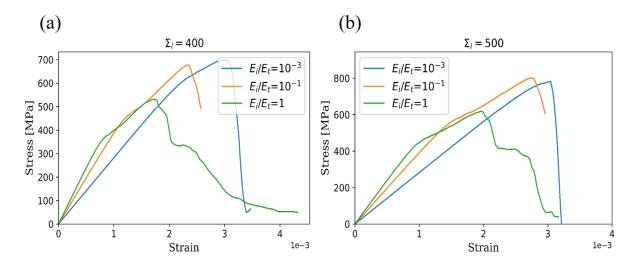
Figure B.2: Stress-strain curves of the three modulus ratios for  $\Sigma_i = \frac{1}{10}\Sigma_t = 400$  MPa and  $\Sigma_i = \frac{1}{8}\Sigma_t = 500$  MPa.
