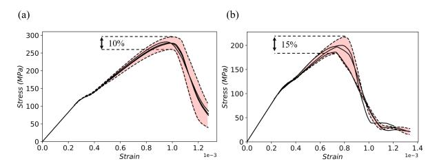
Figure 5.3: Stress-strain curves a given overlap ratio distribution  $\frac{\Delta \rho_0}{\tilde{\rho_0}} = 0.025$  showing the dispersion for both a) unnotched and b) notched samples. 5 simulations are reported with plain curves. Dotted curves are mean a) +/- 5% b) +/- 7.5%.
