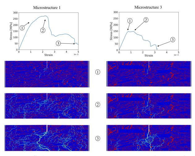
Figure 5.21: Crack propagation illustration in microstructures 1 and 3 for a low interface strength ( $\Sigma_i = \frac{1}{20} \ \Sigma_t = 200 \ \text{MPa}$ ). Stress-strain curves and snapshots of the three main events during SENT (1) damage initiation, (2) maximum stress and (3) material failure.
