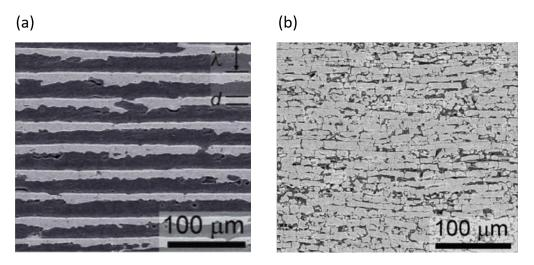
Figure 2.5: a) A SEM image of lamellar structure  $Al_2O_3 - PMMA$  produced by freeze casting by Munch et al. , the lighter phase is the ceramic and the darker one is the polymer. b) Brick and mortar structure issued from pressing and sintering the lamellar scaffolds [Munch et al., 2008].
