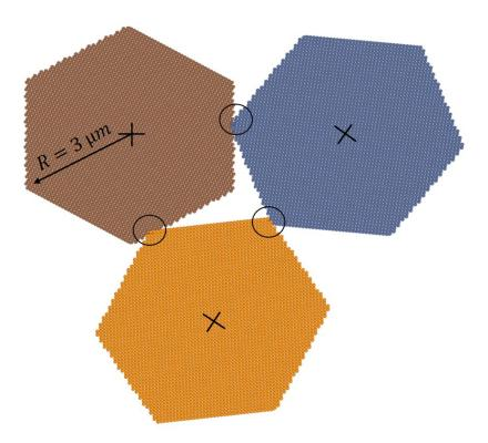
Figure 6.3: A scheme of three clumps interacting through three contacts (black circles). Here the interactions are not calculated inside the clumps. Instead, the total forces and moments are calculated at the center of gravity of the clumps (black cross).
