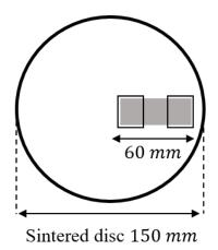
Figure 5.11: Top view of the sintered alumina-nacre disc and the spatial location of the samples.
