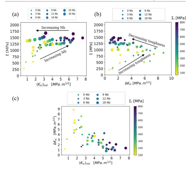
Figure 4.9: Property maps showing the different possible combinations of strength and toughness by variation of either the interface strength or the addition of nano-bridges at the interface. a) crack initiation toughness, b) Crack growth toughness versus crack initiation toughness.
