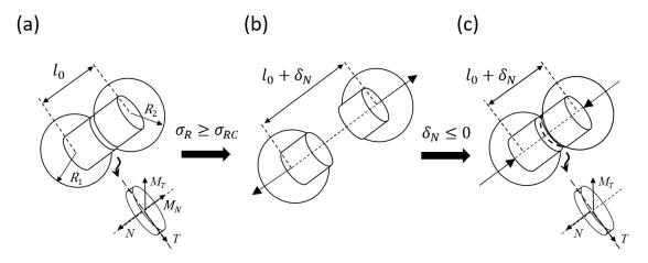
Figure A.2: Two bonded particles transmitting normal/tangential forces and resisting moments with  $l_0$  the initial center to center distance. (a) Unbroken bond. (b) Broken bond. (c) Resumed contact after bond fracture transmitting only compressing forces, friction forces and tangential resisting moment.
