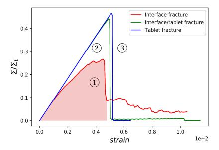
Figure 3.12: Typical stress-strain curves for  $\Sigma_i = 200$  MPa ,1 200 MPa and 4 000 MPa. Three fracture regimes can be identified with increasing interface strengths  $\Sigma_i$ : (1) Interface fracture, (2) Interface/tablet fracture and (3) Tablet fracture.
