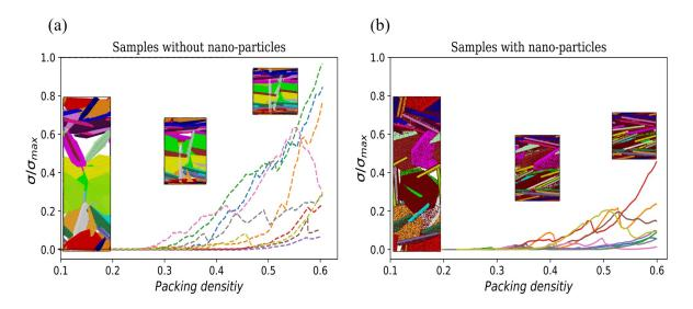
Figure 6.6: Evolution of the normalized axial stress as a function of the packing density for ten simulations for both microstructure types a) without nano-particles and b) with nano-particles. The axial stress is normalized by the maximum stress of the compacted the without nano-particles compacted samples.
