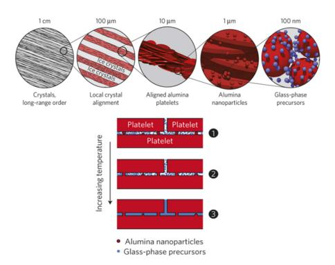
Figure 2.9: A description of the fabrication strategy and structural self-organization in nacre like alumina. Ice crystals grow to trigger the alignment of the alumina tablets, then the nano-particles and the glass precursors get trapped between the tablets. Figures are reproduced from [Bouville et al., 2014b].
