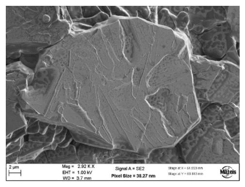
Figure 6.2: SEM micrograph of nacre-like alumina showing the hexagonal shape of an individual tablet. Courtesy of LSFC laboratory.
