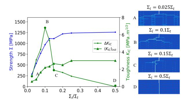
Figure 4.5: Strength, crack initiation toughness, and crack growth toughness for different interface strengths with the crack propagation snapshots.  $\Sigma_i = \frac{1}{10}\Sigma_t$  sample exhibits the largest improvement in both strength and toughness.
