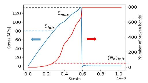
Figure 3.10: Typical stress-strain curve number of broken bonds from a DEM simulation for  $\rho_0 = 2.5$  and  $\frac{E_i}{E_t} = 0.1$ . Two stresses are considered for comparison with analytical models. The fracture initiation stress  $\Sigma_{init}$  corresponds to the stress at which 50 bonds have broken. The strength  $\Sigma_{max}$  corresponds simply to the maximum axial stress.
