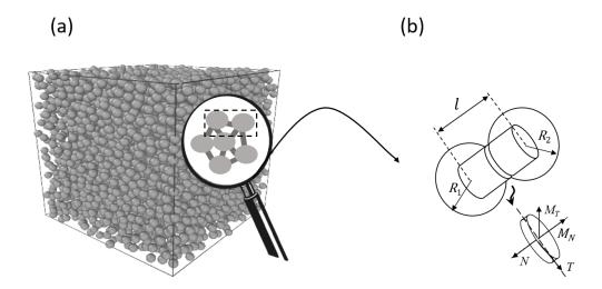
Figure A.1: From macroscopic to microscopic scale. (a) Random packing of bonded particles representing a continuous material. (b) Two bonded particles of radius  $R_1$  and  $R_2$  transmitting normal/tangential forces and resisting moments.
