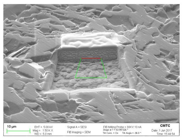
Figure C.3: The final FIB-SEM milling. The BM structure is not distinguishable.
