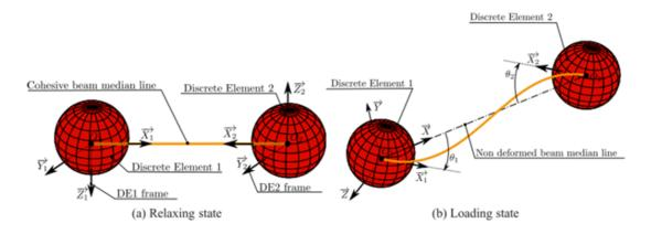
Figure 2.25: Cohesive bond beam configuration: The cohesive beam is represented by its median line. Both cohesive bond ends are fixed to the discrete element centers  $O_1$  and  $O_2$ . Before and after loading states are presented. Figure is adapted from [André et al., 2012].
