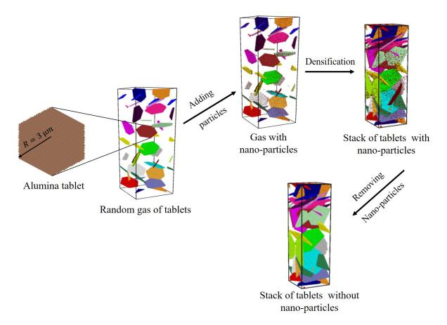
Figure 6.4: Typical evolution of numerical 3D samples with 20 tablets during the preparation stage. The initial gas of tablets has no contact between tablets and an initial density of 0.032. Nano-particles are added and the gas is then densified to obtain a packing of a density of 0.1. The nano-particles are removed to create identical samples but without nano-particles.
