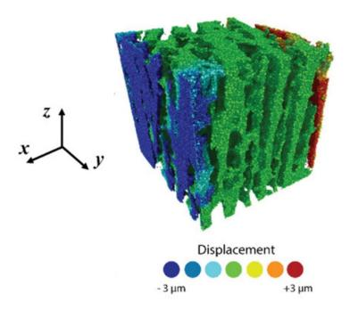
Figure 2.24: Simulation of a longitudinal crushing test of a discrete element packing showing the displacement of particles in the x direction, transverse to the loading axis z. Figures were adapted from [Roussel et al., 2016].
