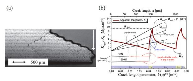
Figure 7.1: Toughness increase in layered ceramics after introducing compressive residual stresses. a) Optical micrographs of the composite bend bars post fracture [Pavlacka et al., 2013]. The arrow indicates the transverse direction b) Stress intensity factor  $(K_{appl})$  and calculated material fracture toughness  $(K_R)$  as a function of the crack length for indented composite [Chang et al., 2014].
