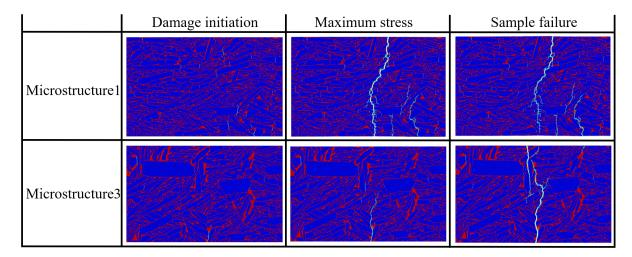
Figure 5.18: Snapshots of the tensile tests performed on microstructure 1 and 3 for a high interface strength ( $\Sigma_i = \frac{1}{4} \Sigma_t$ ).
