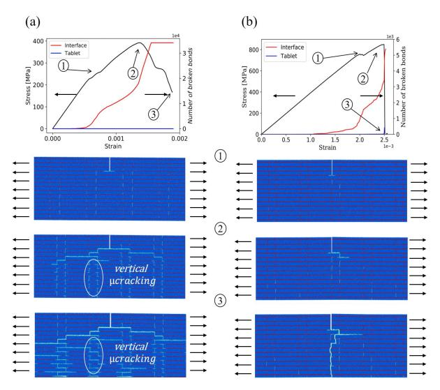
Figure 4.3: Example of a notched sample under uniaxial loading for two different values of interface strength a)  $\Sigma_i = \frac{1}{20} \Sigma_t$  and b)  $\Sigma_i = \frac{1}{5} \Sigma_t$  with tensile stress-strain curves and broken bonds in both interface and tablets. Corresponding sequences of deformation show (1) damage initiation, (2) maximum stress and (3) material failure.
