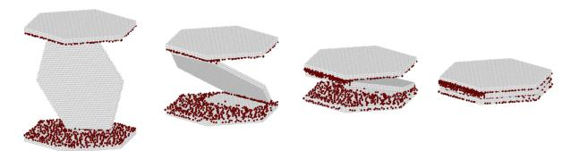
Figure 6.7: Snapshots of a sandwiched tablet under uniaxial compaction between two tablets. Progressively nanoparticles are swept away from the surface.
