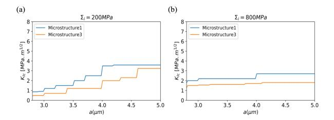
Figure 5.24: Toughness versus crack extension (R-curve) of microstructure1 and 3. a) Low interface strength ( $\Sigma_i = \frac{1}{20} \Sigma_t$ ), b) High interface strength ( $\Sigma_i = \frac{1}{5} \Sigma_t$ ).
