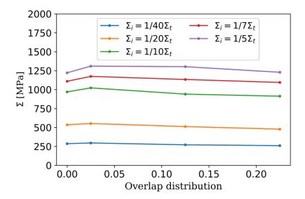
Figure 5.6: Strength versus overlap distributions of the different interface strength values.
