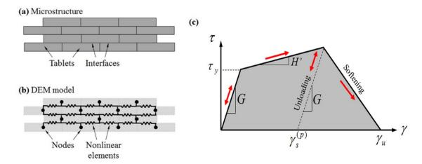
Figure 2.22: (a) A 14 tablet model and (b) corresponding DEM model with rigid tablets and a nonlinear spring at each interface. Tablets and their interfaces are represented by nodes and nonlinear elements respectively. (c) Shear stress-strain curve of individual springs. Figures are adapted from [Abid et al., 2018, 2019].
