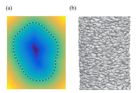
Figure 7.3: a) An example of boundary node discretization with nodes in white seeded on the grain surface. b) A virtual level set function representation of a specimen [Kawamoto et al., 2018].
