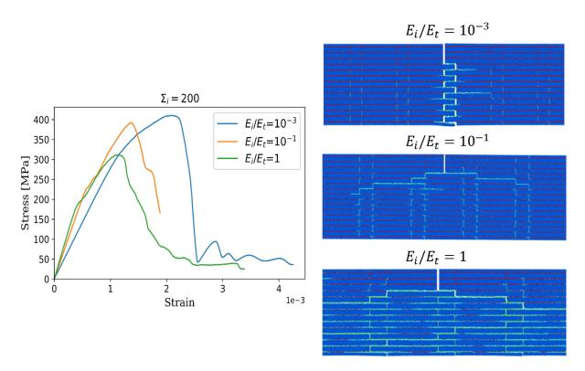
Figure B.1: Stress-strain curves of three notched samples for a given interface strength  $\Sigma_i = \frac{1}{20}\Sigma_t = 200$  MPa and three different interface/tablet Young modulus ratios, and the corresponding snapshots of the final shape of the crack path.
