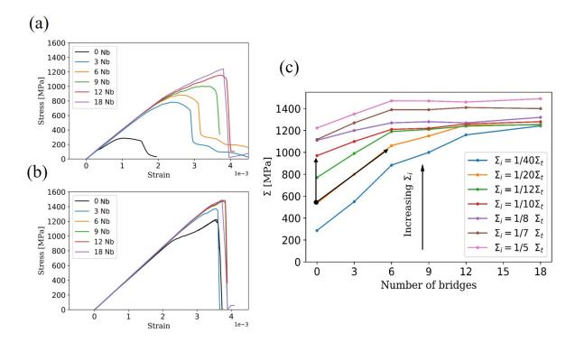
Figure 4.6: Stress-strain response of unnotched samples with various number of bridges per tablet (Nb), for two different interface strengths, a)  $\Sigma_i = \frac{1}{20}\Sigma_t$  and b)  $\Sigma_i = \frac{1}{5}\Sigma_t$ . c) Strength as a function of Nb for increasing interface strengths. The black arrows point to two different paths to obtain the same macroscopic strength either by an increase in  $\Sigma_i$  or the introduction of nano-bridges.
