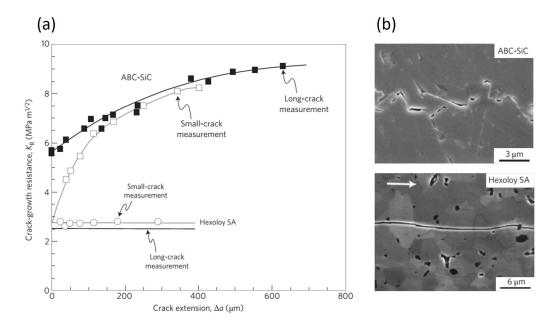
Figure 2.13: : a) An example of a rising crack-resistant curve (R-curve) of ABC/SIC (Silicon carbide, processed with dopants of aluminum, silicon and boron) which can fail intergranulary along the brittle grain-boundary films (extrinsic toughening). b) Commercial SiC hexoloy, fails transgranularly with no extrinsic toughening (no rising R-curve) [Ritchie, 2011].
