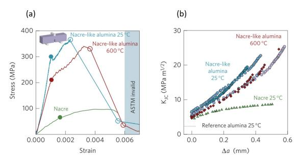
Figure 2.10: Mechanical properties of nacre-like alumina at different temperatures. a) Stress-strain curves. The filled disks show the beginning of stable crack propagation and the circles show the beginning and the end of unstable crack propagation. b) Fracture toughness as a function crack size. Figures are reproduced from [Bouville et al., 2014b].
