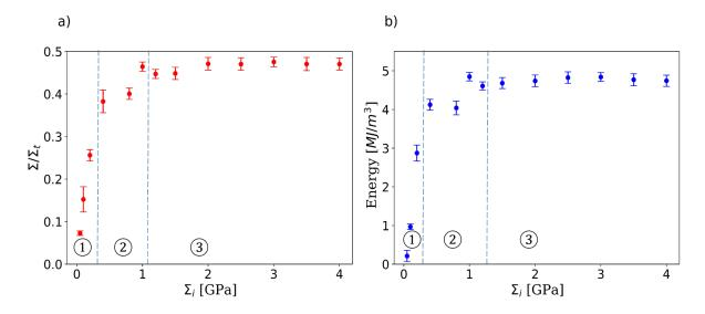
Figure 3.15: (a) Macroscopic strength and (b) fracture energy versus interface strength  $\Sigma_i$ . Standard deviations are calculated from five simulations. Three fracture regimes can be identified with increasing interface strengths  $\Sigma_i$ : (1) Interface fracture, (2) Interface/tablet fracture and (3) Tablet fracture.
