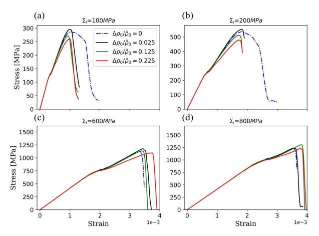
Figure 5.4: Stress-strain plots of the three non-uniform overlap distributions for four different interfaces. All the plots are compared to the uniform overlap distribution tested in the previous chapter  $(\frac{\Delta \rho_0}{\tilde{\rho_0}} = 0)$ .
