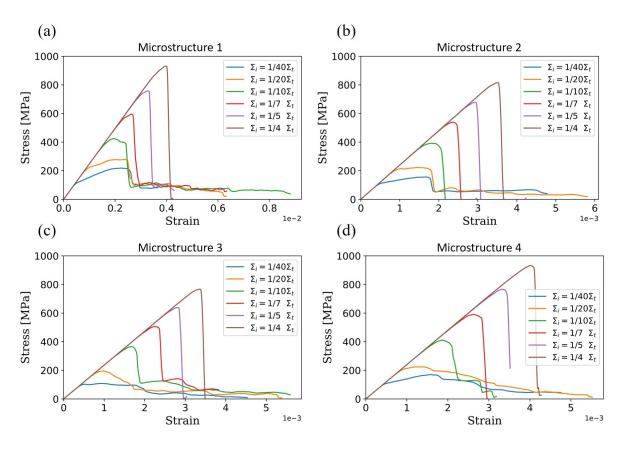
Figure 5.16: Stress-strain curves resulted from tensile tests applied on the four different microstructures.
