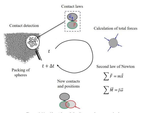
Figure 2.23: Algorithm of the discrete element method
