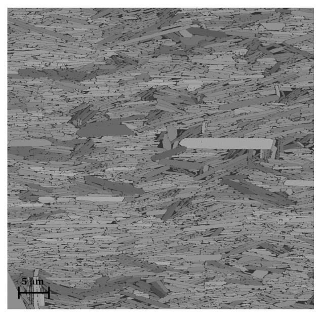
Figure 5.13: EBSD analysis of the sample (Index quality map). The image here is rotated compared to the previous figure.
