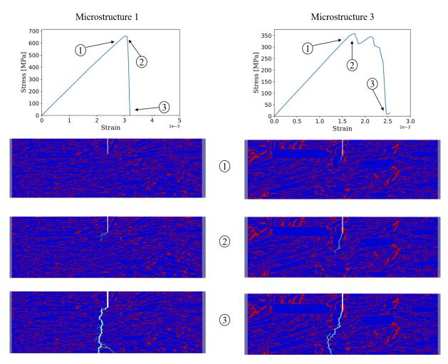
Figure 5.22: Crack propagation illustration in packings 1 and 3 for a high interface strength ( $\Sigma_i = \frac{1}{4} \Sigma_t = 1000 \text{ MPa}$ ). Stress-strain curves and snapshots of the three main events during SENT (1) damage initiation, (2) stress maximum and (3) material failure.
