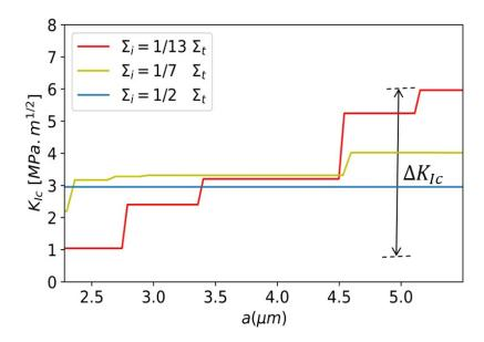
Figure 4.4: Typical crack resistance curves for three interface values representing different behaviors: a rising curve with a staircase pattern for low interface strength, a constant  $K_{Ic}$  value for high interface strength and an intermediate case with moderate increase of  $K_{Ic}$ .
