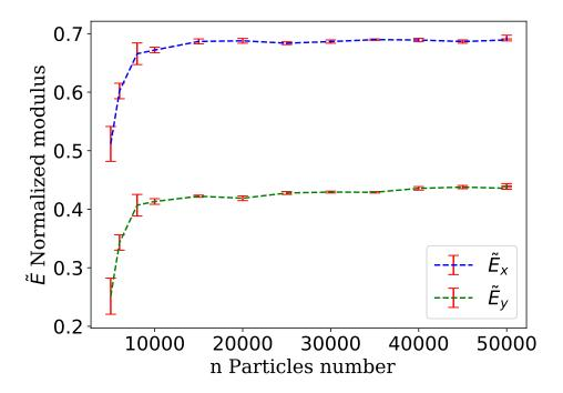
Figure 3.6: Evolution of macroscopic normalized moduli  $\tilde{E}_x$  and  $\tilde{E}_y$  for the RVE shown in Fig. 3.5 against the particle number n for a constant set of microscopic parameters. Sample characteristics: tablet aspect ratio  $\rho = 16$ , overlap ratio k = 0.5, and  $\phi = 0.87$ .
