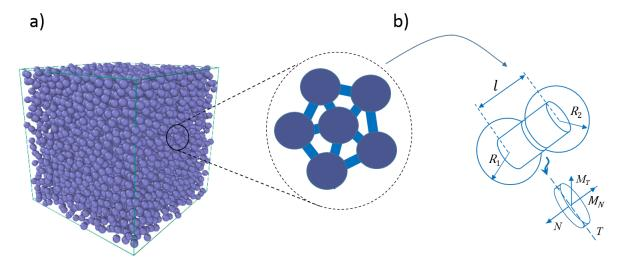
Figure 3.1: From macroscopic to microscopic scale. (a) Random packing of bonded particles representing a continuous material. (b) Two bonded particles of radius  $R_1$  and  $R_2$  transmitting normal/tangential forces and resisting moments.
