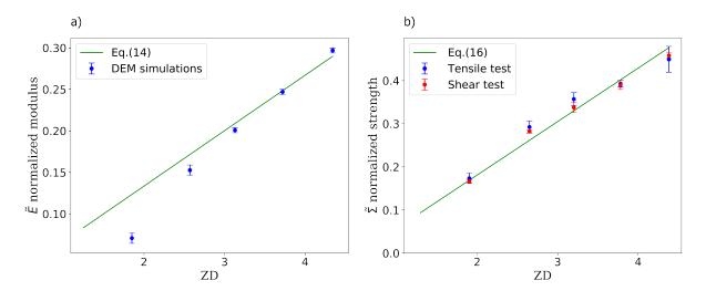
Figure 3.4: Calibration of macroscopic properties of the RVE : (a) Normalized Young's modulus  $\tilde{E} = \frac{E}{\sigma_N}$  and Eq. (3.14). (b) Normalized strength  $\tilde{\Sigma} = \frac{\Sigma}{\sigma_R}$  calibrated in tensile and shear tests.
