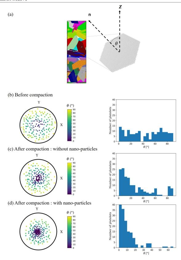
Figure 6.8: a) On of the packings of tablets with a zoom-in on one tablet and the normal vector to it  $\mathbf{n}$ . The angle  $\theta$  between the compaction axis  $\mathbf{z}$  and  $\mathbf{n}$  of each tablet describes its orientation b) before compaction and  $\mathbf{c}$ , d) after compaction for both types of samples.
