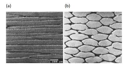
Figure 2.7: Microstructure of  $Si_3N_4$  fibrous monolithic composite Wang et al. [2000a].a) On both sides of the sample, the fibers are arranged regularly in a uniaxial direction. b) A cross section showing the hexagonal shape of the cells.
