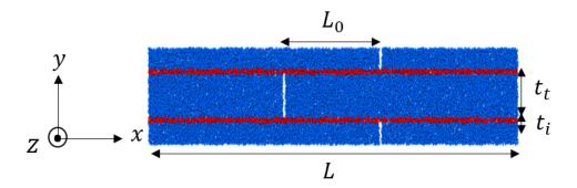
Figure 3.5: Representative Volume Element generated with discrete particles. Red particles mesh interfaces and blue particles mesh tablets. L,  $L_0$ , t and  $t_i$  are geometrical parameters characterizing the RVE.
