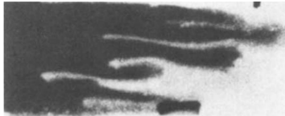
(b) Viscous fingering in an opaque medium visualized by X-ray absorption.
