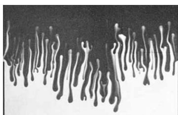
(a) Viscous fingering in a gravity driven miscible displacement in a Hele-Shaw cell.
