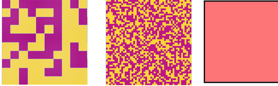
Figure 1.4: Example of a random stationary material: random checkerboard for different values of \varepsilon ( \varepsilon = 1/10 , \varepsilon = 1/50 , \varepsilon \ll 1 , from left to right).
