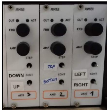
FIGURE C.6: Piezo-motor controller
