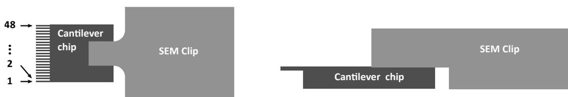
FIGURE C.1: Convention of position of the cantilever chip inside the SEM, and numbering of the cantilevers.
