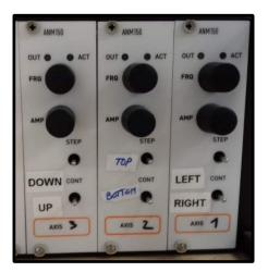
FIGURE C.6: Piezo-motor controller
