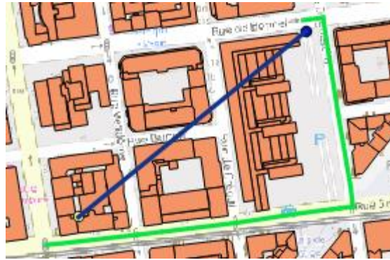
Figure 45 - Euclidian distance vs routable road distance
