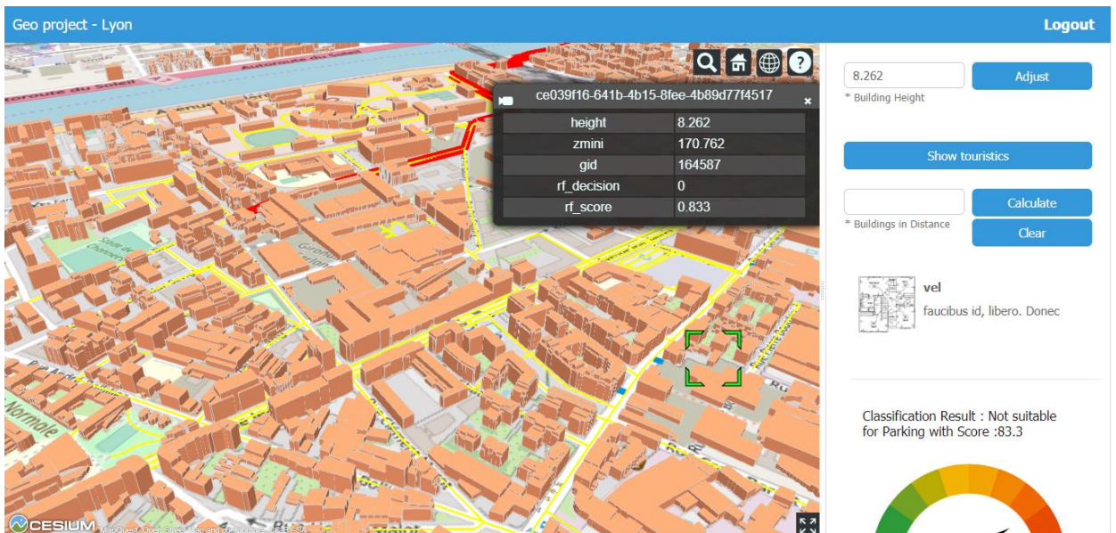
Figure 44 - Building with classification score provided by machine learning techniques
