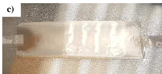
Fig. 1. Illustration of a) “fogging” or b) “slightly fogging” or c) “anti-fogging” surface exposed 1 min to water vapor.
