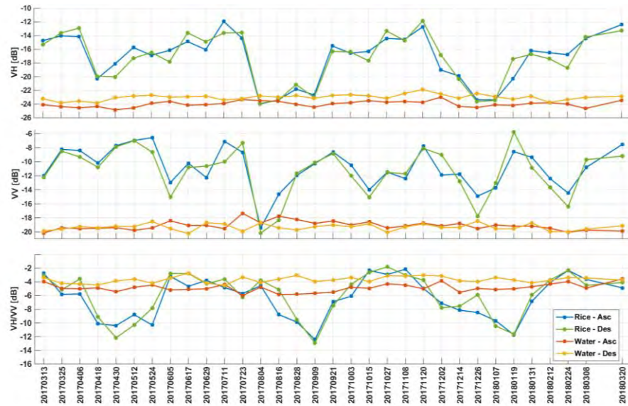
Figure 32. Variation of VH, VV backscattering coefficient, and polarization ratio VH/VV over rice fields and water sample extracted from S1 images at ascending and descending orbits.
