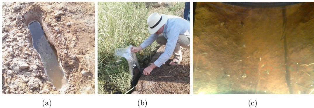
Figure 5.13: (a) An overflooded trench where the wedge can be used; (b) a wedge being used for observing the side of a flooded area; (c) image acquired underwater.
