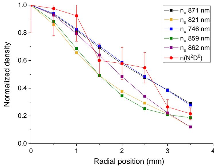
**Figure 106:** Normalized density profiles for the upper states of transitions in the visible/NIR region compared with the density profile of  $N(^2D^0)$  (in equilibrium with N ground state) for the  $N_2/Ar$  HF mixture. These profiles are measured at the exit of the 15-cm tube. The uncertainties are about 35%.
