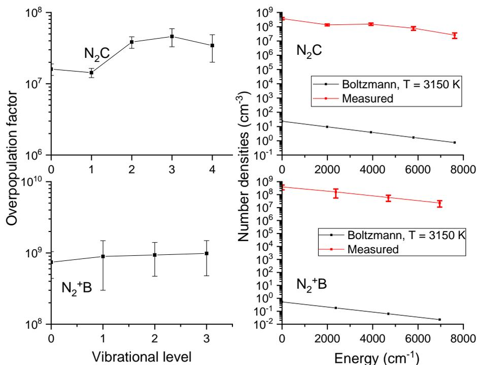
Figure 72: Overpopulation factors (left) for N<sub>2</sub>(C) (top) and N<sub>2</sub><sup>+</sup>(B) resulting from the minimization algorithm and comparison between the measured and equilibrium densities (left).
