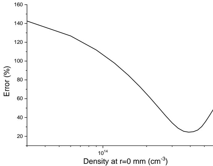
**Figure 119:** Relative error between measured and computed spectra of the 174-nm line at the exit of the 10-cm tube for the N<sub>2</sub>/Ar LF case as a function of the density of the lower state taken in SPECAIR calculations.
