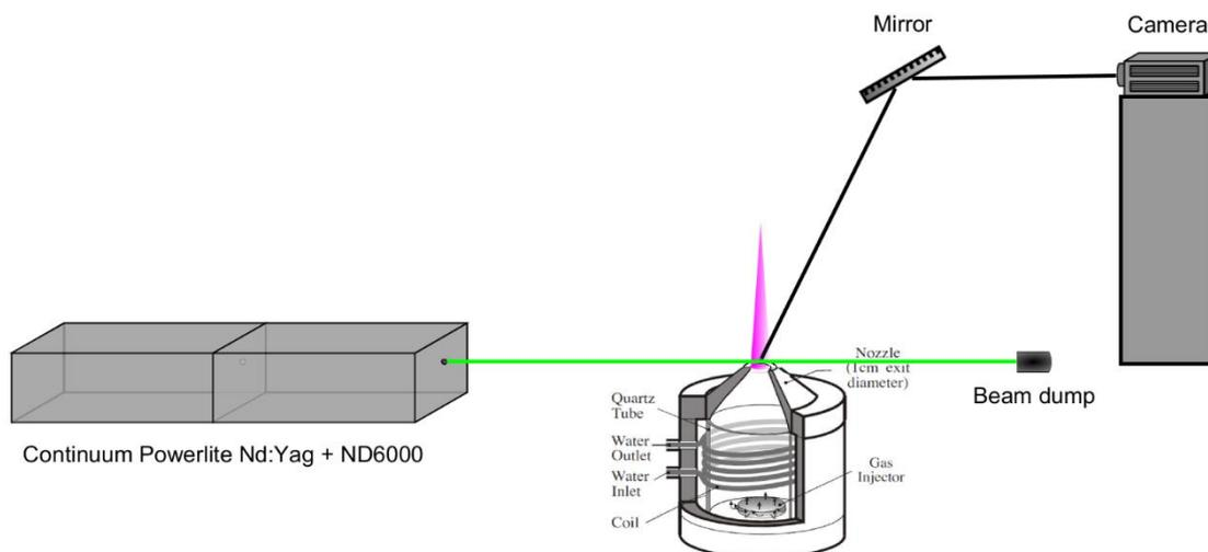
**Figure 38: Experimental setup for beam steering detection**
