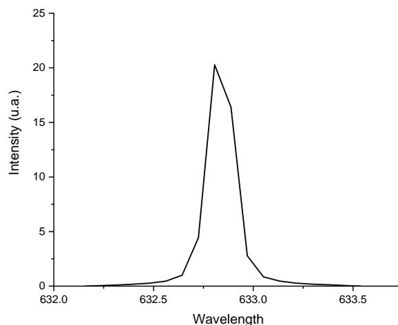
**Figure 75: Slit function measured using a He-Ne laser**
