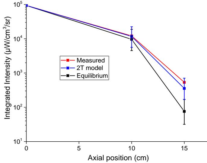
**Figure 86: Integrated intensity between 250 and 900 nm. Red: measurements. Black: computed intensity assuming equilibrium at the measured gas temperature. Blue: computed intensity using the 2-temperature model. N<sub>2</sub>/argon LF.**
