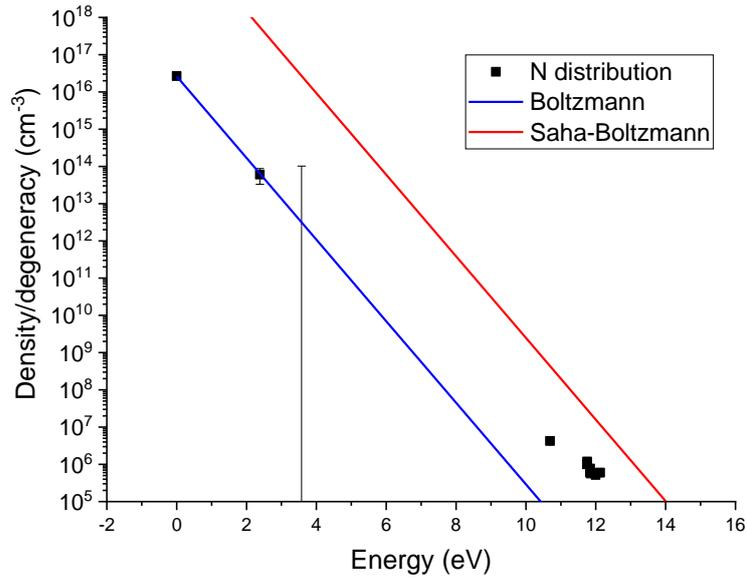
Figure 127: Measured population distribution of ground and excited states of atomic nitrogen (black) at the exit of the 15-cm tube for the  $N_2/Ar$  LF case at  $r = 0$  mm. The Boltzmann (blue) and Saha Boltzmann (red) distributions are also plotted.
