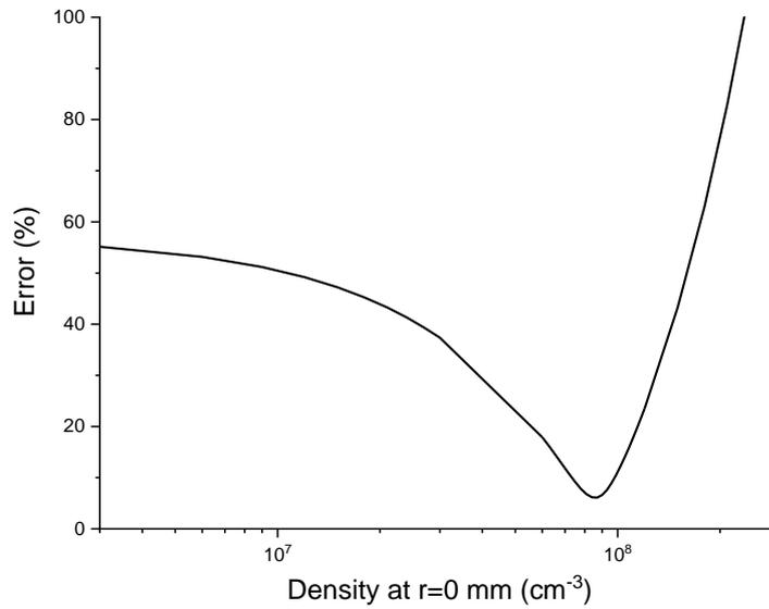
Figure 122. Relative error between measured and computed spectra of the 149-nm line at the exit of the 15-cm tube for the  $N_2/Ar$  LF case as a function of the amplitude of the density of the upper state taken in SPECAIR calculations.
