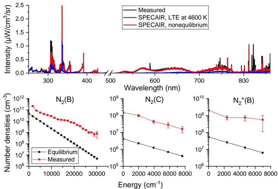
Figure 78. Top: comparison between measured and computed spectra at the exit of the 15-cm tube for the  $\text{N}_2/\text{Ar}$  LF case at the center of the tube ( $r = 0$  cm).
