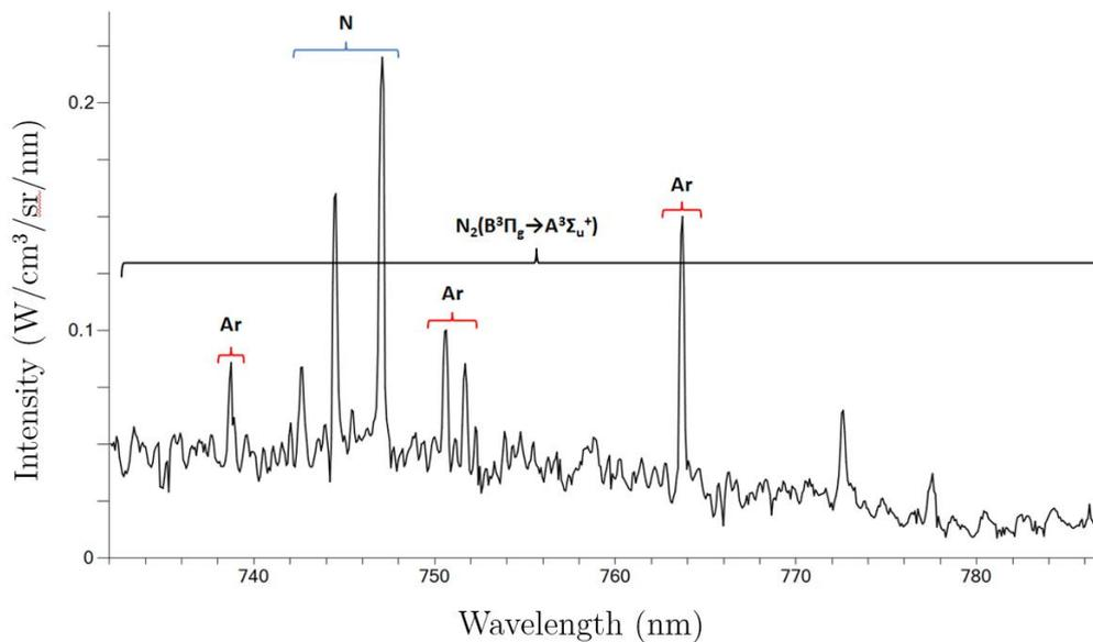
**Figure 18: Abel-inverted emission spectrum of a  $N_2/Ar$  plasma at the exit of the torch. The atomic and molecular transitions are identified.**
