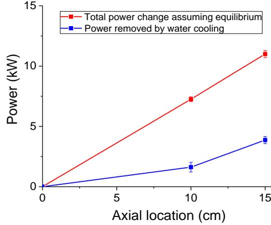
Figure 145: Power measurements for the  $N_2/Ar$  HF case. Blue: measured power removed by water cooling. Red: Power change between the exit and the inlet of the tube assuming equilibrium throughout the tube.
