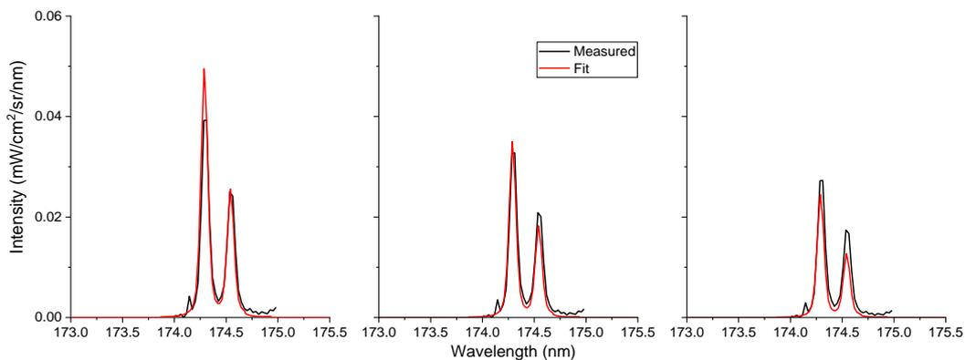
**Figure 138.** 174-nm line: comparison between the measured spectra and the optically thin computed SPECAIR spectra using the measured density profile of the upper state at the exit of the 15-cm tube for the  $N_2/\text{Ar}$  HF case. These three line-of-sight spectra were taken at different lateral positions (0, 1, and 2 mm).
