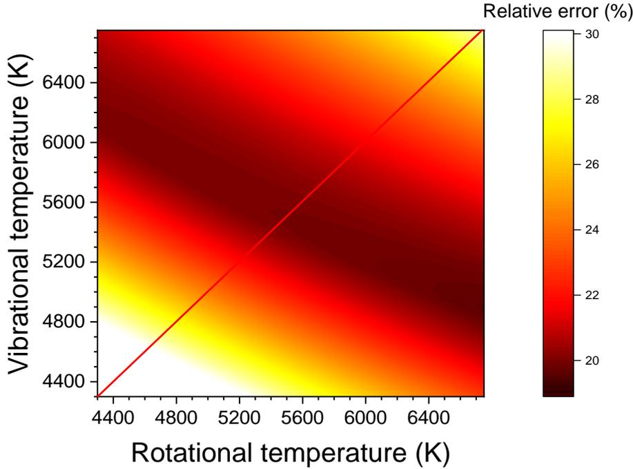
**Figure 26:** Relative error between computed Stokes spectra at  $(T_{rot}, T_{vib})$  and the measured Stokes spectrum. The red line corresponds to  $T_{rot} = T_{vib}$  (equilibrium). Measurements taken in the air plasma, 1 cm downstream of the 5-cm nozzle.
