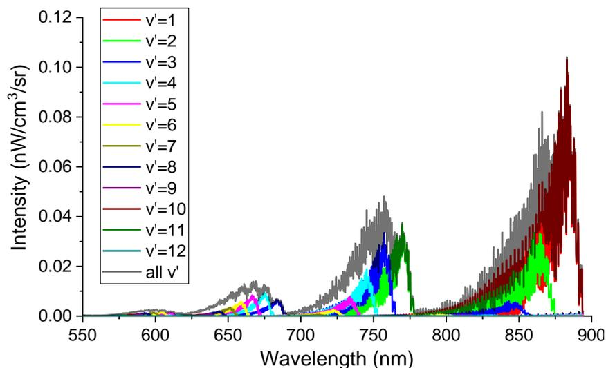
Figure 68: Emission spectra from individual upper vibrational levels, assuming  $T_{\text{rot}} = T_{\text{gas}} = 3200$  K. The cumulative spectrum representing LTE is also plotted in grey. The emission pathlength is 1 cm.
