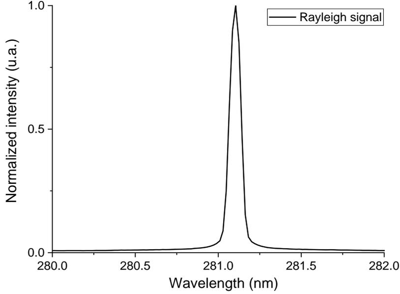
**Figure 25 :** Normalized Rayleigh spectrum obtained for the air case. The slit width was 300  $\mu\text{m}$ . This spectrum was taken in ambient air (300 K, 1 atm). The equivalent FWHM is about 0.15 nm.
