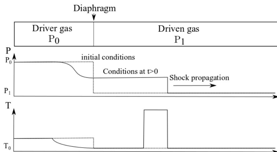
Figure 8: Description of a shock tube facility
