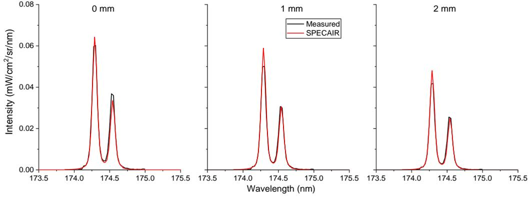
**Figure 125.** 174-nm line: comparison between the measured spectra and the optically thin computed SPECAIR spectra using the measured density profile of the upper state at the exit of the 15-cm tube for the N<sub>2</sub>/Ar LF case. These three line-of-sight spectra were taken at different lateral positions (0, 1, and 2 mm).
