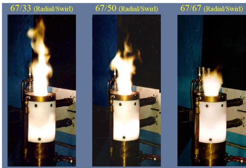
Figure 14: Air plasma plume for three conditions of the radial/swirl flowrates.
