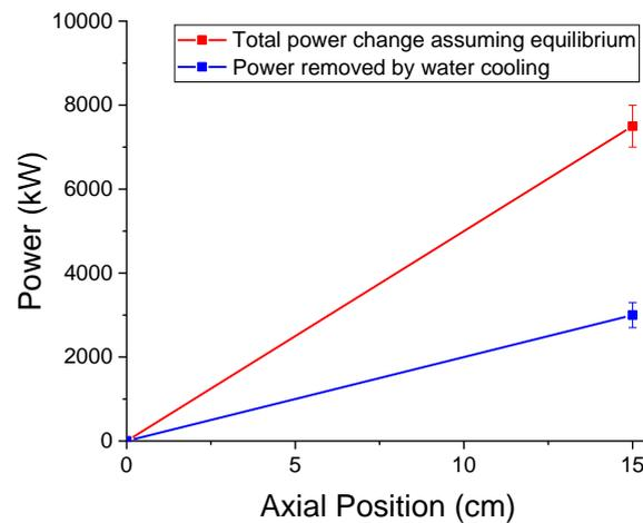
**Figure 144:** Power measurements for the  $N_2/Ar$  LF case. Blue: measured power removed by water cooling. Red: Power change between the exit and the inlet of the tube assuming equilibrium throughout the tube.
