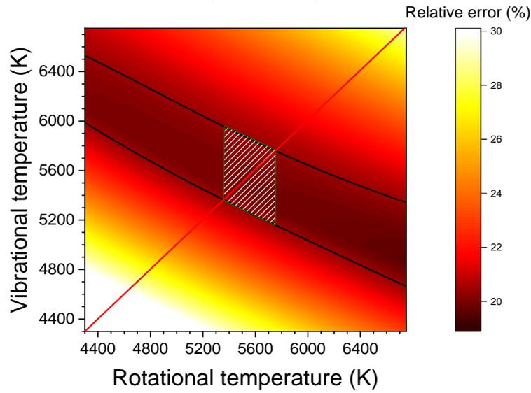
Figure 27: Relative error between the computed Raman spectra at  $(T_{rot}, T_{vib})$  and the measured Stokes spectrum. The black lines define the area where the error is below 21%. The white-hatched region corresponds to the range of acceptable values for  $(T_{rot}, T_{vib})$ . Measurements taken in the air plasma, 1 cm downstream of the 5-cm nozzle.
