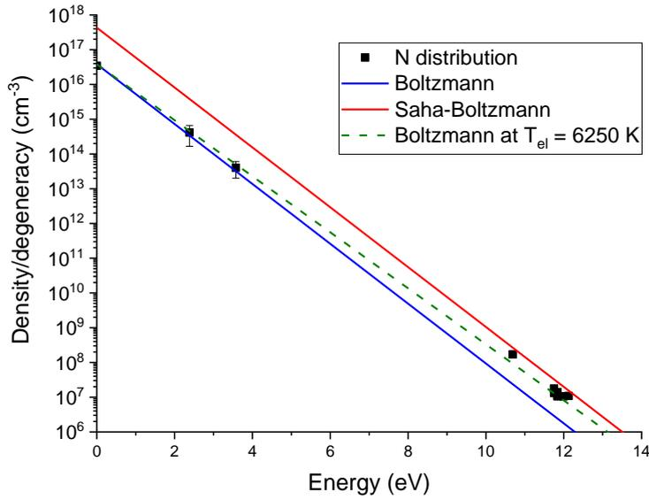
**Figure 126:** Measured population distribution of ground and excited states of atomic nitrogen (black) at the exit of the 10-cm tube for the  $N_2/Ar$  LF case at  $r = 0$  mm. The Boltzmann (blue) and Saha Boltzmann (red) distributions are also plotted. A Boltzmann distribution at  $T_{el} = 6250$  K is also plotted in green.
