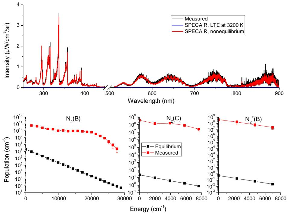
Figure 88. Top: measured and computed spectra using SPEC-AIR assuming equilibrium or nonequilibrium conditions at the exit of a 15-cm tube for the  $\text{N}_2/\text{Ar}$  HF case. Bottom: measured and equilibrium vibrational densities of  $\text{N}_2(\text{B})$ ,  $\text{N}_2(\text{C})$ , and  $\text{N}_2^+(\text{B})$  used in the SPEC-AIR calculations.
