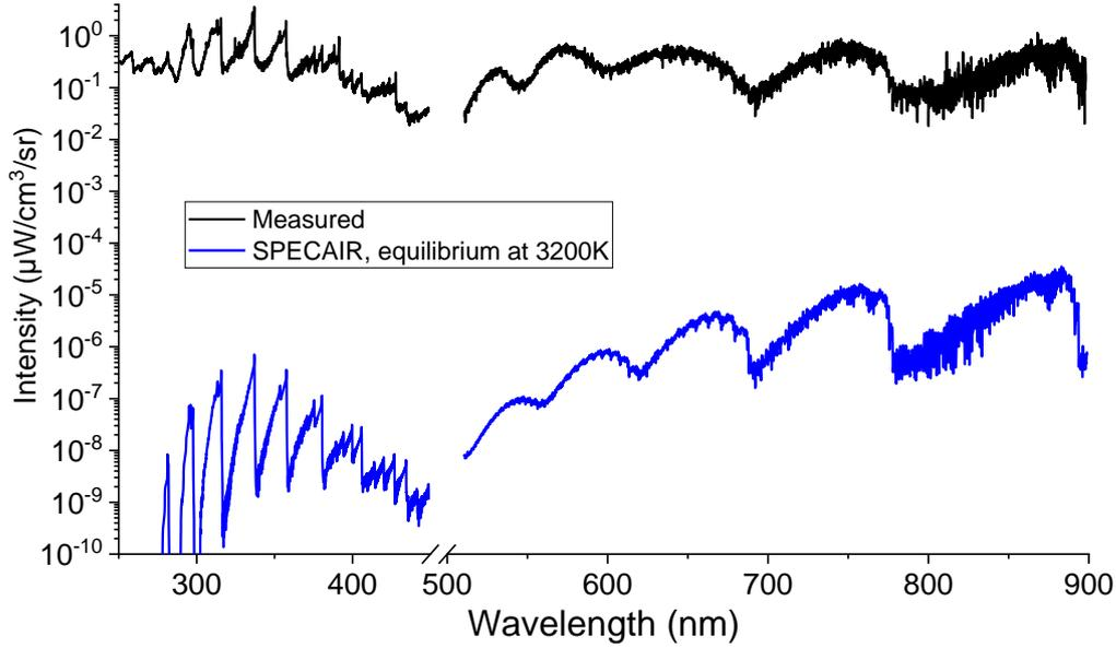
**Figure 66:** Comparison between experimental (black) and computed (blue) spectra at the exit of the 15-cm tube for the  $N_2/Ar$  HF case. The computed spectrum assumes equilibrium at the measured temperature (3200 K).
