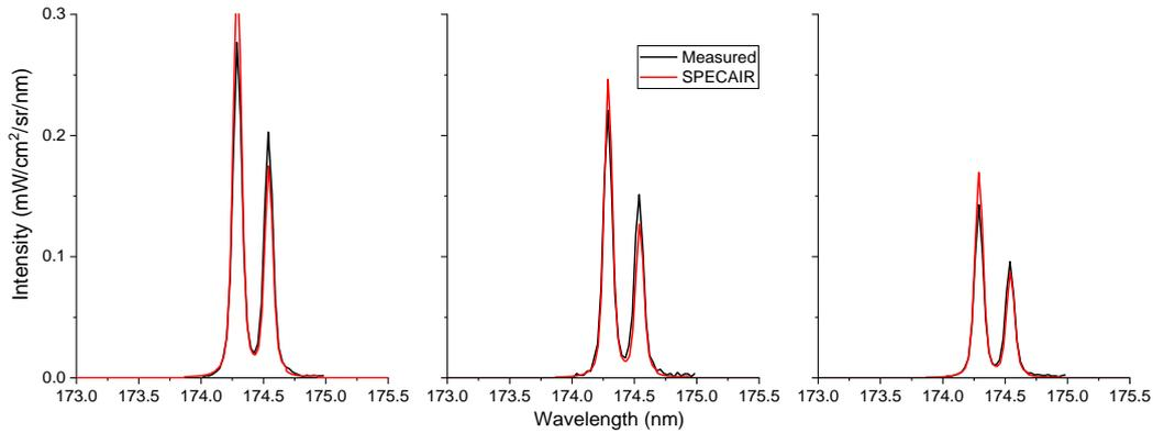
**Figure 134.** 174-nm line: comparison between the measured spectra and the optically thin computed SPECAIR spectra using the measured density profile of the upper state at the exit of the 10-cm tube for the  $N_2/Ar$  HF case. These three line-of-sight spectra were taken at different lateral positions (0, 1, and 2 mm).
