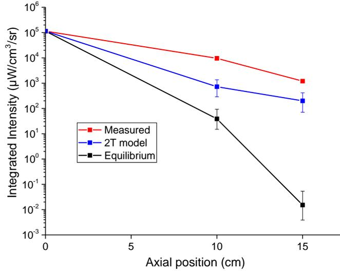
**Figure 97:** Integrated intensity between 250 and 900 nm. Red: measurements. Blue: computed intensity using the 2-temperature model. Black: computed intensity assuming equilibrium at the measured gas temperature. N<sub>2</sub>/Ar HF.
