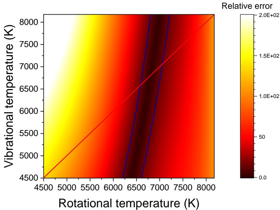
**Figure 34:** Relative error between computed area at  $(T_{\text{rot}}, T_{\text{vib}})$  and the measured area of the Stokes spectrum. The blue lines circle the values below 14%. Measurements taken in the air/argon plasma, 1 cm downstream of the exit of the 1-cm diameter nozzle.
