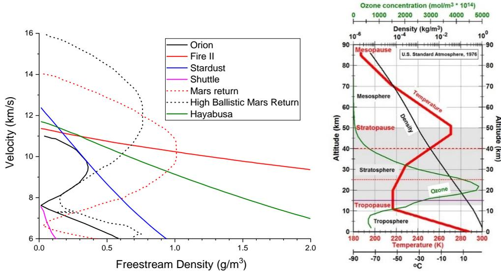
**Figure 1: Velocities during Earth atmospheric reentry for past and future missions. The velocities are presented as a function of the free stream density (left, data taken from (Brandis & Cruden, 2017)). Dashed lines represent potential future missions. The density can be linked to the altitude using the US Standard Atmosphere model (Krueger & Minzner, 1976)(right).**
