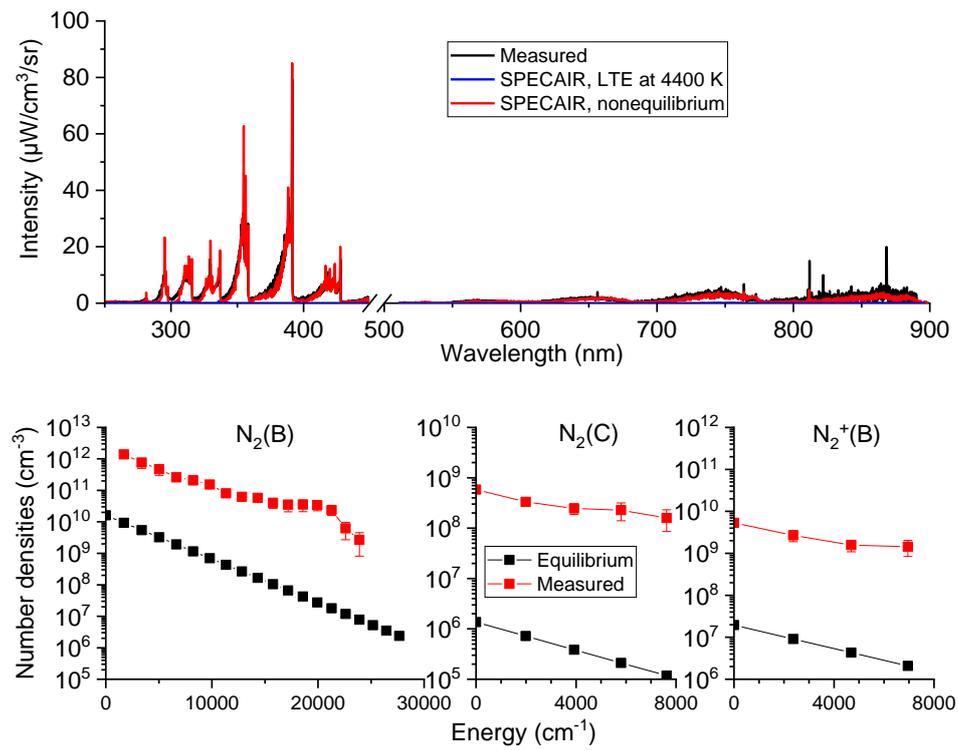
Figure 87. Top: measured and computed spectra using SPECAIR assuming equilibrium or nonequilibrium conditions at the exit of the 10-cm tube for the  $\text{N}_2/\text{Ar}$  HF case. Bottom: measured and equilibrium vibrational densities of  $\text{N}_2(\text{B})$ ,  $\text{N}_2(\text{C})$ , and  $\text{N}_2^+(\text{B})$  used in the SPECAIR calculations.
