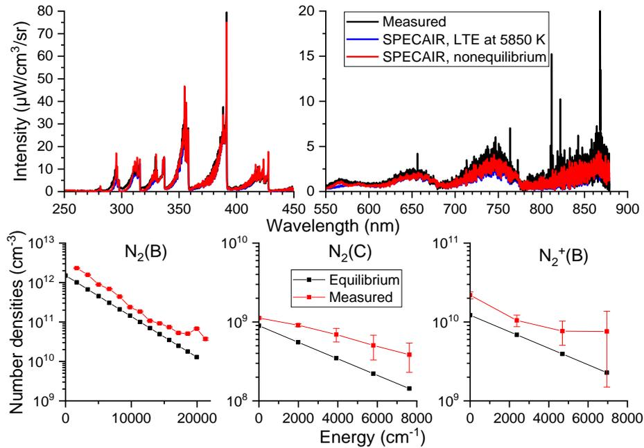
Figure 77. Top: comparison between measured and computed spectra at the exit of the 10-cm tube for the  $\text{N}_2/\text{Ar}$  LF case at the center of the tube ( $r = 0$  cm). Equilibrium spectrum (blue) and fitted spectrum (red). Bottom: equilibrium and measured populations of emitting levels used for SPECAIR calculations.
