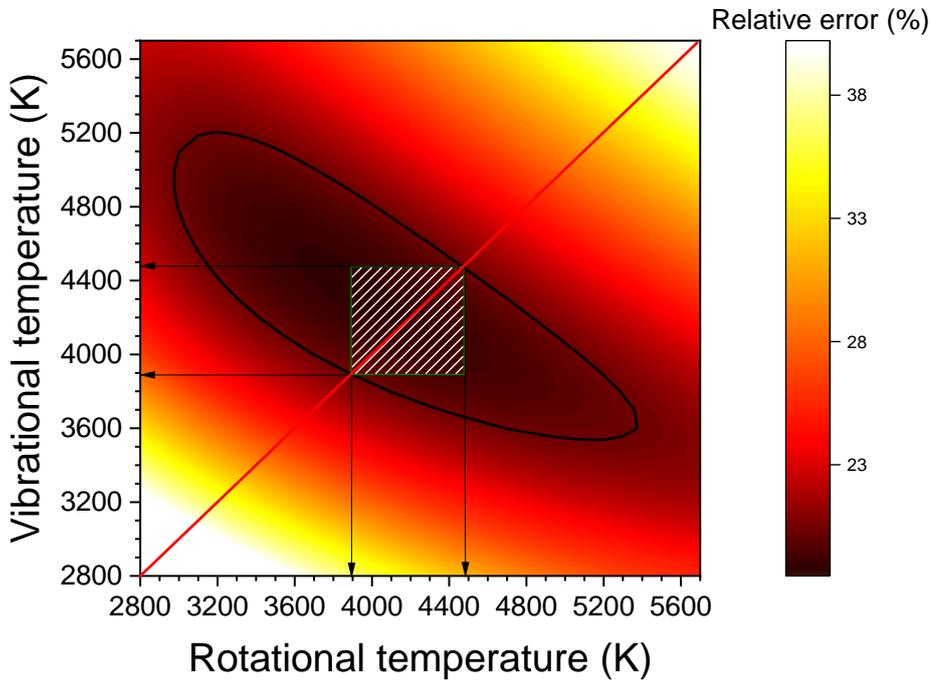
**Figure 30: Relative error between the Raman spectra computed at  $(T_{\text{rot}}, T_{\text{vib}})$  and the measured Stokes spectrum. The black lines indicate the range of temperatures where the error is below 20% (limit of acceptable fits). The white hatched region corresponds to the acceptable values for  $(T_{\text{rot}}, T_{\text{vib}})$  assuming that the plasma is close to equilibrium. Measurements taken in the air plasma, 1 cm downstream of the exit of the 30-cm tube**
