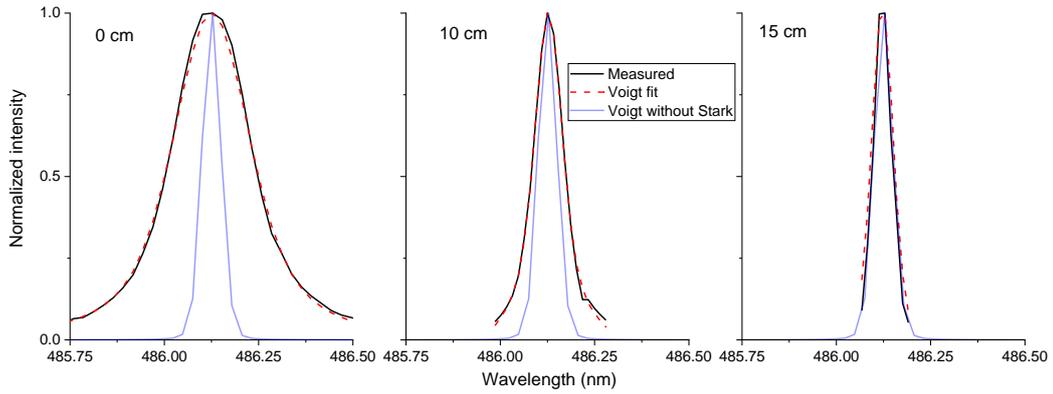
**Figure 109: Comparison between the measured H $\beta$  lineshape (black) and the fitted Voigt profiles (red dash) at 0 cm (left), 10 cm (middle) and 15 cm (right). The Voigt profiles excluding Stark broadening are plotted in blue. Air/Ar case.**
