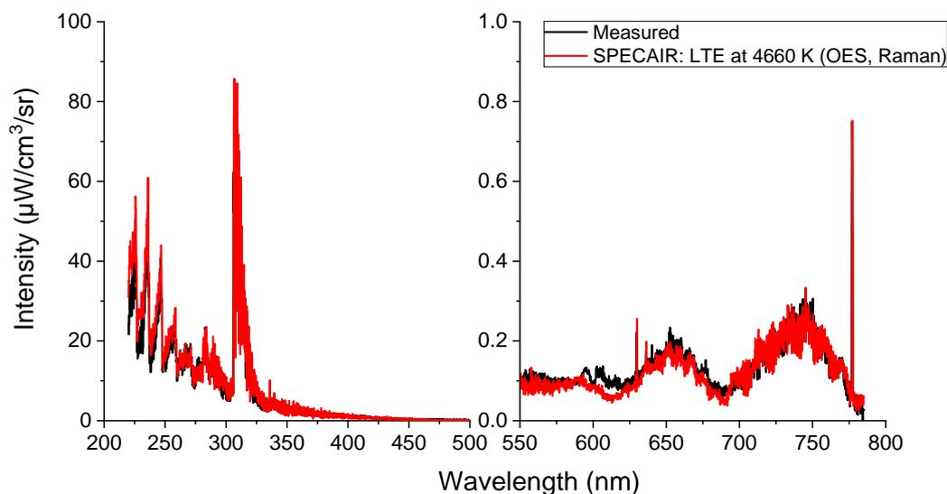
**Figure 76:** Comparison between experimental (black) and computed (red) spectrum using SPECAIR assuming equilibrium at the measured temperature (4660 K) at the center of the tube ( $r = 0$  mm) for the Air/Ar gas mixture.
