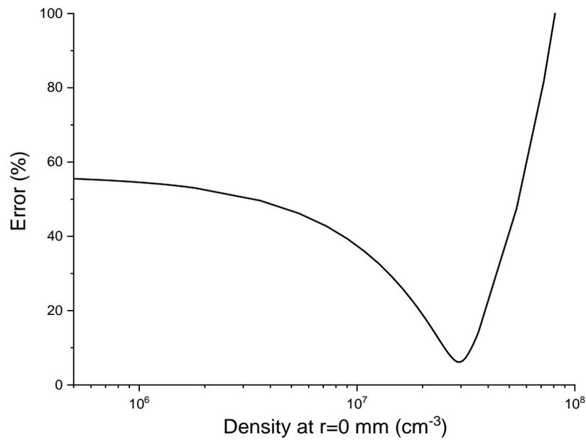
Figure 135: Relative error between measured and computed spectra of the 149-nm line at the exit of the 15-cm tube for the N<sub>2</sub>/Ar HF case as a function of the amplitude of the density of the upper state taken in the SPECAIR calculations.
