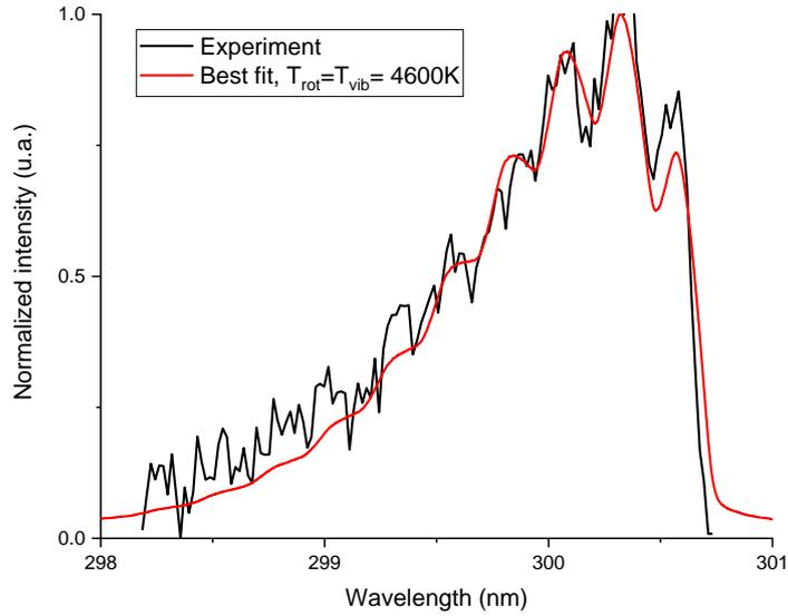
**Figure 42:** Comparison between the measured Stokes spectrum (black) and the computed Stokes spectrum assuming equilibrium at 4600 K (red). Measurements taken in the air/argon plasma, 1 cm downstream of the exit of the 15-cm tube.
