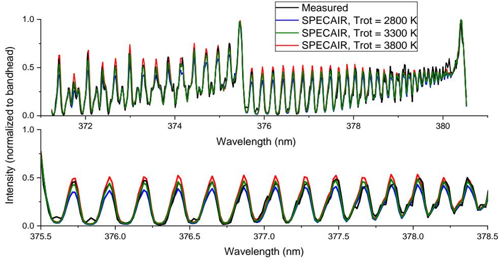
**Figure 48:** Measured and computed spectra for the rotational temperature measurement of  $N_2(C)$ . **Top:** spectrum between 371 and 381 nm used for the measurement. **Bottom:** zoom over the range 375.5 to 378.5 nm. The green spectrum (3300 K) is the best fit.
