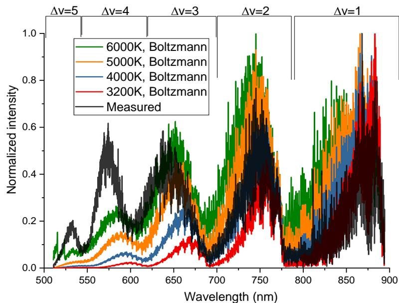
Figure 67: Comparison between experimental and computed spectra at different temperatures. The intensities are normalized. Each computed spectrum assumes a Boltzmann distribution of the vibrational levels at the indicated temperature. The rotational temperature is taken equal to the gas temperature. The vibrational bands of the  $N_2$  first positive systems are also indicated.
