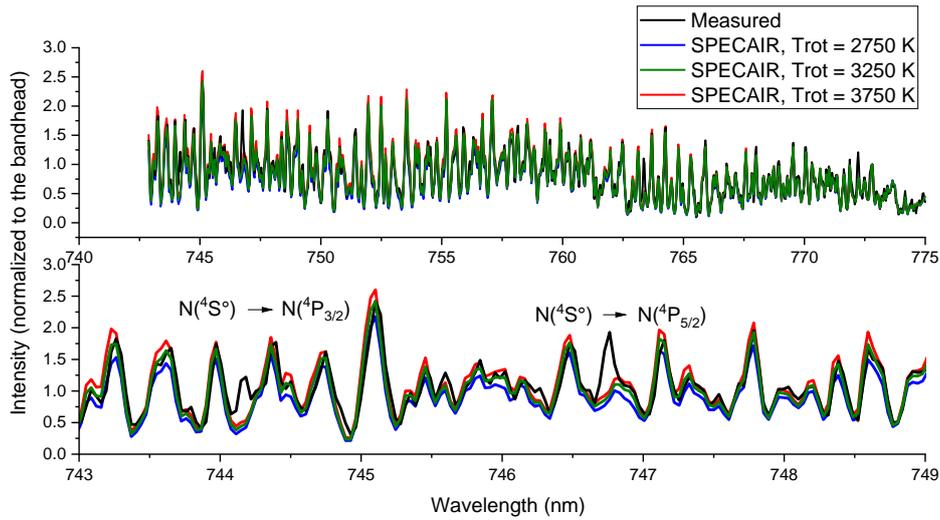
**Figure 47: Determination of the  $N_2(B)$  rotational temperature.** Measured and computed spectra for the  $N_2/Ar$  HF case at the exit of the 15-cm tube for the (2,0), (3,1) and (4,2) vibrational bands. Top: spectra between 740 and 775 nm. Bottom: zoom over the range 43 - 749 nm. The green spectrum (3250 K) is the best match. Note the presence of two atomic nitrogen lines that were not included in the SPECAIR calculations.
