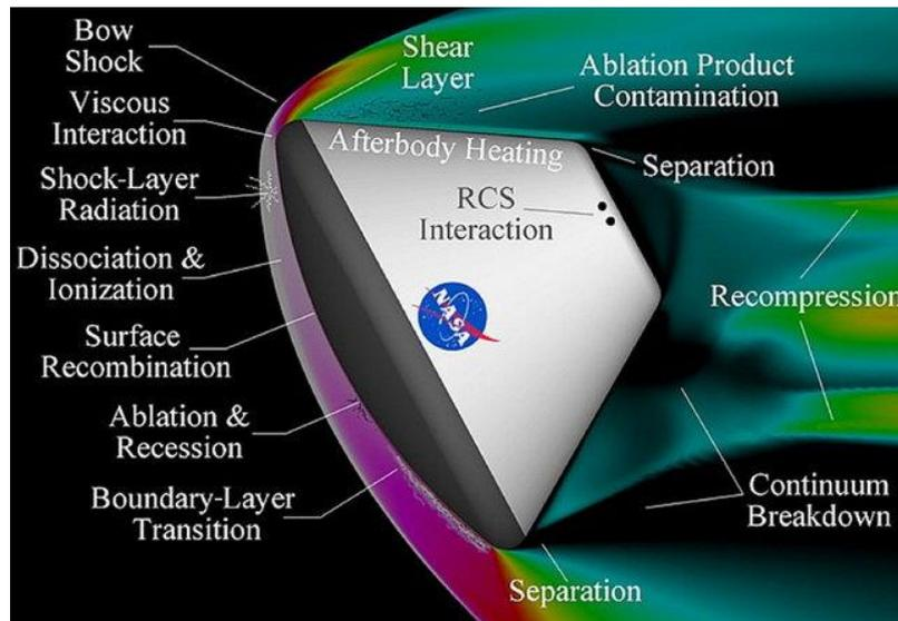
**Figure 2: Physical phenomena occurring during entry (credit NASA)**
