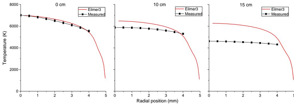
**Figure 65: Comparison of the measured radial temperature profiles with those simulated using Eilmer3. The black curve represents the measurements and the red one the simulations. The axial positions are shown at the top of each graph.**
