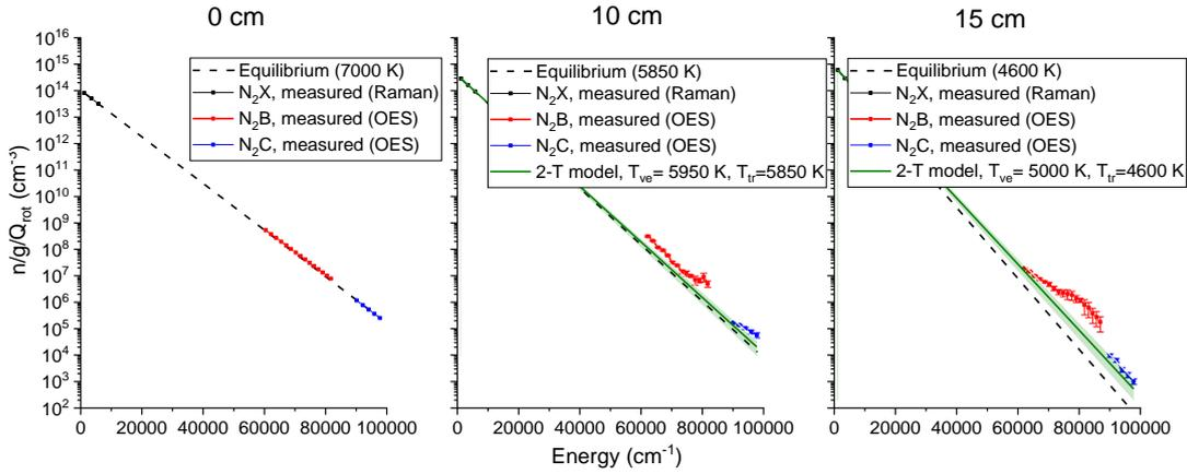
**Figure 85:** Comparison between the population distribution computed using a 2-temperature model (green) and the measurements for the  $N_2/Ar$  LF case. The green-shaded areas represent the uncertainty bands on the computed  $T_{ve}$ .
