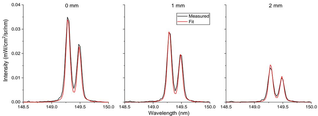
Figure 123. 149-nm line: Comparison of the measured spectra and the computed SPECAIR spectra resulting from the best fit at the exit of the 15-cm tube for the  $N_2/Ar$  LF case. These three line-of-sight spectra were taken at different lateral positions (0, 1, and 2 mm).
