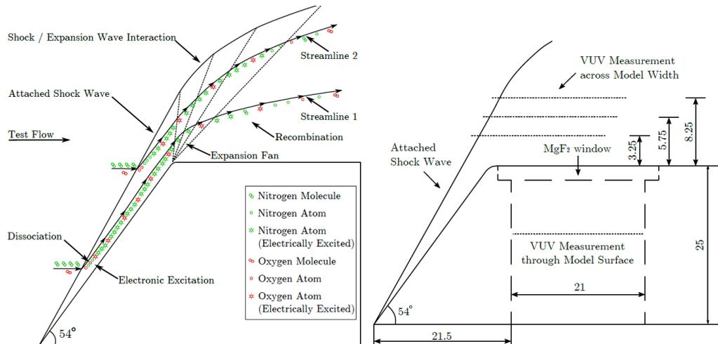
**Figure 10: Wedge configuration and measurements performed in the X2 facility. Figures taken from (Wei, 2017).**
