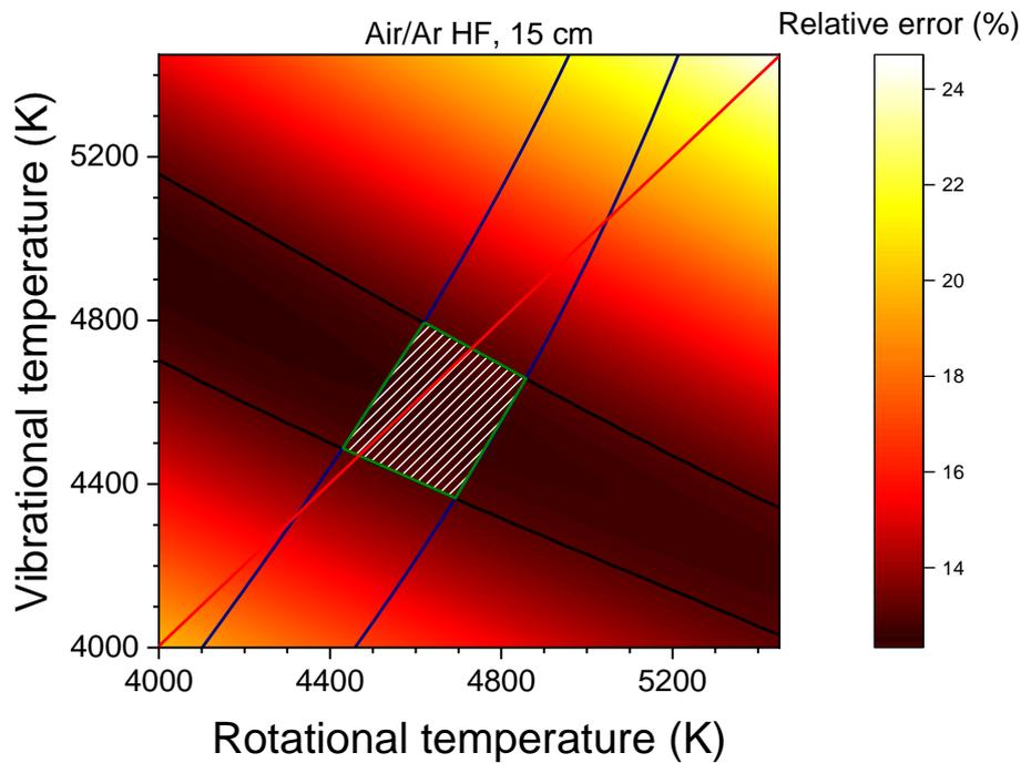
Figure 41: Relative error between computed Stokes spectra at  $(T_{rot}, T_{vib})$  and the measured Stokes spectrum. The black lines circle the values below 13%. The blue lines circle the values below 5% for the density analysis. The white hatched region corresponds to the acceptable values for  $(T_{rot}, T_{vib})$ . Measurements taken in the air/argon plasma, 1 cm downstream of the exit of the 15-cm tube.
