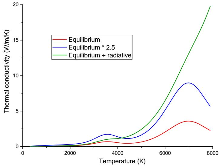
Figure 60: Thermal conductivities taken for our simulations as a function of the temperature. Red: equilibrium conductivity computed by the CEA code. Blue: same conductivity multiplied by 2.5. Green: the equilibrium conductivity plus the argon radiative conductivity multiplied by 300
