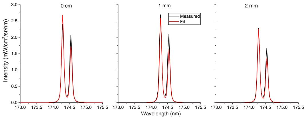
**Figure 120:** 174-nm line: comparison between the measured spectra and the computed SPECAIR spectra resulting from the best fit at the exit of the 10-cm tube for the N<sub>2</sub>/Ar LF case. These three line-of-sight spectra were taken at different lateral positions (0, 1, and 2 mm).
