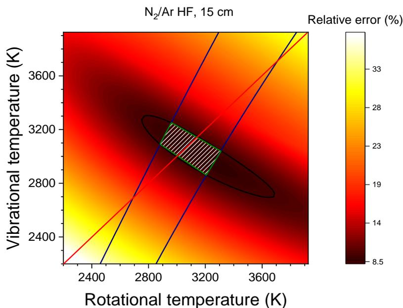
Figure 44: Relative error between computed spectra using  $(T_{\text{rot}}, T_{\text{vib}})$  and the measured Stokes signal at the exit of a 15-cm tube for the N<sub>2</sub>/Ar mixture at high flowrate. The black lines circle the values below 9%. The blue lines circle the values below 8% for the density analysis. The white dash region corresponds to the acceptable values for  $(T_{\text{rot}}, T_{\text{vib}})$ .
