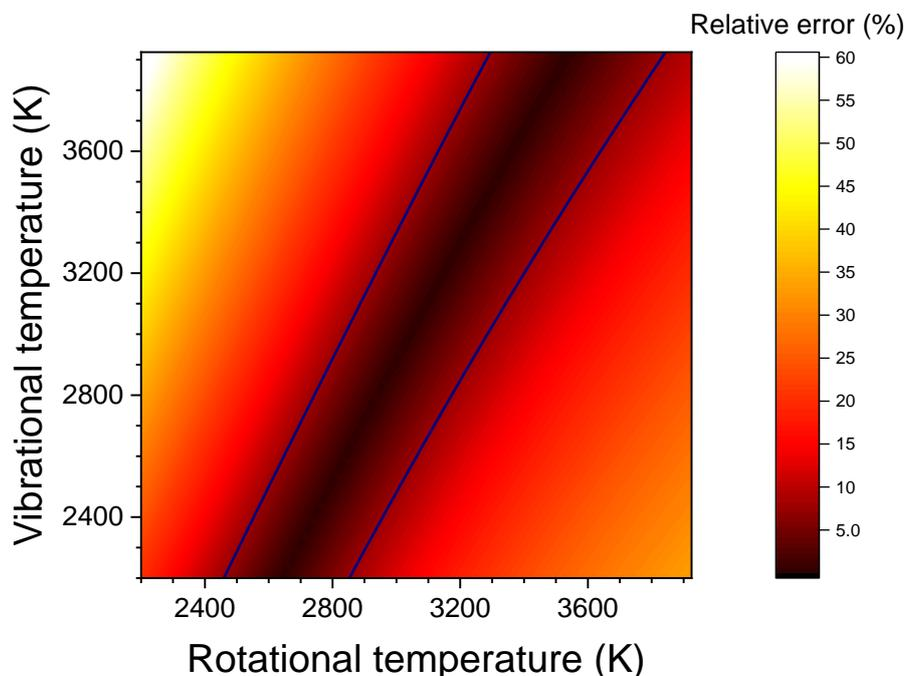
**Figure 43:** Relative error, in the density analysis, between computed area using ( $T_{rot}, T_{vib}$ ) and the measured area of the Stokes signal at the exit of a 15-cm nozzle for the  $N_2/Ar$  mixture at high flowrate. The blue lines circle the values below 8%.
