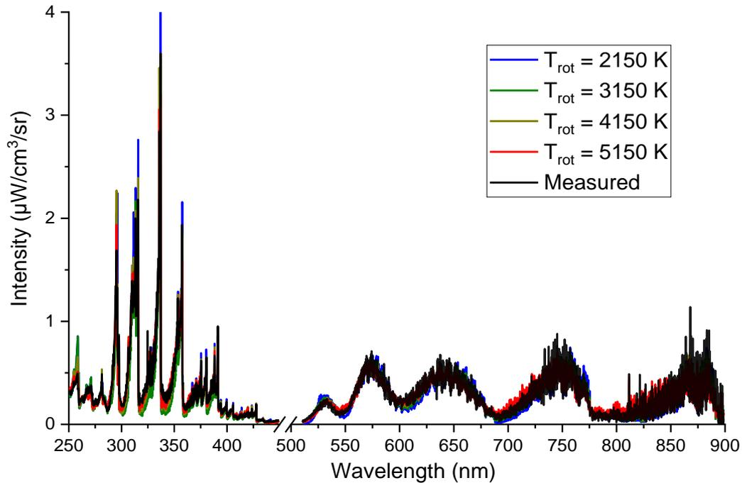
**Figure 73: Comparison between the experimental spectrum and the computed spectra resulting from the minimization algorithm for different input rotational temperatures.**
