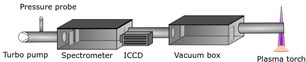
**Figure 103: Experimental setup for VUV emission spectroscopy**
