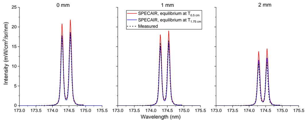
**Figure 112: Comparison between measured spectrum (black dash) and SPECAIR calculation assuming the measured temperature profile 0.5 cm downstream (red) or 1.75 cm downstream (blue) at the exit of the torch (0 cm) for the N<sub>2</sub>/Ar LF case. Three line-of-sight spectra were taken at different lateral positions (0, 1, and 2 mm).**
