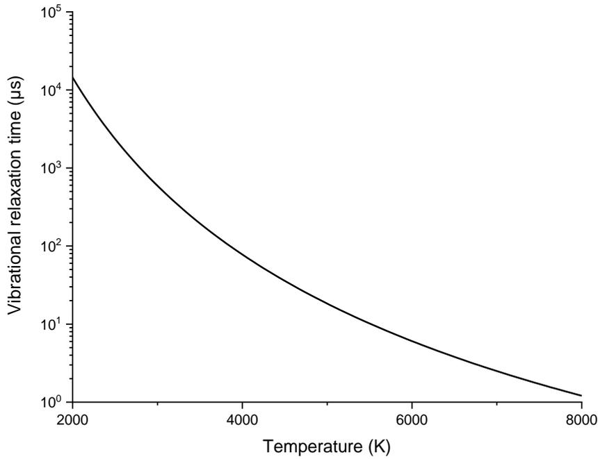
**Figure 82:** Vibrational relaxation time for the N<sub>2</sub>/Ar LF case.
