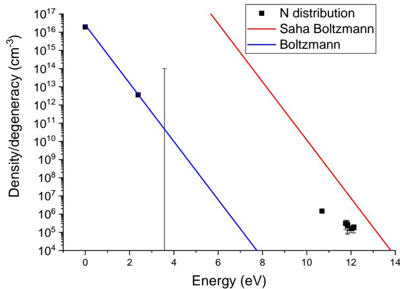
**Figure 140:** Measured population distribution of ground and excited states of atomic nitrogen (black) at the exit of the 15-cm tube for the  $\text{N}_2/\text{Ar}$  HF case at  $r = 0$  mm. The Boltzmann (blue) and Saha-Boltzmann (red) distributions are also plotted.
