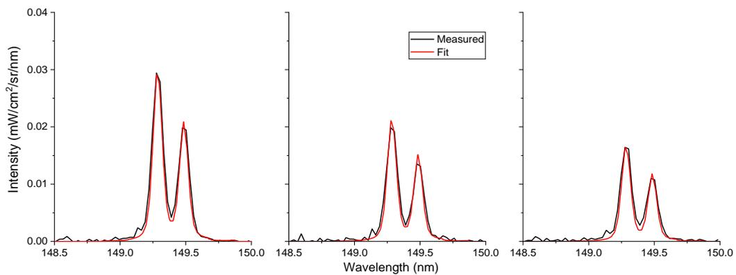
Figure 136. 149-nm line: comparison between the measured spectra and the computed SPECAIR spectra resulting from the best fit at the exit of the 15-cm tube for the N<sub>2</sub>/Ar HF case.
