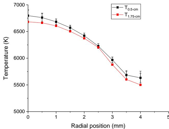
**Figure 129:** Temperature profiles at the exit of the torch (0 cm) for the N<sub>2</sub>/Ar HF case measured 0.5 cm (black) and 1.75 cm (red) downstream of the torch exit.
