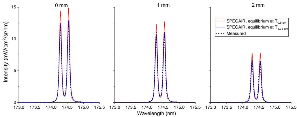
**Figure 128:** Comparison between measured spectrum (black dash) and SPECAIR calculation assuming the measured temperature profile 0.5 cm (red) or 1.75 cm downstream (blue) of the torch exit (0 cm) for the N<sub>2</sub>/Ar HF case. Three line-of-sight spectra were taken at different lateral positions (0, 1, and 2 mm).
