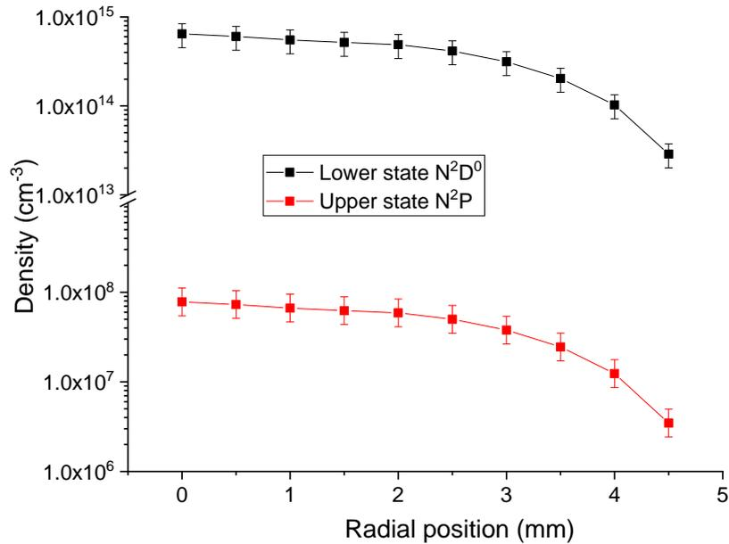
**Figure 124** Lower and upper state densities of the 149-nm transition at the exit of the 15-cm tube for the  $N_2/Ar$  LF case. Only the points out to 2 mm were measured for  $N(^2D^0)$  and the others result from the extrapolation procedure.
