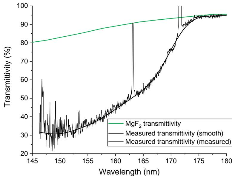
**Figure 115:** Transmittivity of a virgin MgF<sub>2</sub> window (green) and a window coated with a dark film after an experiment (black). The atomic features observed come from impurities in the argon mini arc.
