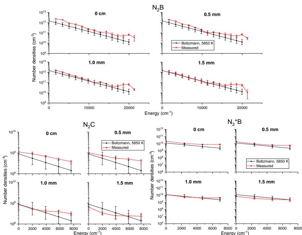
Figure 79: Radial distribution of measured and equilibrium densities of  $N_2(B)$  (top),  $N_2(C)$  (bottom left) and  $N_2^+(B)$  (bottom right) for the  $N_2/Ar$  LF case at the exit of the 10-cm tube.
