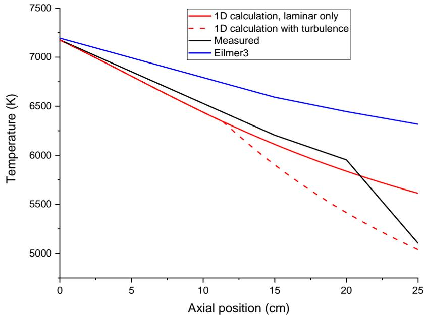
**Figure 62: Comparison between axial temperature profiles. Red line: profile computed using the 1D model using the laminar correlation only. Rad dashed line: profile computed using the 1D model using laminar and turbulent correlations for  $Re$  below and above 2300, respectively. Black: measurements. Blue: profile computed using Eilmer3.**
