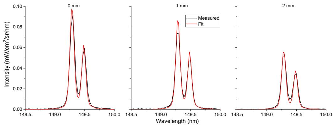
**Figure 132: Comparison of the 149-nm line between the measured spectra and the computed spectra using SPECAIR resulting from the best fit at the exit of the 10-cm tube for the N<sub>2</sub>/Ar HF case.**
