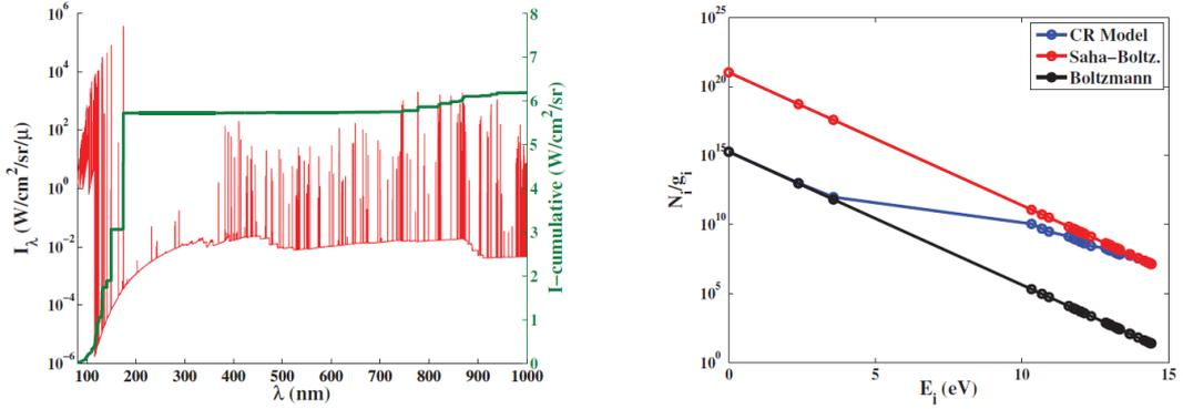
**Figure 98.** Left: Typical line-of-sight spectrum predicted in the afterbody region for Earth entry (Stardust conditions). Right: distribution of the electronic states of atomic nitrogen used to calculate the spectrum shown on the left. Figures taken from (Johnston & Brandis, 2015).
