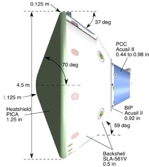
**Figure 7: Geometry and Thermal Protection System of the MSL Aeroshell**
