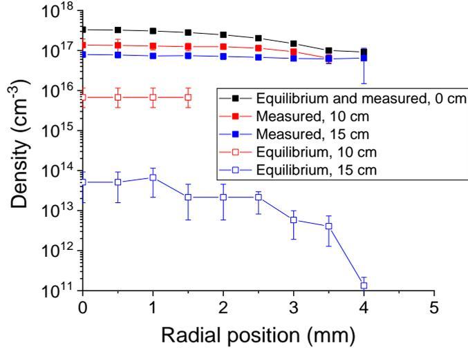
**Figure 100:** Measured radial profiles of nitrogen atom density at 0, 10, and 15 cm, and comparison with the equilibrium density profiles calculated at the temperature measured using Raman spectroscopy. N<sub>2</sub>/Ar plasma case at high flow rate.
