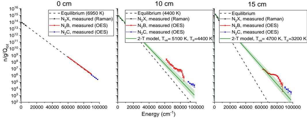
**Figure 96:** Comparison between the population distributions computed using the 2-Temperature model (green), the equilibrium model (dashed line) and the measurements for the  $N_2/Ar$  LF case. The green-shaded areas represent the uncertainty bands on the computed  $T_{ve}$ .
