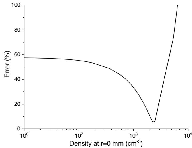
**Figure 131: Relative error between measured and computed spectra of the 149-nm line at the exit of the 10-cm tube for the N<sub>2</sub>/Ar HF case as a function of the amplitude of the density of the upper state taken in the SPECAIR calculations.**
