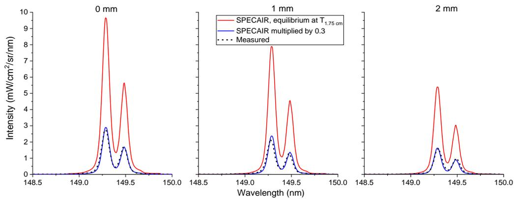
**Figure 114:** Comparison between measured spectra (black dash) and SPECAIR calculations assuming the measured temperature profile 1.75 cm downstream of the torch exit (0 cm) for the N<sub>2</sub>/Ar LF case. The blue line corresponds to SPECAIR spectra multiplied by a transmissivity of 0.3. These three line-of-sight spectra were taken at different lateral positions (0, 1, and 2 mm).
