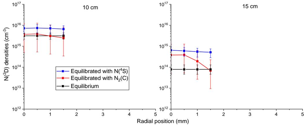
**Figure 101: Radial density profiles of  $N(^2D^0)$  at 10 cm (left) and 15 cm (right) for the  $N_2/Ar$  LF case. Red: measured. Blue: assuming partial equilibrium with  $N(^4S^0)$  at the gas temperature. Black: assuming LTE at the gas temperature.**
