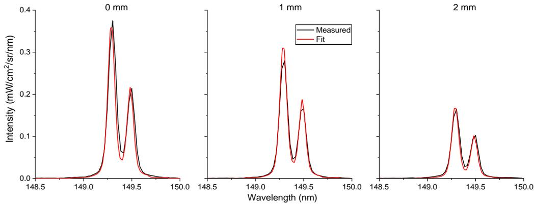
**Figure 117: 149-nm line: comparison between the measured spectra and the computed SPECAIR spectra resulting from the best fit at the exit of the 10-cm tube for the  $N_2/Ar$  LF case. These three line-of-sight spectra were taken at different lateral positions (0, 1, and 2 mm).**
