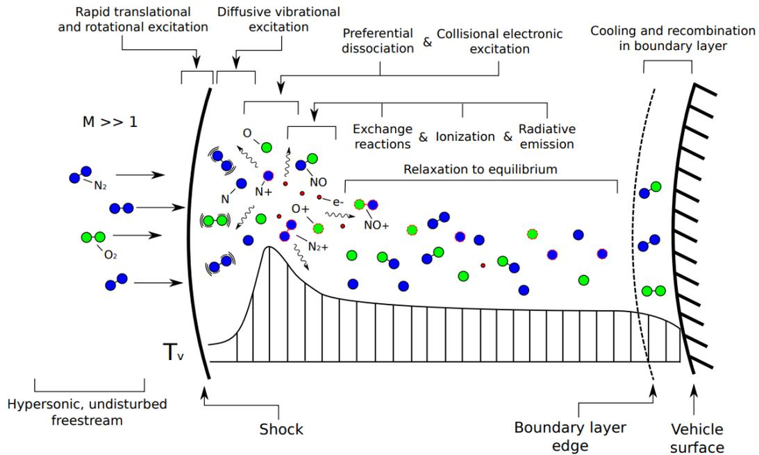
**Figure 6: Schematic of kinetics occurring along the stagnation streamline for Earth reentry. The nonequilibrium region is observed near the shock and the gas relaxes to equilibrium in the shock layer (figure taken from (Potter, 2011))**
