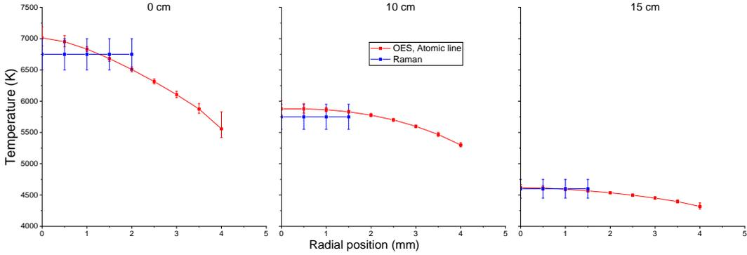
Figure 50: Temperature profiles measured using OES and Raman spectroscopy for the Air/Ar plasma case.
