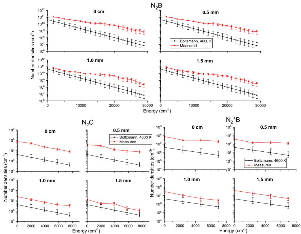
**Figure 80:** Radial distribution of measured and equilibrium densities of  $N_2(B)$  (top),  $N_2(C)$  (bottom left), and  $N_2^+(B)$  (bottom right) for the  $N_2/Ar$  LF case at the exit of the 15-cm tube.
