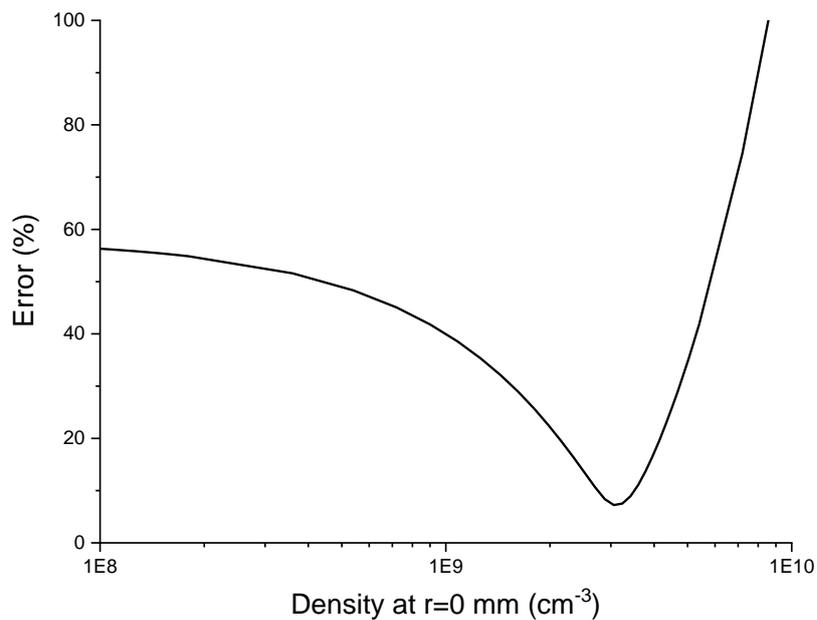
**Figure 116:** Relative error between measured and computed spectra of the 149-nm line at the exit of the 10-cm tube for the  $N_2/Ar$  LF case as a function of the amplitude of the density of the upper state taken in SPECAIR calculations.
