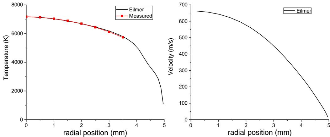
**Figure 56: Left - Inlet temperature profiles used for the CFD calculations (black line) and corresponding measurements (red). Right – predicted velocity profile at the inlet of the tube**
