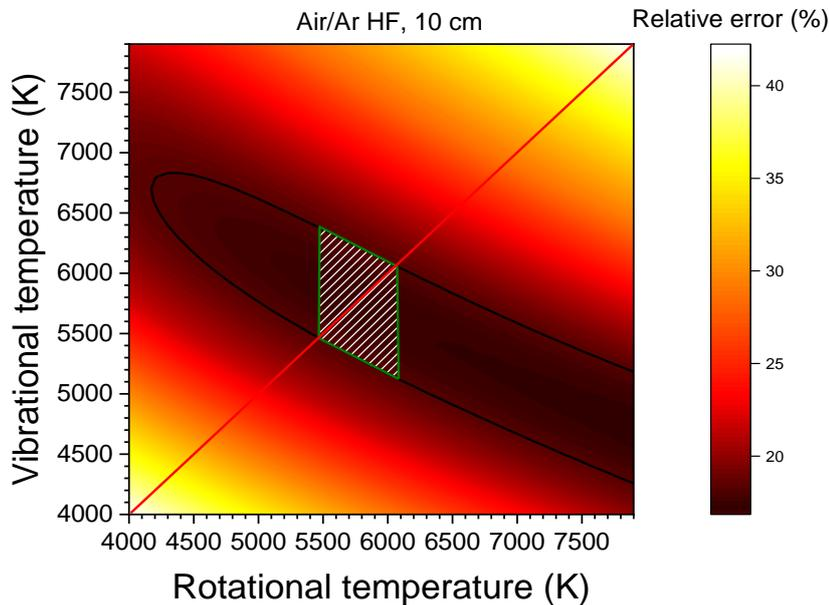
**Figure 40:** Relative error between computed Stokes spectra at  $(T_{\text{rot}}, T_{\text{vib}})$  and the measured Stokes spectrum. The black lines circle the values below 18%. The white hatched region corresponds to the acceptable values for  $(T_{\text{rot}}, T_{\text{vib}})$ . Measurements taken in the air/argon plasma, 1 cm downstream of the exit of the 10-cm tube.
