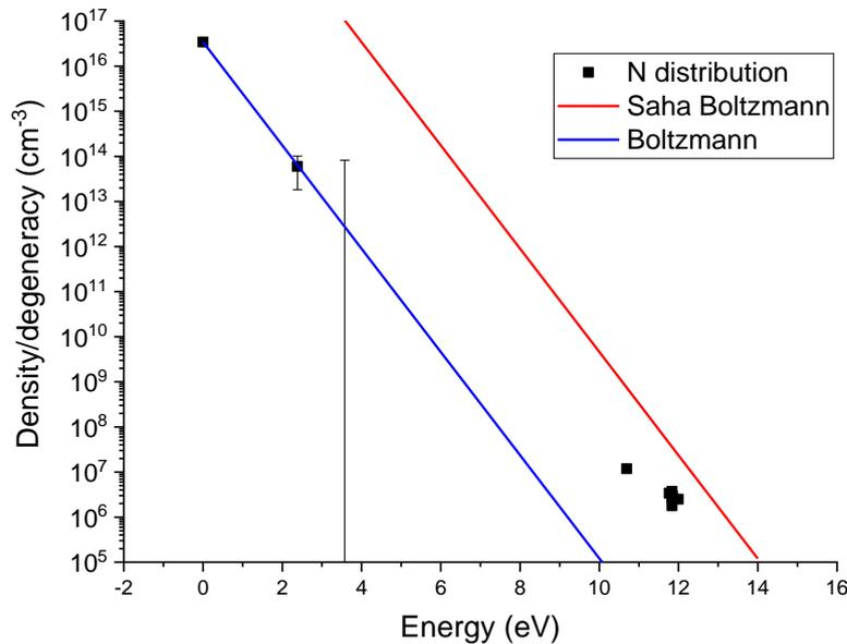
Figure 139: Measured population distribution of ground and excited states of atomic nitrogen (black) at the exit of the 10-cm tube for the  $N_2/Ar$  HF case at  $r = 0$  mm. The Boltzmann (blue) and Saha-Boltzmann (red) distributions are also plotted.
