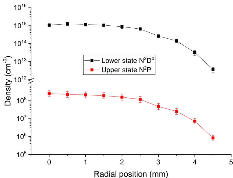
**Figure 133:** densities of the lower and upper states of the 149-nm transition at the exit of the 10-cm tube for the  $N_2/Ar$  HF case. Only the points out to 2 mm were measured for  $N(^2D^0)$  and the others were extrapolated.
