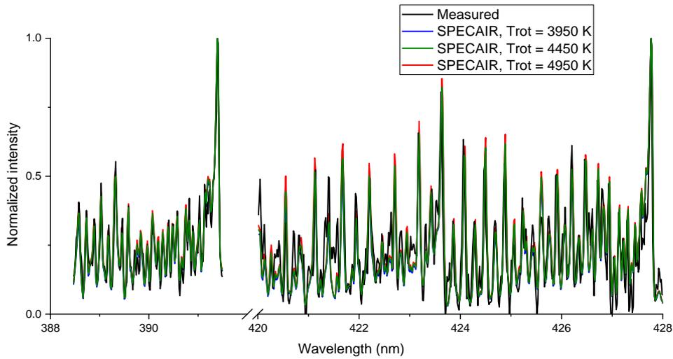
**Figure 49:** Measured and computed spectra for the determination of the rotational temperature of  $N_2^+(B)$ . The green curve ( $T=4450K$ ) is the best fit.
