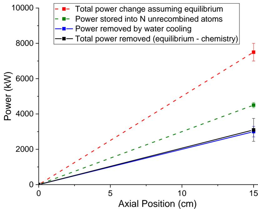
Figure 146: Power balance measurements for the  $N_2/Ar$  plasma (low mass flowrate), using two different approaches. Blue: measured power removed by water cooling. Red: Power change between the outlet and the inlet of the tube assuming equilibrium throughout the tube. Green: power stored into unrecombined N atoms using the measured overpopulation factors. Black (red minus green curve): total power removed from the gas.
