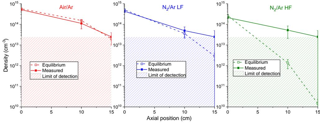
**Figure 111: Electron density measurements using Stark broadening of the  $H_\beta$  line for the Air/Ar (left),  $N_2$ /Ar LF (middle) and  $N_2$ /Ar HF (right) cases at 0, 10 and 15 cm. The lower limit of detection is  $2.5 \times 10^{13} \text{ cm}^{-3}$ .**
