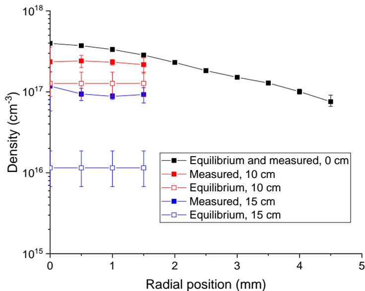
**Figure 99:** Measured radial profiles of nitrogen atom density at 0, 10, and 15 cm, and comparison with the equilibrium density profiles calculated at the temperature measured using Raman spectroscopy. N<sub>2</sub>/Ar plasma at low mass flowrate.
