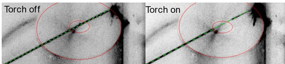
**Figure 39: Images taken to check potential beam steering effects. The inner and outer contours of the nozzle are drawn in red. The laser beam corresponding to Rayleigh scattering is highlighted in green. Left: torch off. Right: torch on (the light scattered by the laser beam is lower when it crosses the hot plasma). No significant deviation ( $< 1$  mm) of the beam is observed.**
