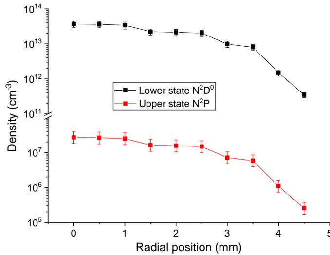
**Figure 137:** Lower and upper state densities of the 149-nm transition at the exit of the 15-cm tube for the  $N_2/\text{Ar}$  HF case. Only the points out to 2 mm were measured for  $N(^2D^0)$  and the others result from the extrapolation procedure.
