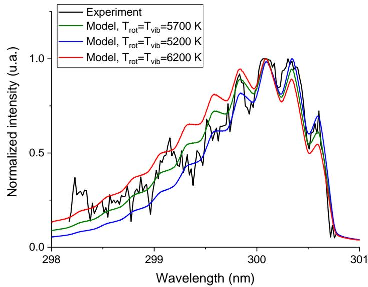
Figure 28: Comparison between the measured Stokes spectrum (black), the best fit corresponding to  $T_{rot} = T_{vib} = 5700\text{K}$  (green), and the lower and upper uncertainty limits:  $T_{rot} = T_{vib} = 5700 - 500 = 5200\text{K}$  (blue) and  $T_{rot} = T_{vib} = 5700 + 500 = 6200\text{K}$  (red).
