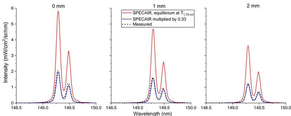
**Figure 130: Comparison between measured spectrum (black dash) and SPECAIR calculation assuming the measured temperature profile 1.75 cm downstream of the torch exit (0 cm) for the N<sub>2</sub>/Ar HF case. The blue line corresponds to the same calculation multiplied by a transmissivity of 0.33. Three line-of-sight spectra were taken at different lateral positions (0, 1, and 2 mm).**
