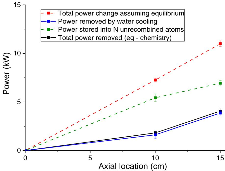
**Figure 147: Power balance measurements for the N<sub>2</sub>/Ar plasma (high mass flowrate), using two different approaches. Blue: measured power removed by water cooling. Red: Power change between the outlet and the inlet of the tube assuming equilibrium throughout the tube. Green: power stored into unrecombined N atoms using the measured overpopulation factors. Black (red minus green curve): total power removed from the gas.**
