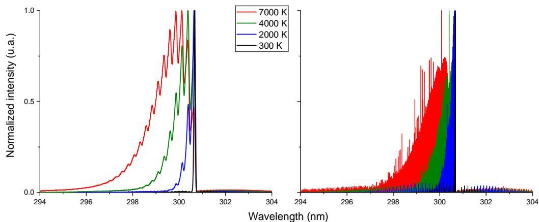
**Figure 21: Modeled Raman spectra of  $N_2$  (normalized in intensity) for  $T_{vib} = T_{rot} = 300, 2000, 4000,$  and  $7000$  K. Left: Modeled spectra convolved with a triangular instrumental function of  $FWHM = 0.065$  nm. Right: No slit function. Laser excitation wavelength:  $281$  nm.**
