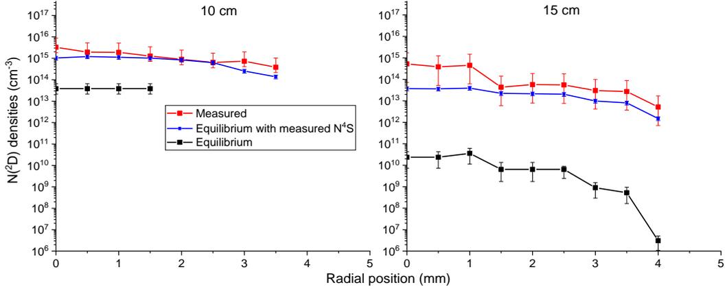
Figure 102: Radial density profiles of  $N(2D^0)$  at 10 cm (left) and 15 cm (right) for the  $N_2/Ar$  HF case. Red: measured. Blue: assuming partial equilibrium with  $N(4S^0)$  at the gas temperature. Black: assuming LTE at the gas temperature.
