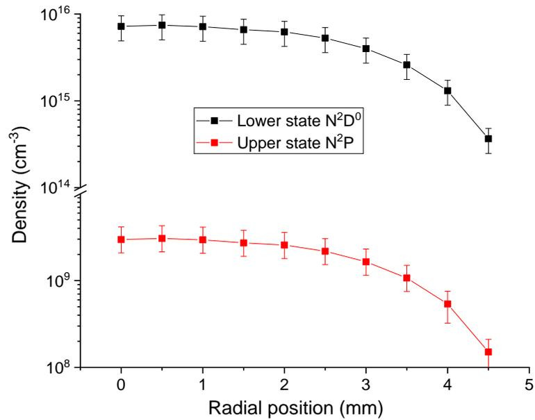
**Figure 118:** Lower and upper state densities of the 149-nm transition at the exit of the 10-cm tube for the  $N_2/Ar$  LF case. Only the points out to 2 mm were measured for  $N(^2D^0)$  and the others result from the extrapolation procedure.
