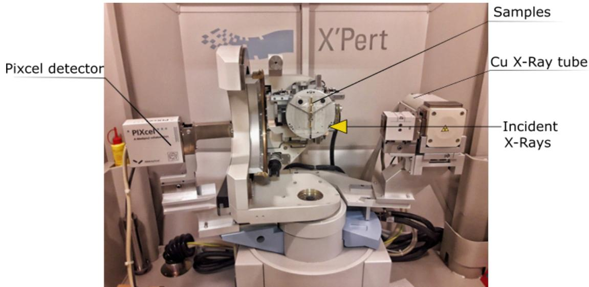
Figure 4.36: Interior of X-Ray diffractometer from PANalytical.
