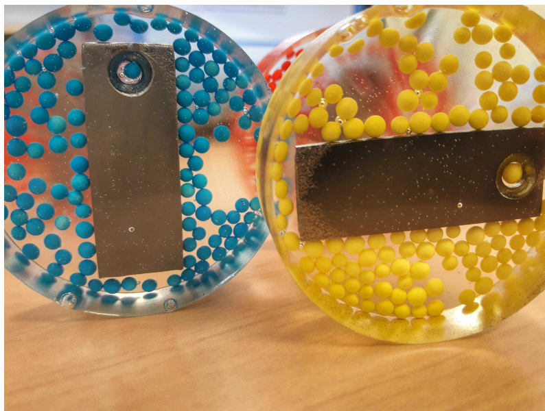
Figure A3.2: Mounted samples in the epoxy with the different ceramic balls (yellow, blue and red).
