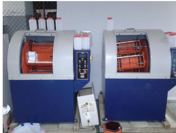
Figure 4.9: Photograph of CBP machine with 4 barrels (ABC SwissTech production).
