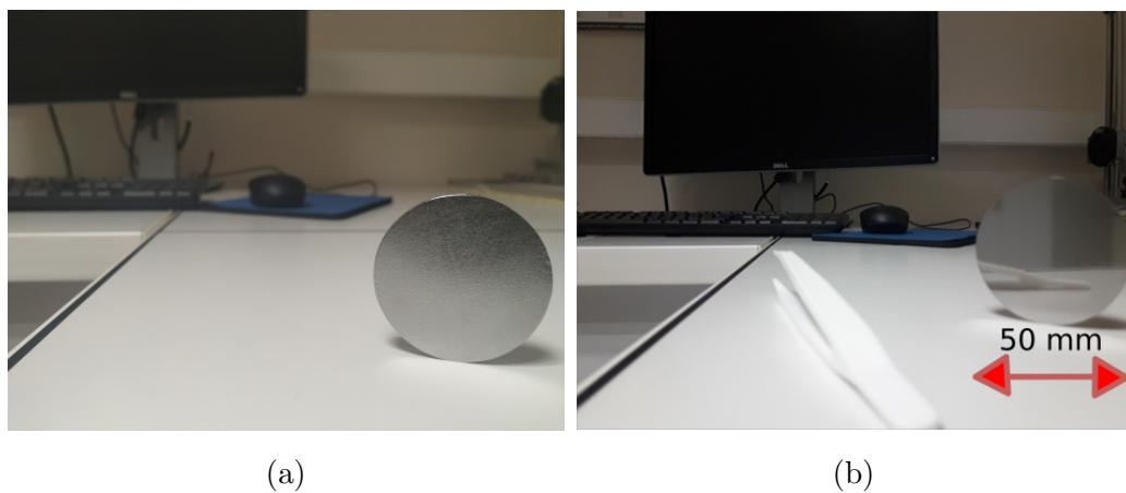
Figure 5.40: Photographies of Nb disk after BCP (a) and after 2 step MP for RF test at SLAC.
