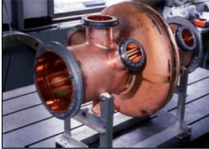
Figure 2.3: The LHC single cell elliptical cavity [27].
