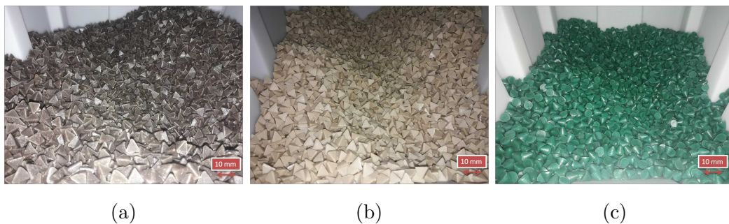
Figure 4.12: Photographs of plastic media from ABC SwissTech production: a) pyramids TET-TKS, b) pyramids TET-TKP and c) cones TKV.
