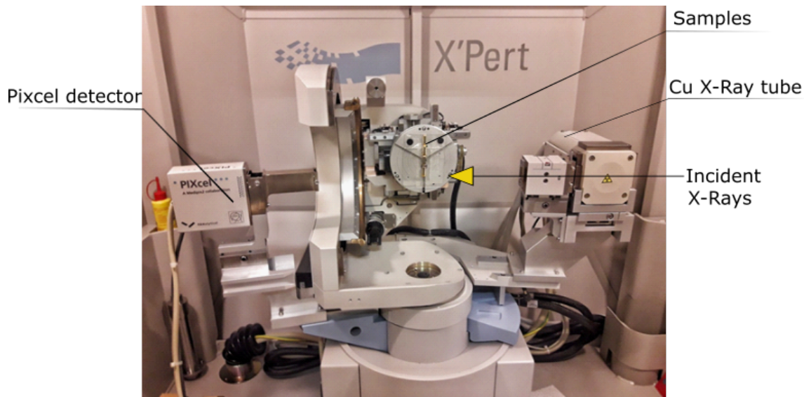
Figure 4.36: Interior of X-Ray diffractometer from PANalytical.
