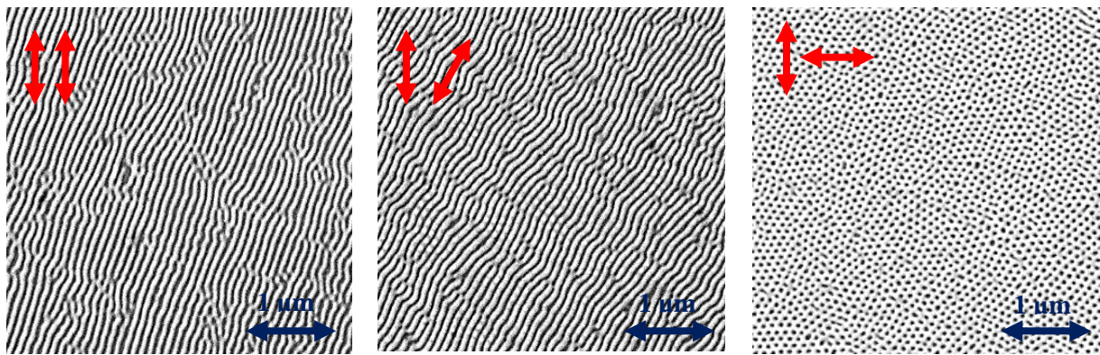
Fig 8.4 SEM images of three different zones irradiated with N_{\text{DPS}} = 25 at 0.24 \text{ J/cm}^2 with a time-delay of 24ps. The polarization between the pulses of a sequence is varied. Nanoholes are formed only for crossed polarization.
