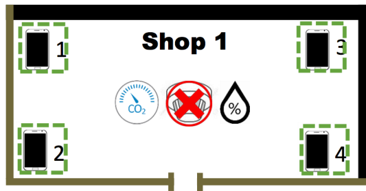
FIGURE 4.5: Assigning all mobile sensors to smoke observation
