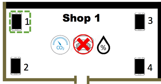
FIGURE 4.4: Mobile Sensor 1 replaces the smoke sensor
