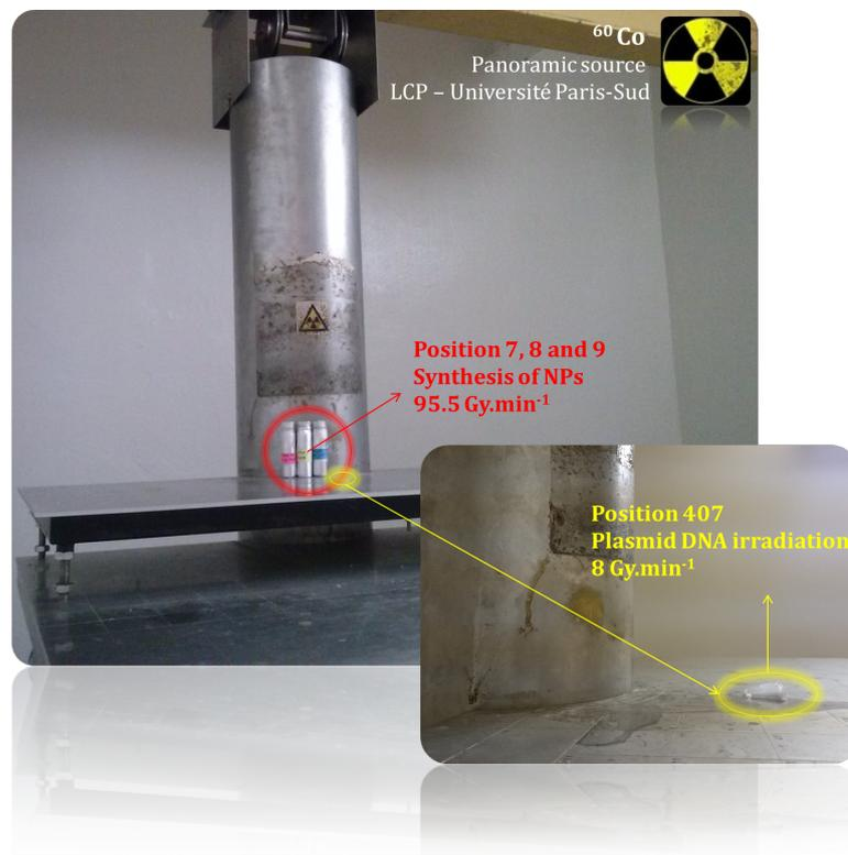
**Figure II - 4.** The cobalt-60 panoramic source used for NPs synthesis and plasmid DNA irradiation.
