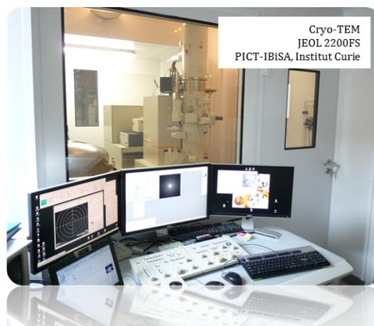
**Figure II - 15.** The JEOL 2200FS used at the PICT-IBiSA platform for cells imagery.
