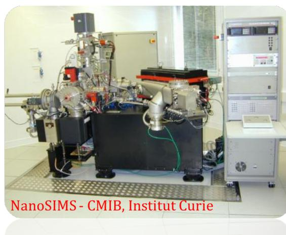
**Figure II - 13.** The Cameca NanoSIMS 50 ion-probe for element analysis at the CMIB platform (Institut Curie).
