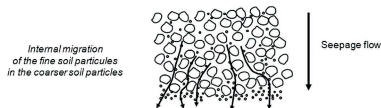
FIGURE I.6 – Principle of suffusion (Sharp et al., 2013)
